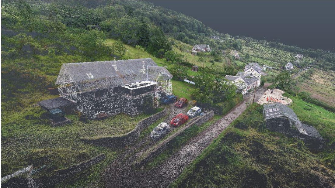
Figure A-7: A dense point cloud of a countryside house produced using commercial reconstruction software, Pix4D [127].
