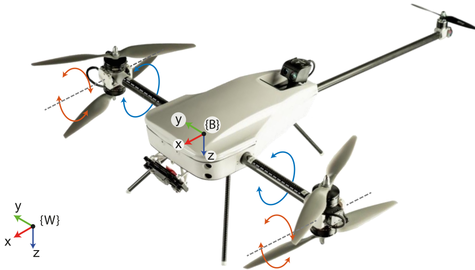
Figure 3-2: The Voliro tricopter aerial manipulation platform. Annotations show the body and inertial world coordinate frames and axes of actuation granting 6 DoF wrench exertion. Both propeller arms rotate independently. Bi-propeller assemblies rotate in one further axis about the tip of these arms, as indicated by blue and orange arrows.
