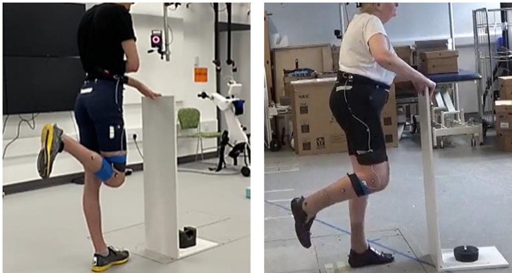
Figure 4-10. Full range of motion flexion/extension stability platform, used to maintain balance during the Flexion/Extension activity.
