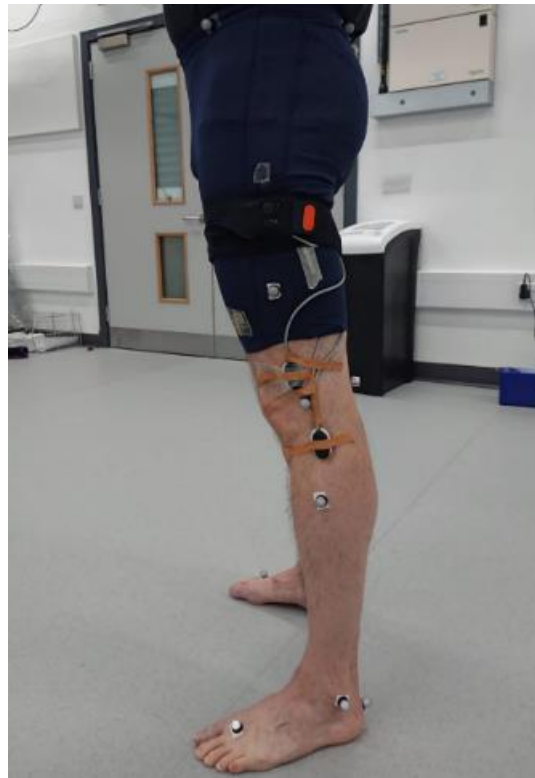
Figure 4-5 Participant with lower body Plug-in-Gait marker model and wired IMU device.
