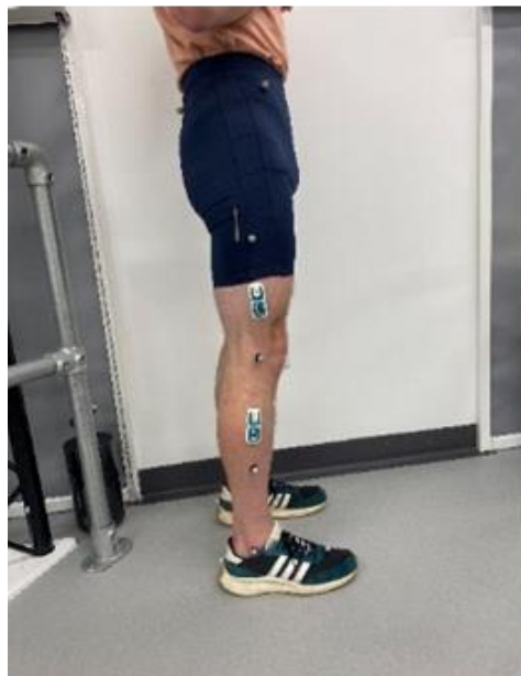
Figure 4-4. Participant with lower body Plug-in-Gait marker model, and left and right sagittal view of participant with MotionSense™ sensors attached to their thigh and shank.
