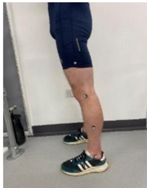
Figure 4-4. Participant with lower body Plug-in-Gait marker model, and left and right sagittal view of participant with MotionSense™ sensors attached to their thigh and shank.
