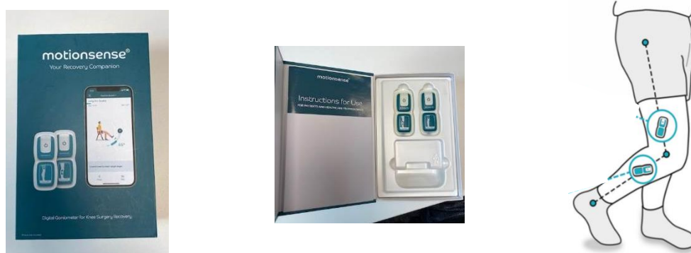
Figure 1. MotionSense box (left), IMU wearables in box (middle) and attached to leg (right).
