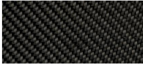
Figure 3.10 The 12k G34-700 carbon fibre cloth with 2×2 Twill pattern.
