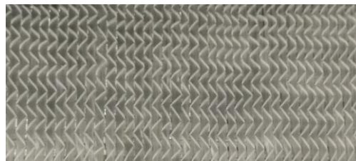
Figure 3.9 Biaxial U-E 592 g/m 2 from Cristex Composite Material Ltd
