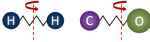
FIGURE 1.8. The rotation of \text{H}_2 and \text{CO} molecules about their centre of mass. For \text{H}_2 , the centre of charge coincides with the centre of mass and it has no dipole moment.
