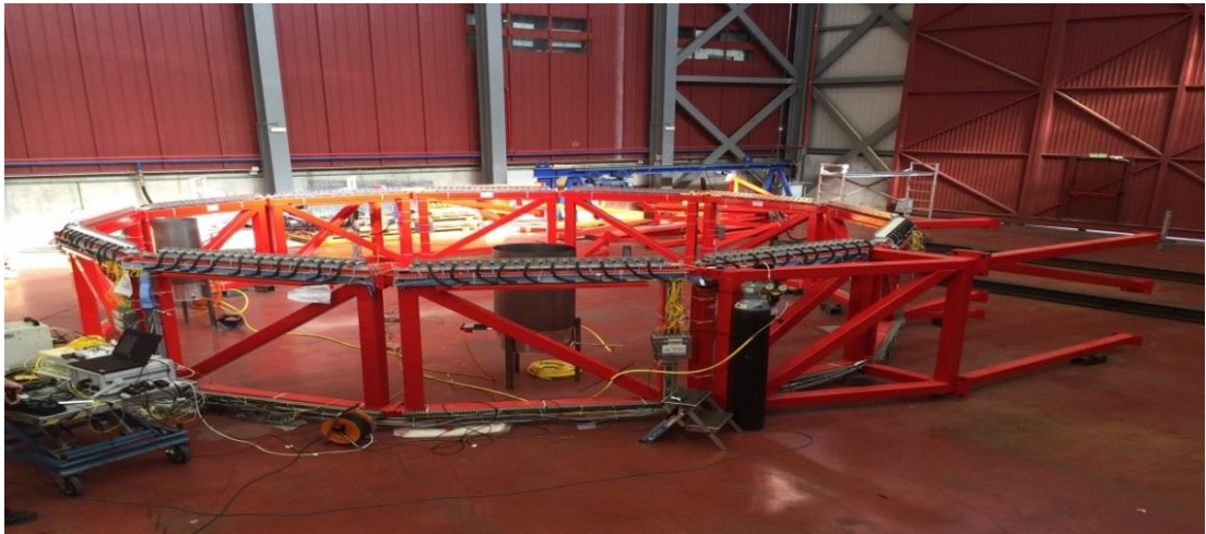
Figure 7-1. Paella burners at the centre of the dodecagon mounting ring placed horizontally, for the phantom tests at INTA (Courtesy of the FLITES consortium).
