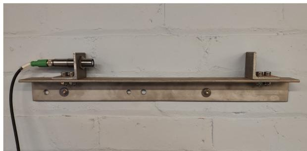
Figure 3.5: Ultrasonic wave probe calibration
