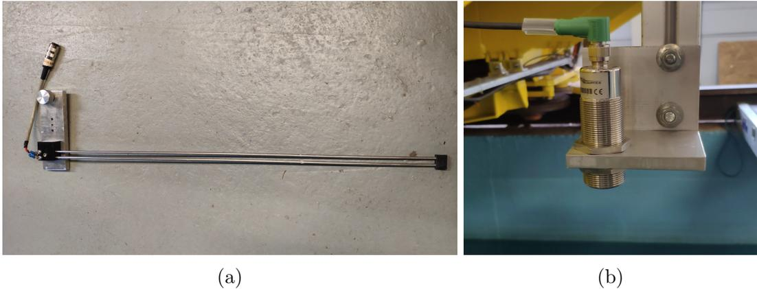
Figure 3.1: Left: The resistance wave probe. Right: The ultrasonic wave probe.
