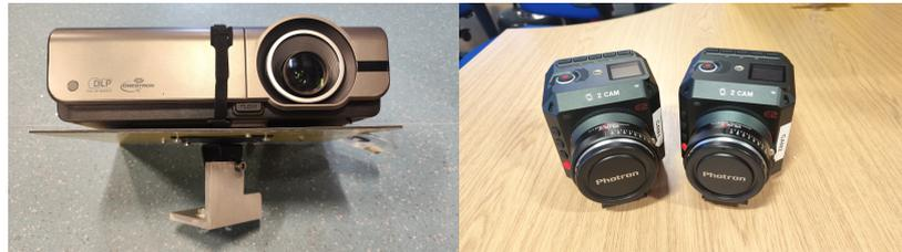
Figure 5.3: Projector (left) and cameras (right) used for the stereo vision system.
