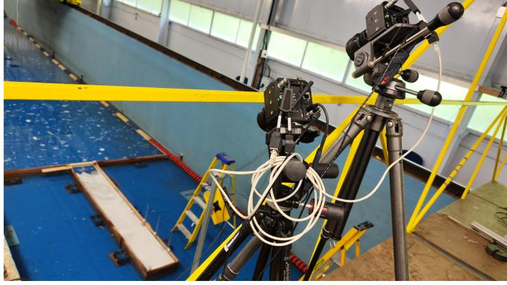
Figure 6.4: Experiment setup for measuring the water surface inside the lock area
