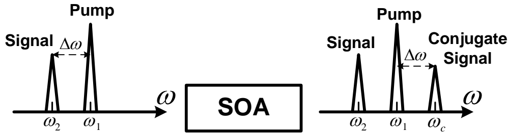
Figure 4.6 Schematic of the degenerate four wave mixing process in the SOA (output satellite signal at a frequency of 2\omega_2 - \omega_1 and ASE spectrum are omitted).
