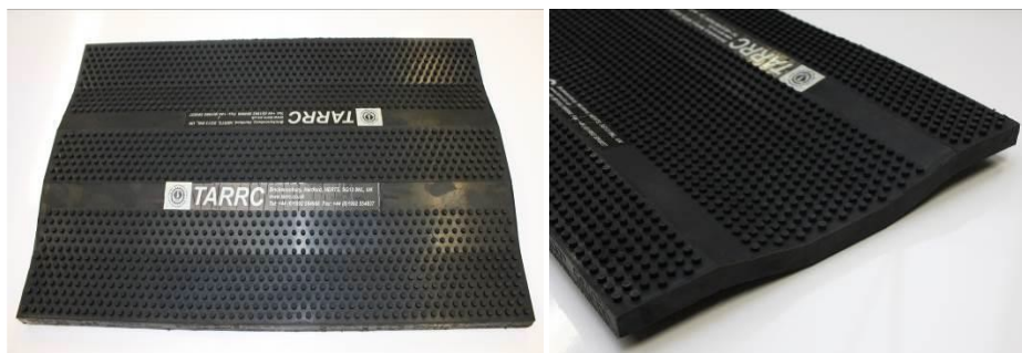
Figure 2.20. Horizontal rubber joints developed by TARRC (Ahmadi et al. 2017).
