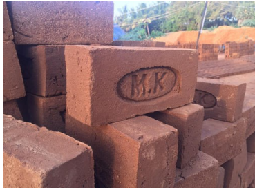
a) Solid fired clay bricks
