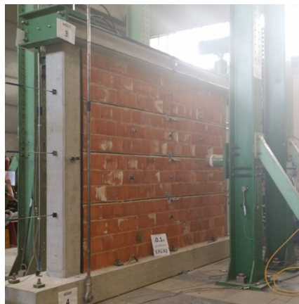
Figure 3.1. Masonry infilled frame with horizontal and vertical rubber joints tested within INSYSME project (INSYSME 2016).
