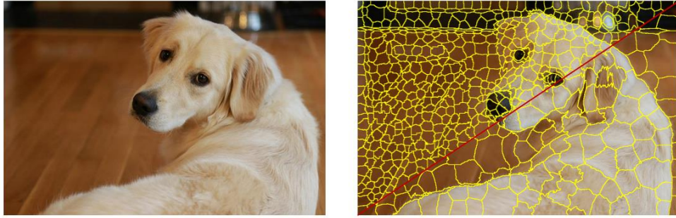
Figure 3. 1: (left) Sample image. (right) Superpixel segmentation results with 200 (lower right) and 1000 (upper left) superpixels and the boundaries of each superpixel marked in yellow.
