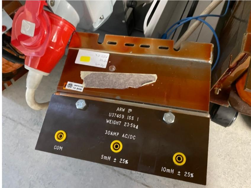
Figure 5.3. Inductor used as  $L_{ac}$  in experimental circuit.
