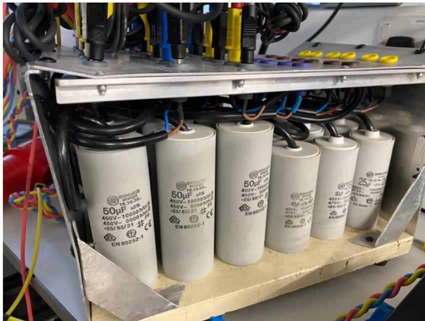
Figure 5.4. Capacitor bank used as  $C_{comp}$  in experimental circuit.
