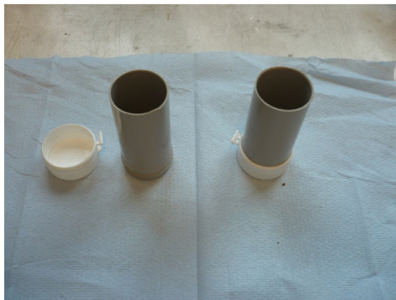
Figure 3.7: On the left a grey plastic cylinder of length 7 cm and internal volume of 198 cm 3 next to a white cap with a plastic release mechanism on rear with an internal diameter of 3 cm. The construction of the pour mould is shown on the right
