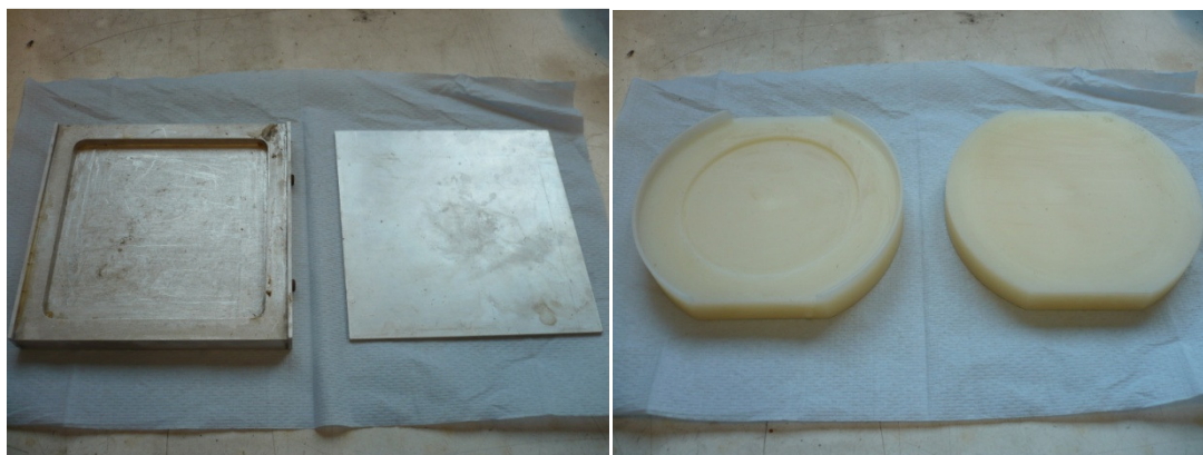
Figure 3.6: On left an aluminium mould with an internal depth of 5 mm and on the right hand side a nylon mould with an internal depth of 2mm
