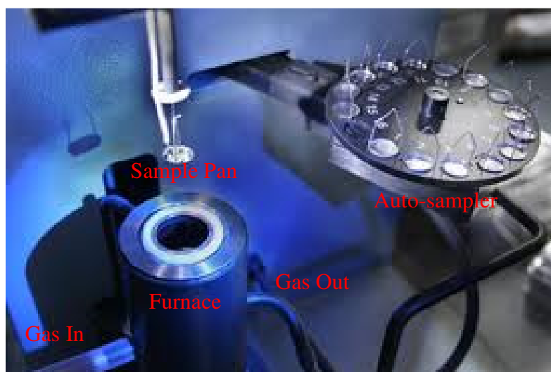
Figure 2.1: Design of a typical TGA instrument showing the sample pan, furnace, gas flow and auto-sampler
