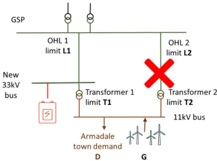
Figure 90 Armadale, N-1 scenario 1: OHL 2 or Transformer 2 not operational
