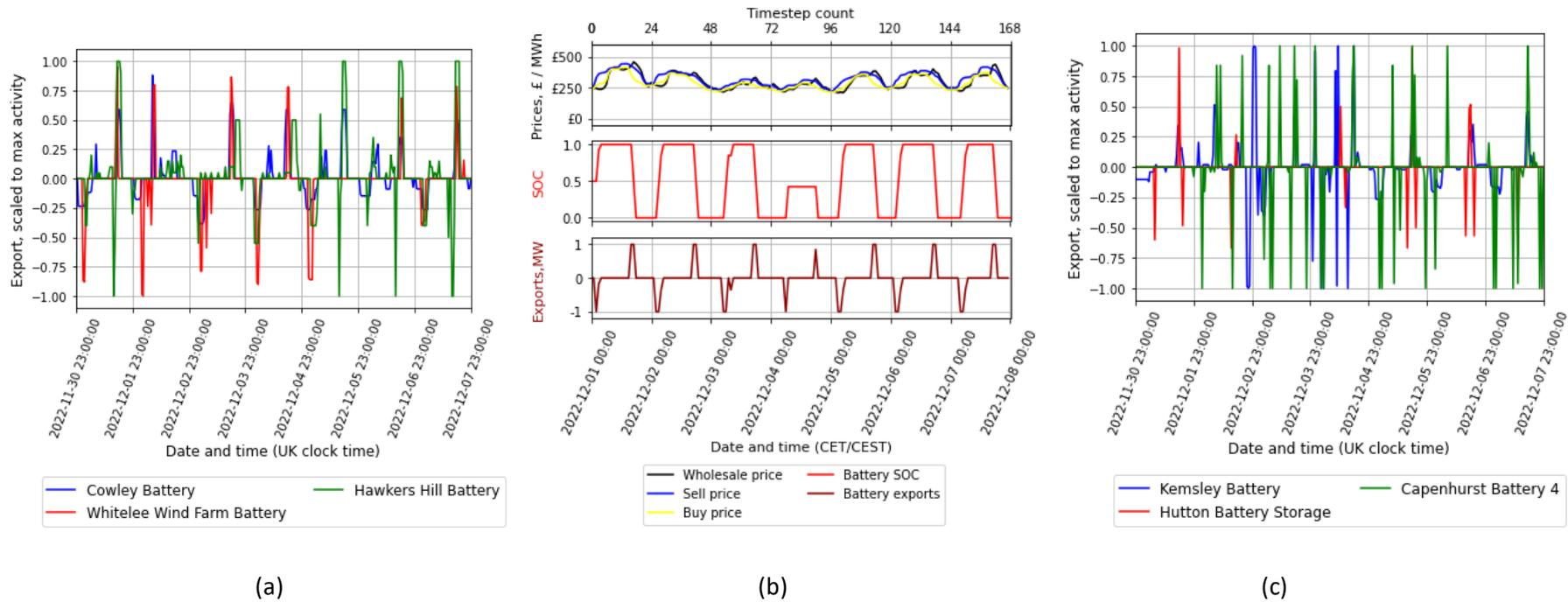
Figure 149 Winter week 3. (a) 3 batteries (Cowley, Whitelee and Hawkers Hill) engaged in broadly similar actions – 1 cycle per day - to those simulated (b). Cowley and Hawkers Hill batteries engaged in an additional daytime trade on several days. (c) shows 3 different batteries (Kemsley, Hutton and Capenhurst 4) engaging in numerous additional trades.
