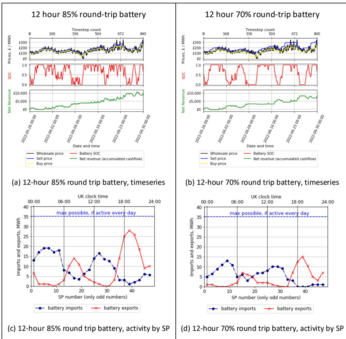
Figure 35 Summer case study. Effect of round-trip efficiency on activity of 12 hour battery, “best cashflow” scenario. Plots of battery activity timeseries, and activity by Settlement Period, for 85% and 70% round-trip batteries.
