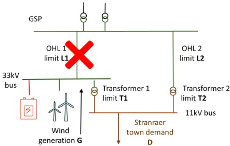
Figure 92 Stranraer circuit arrangement. N-1 scenario 2: OHL line 1 unavailable
