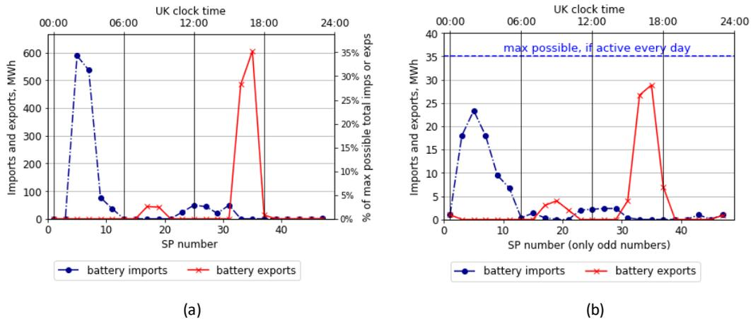
Figure 42 Winter: aggregate imports and exports by SP, (a) Pillswood 1 battery (1-hour resolution, as shown above in Figure 40), and 2-hour battery simulation (highest revenue scenario) as shown in Figure 30
