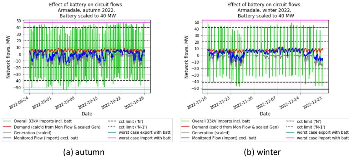
Figure 69 Effect of a 20 MW capacity battery on 33kV circuit flows at Armadale, in autumn and winter case study periods
