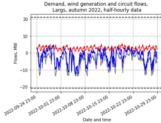
— Largs 11kV flow (demand) — Largs 33kV flow (11kV flow - wind gen)
