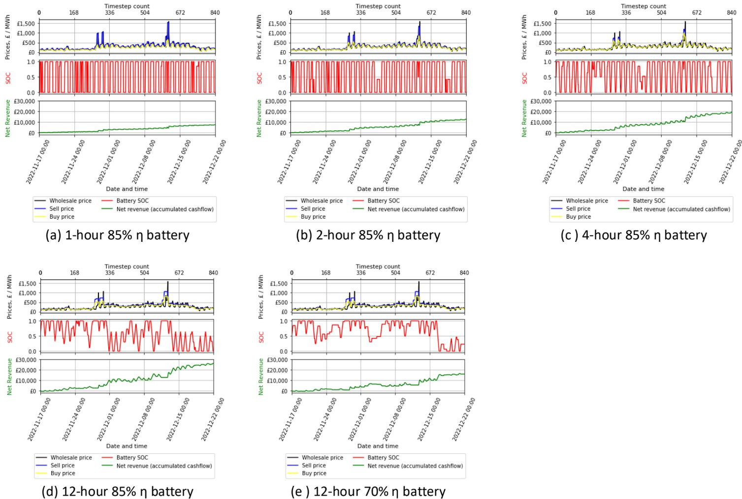
Figure 141 Timeseries plots of wholesale price, battery SOC and overall net revenue, for 1 MW battery (a) 1-hour, (b) 2-hour, (c) 4-hour, (d) and (e) 12-hour. (a) to (d) battery round-trip efficiency 85%; (e) 70%, Winter, all “best cashflow” scenarios.
