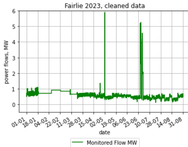
Fairlie “Monitored Flow” at 11kV bus. Sept 2022 – Aug 2023, as downloaded, and after “cleaning”. Scaled to 1.5 MW.
