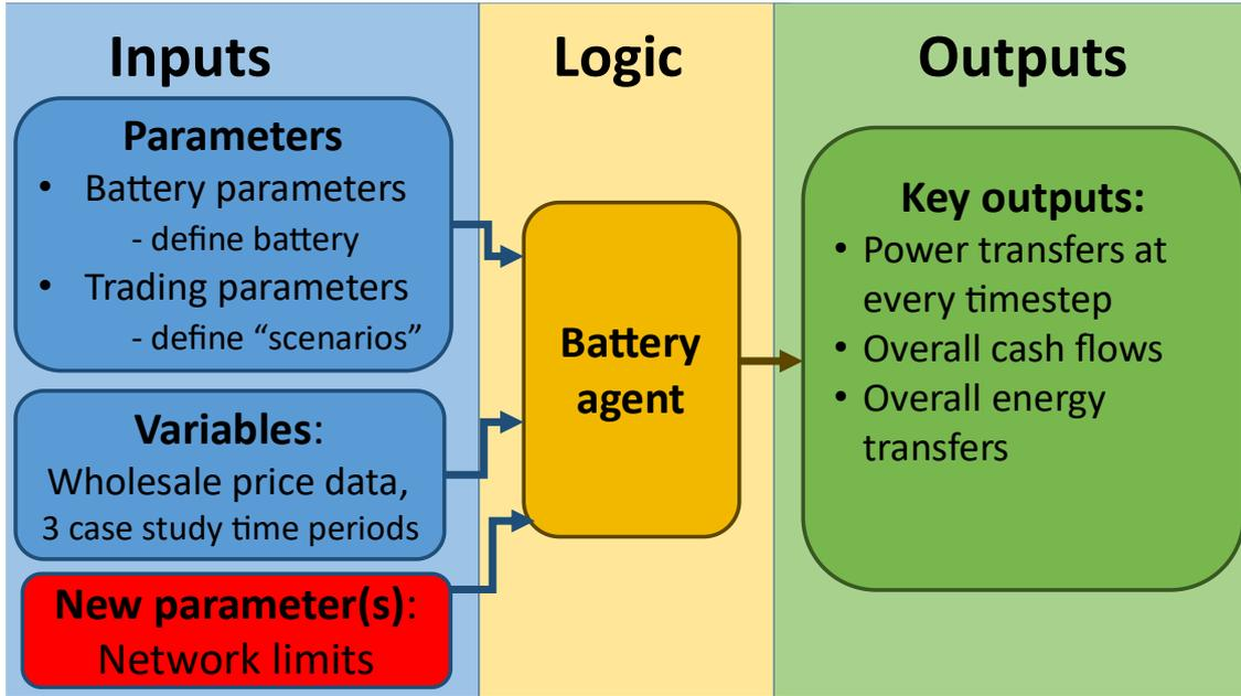
Figure 85 Battery model formulation amended to include network limits
