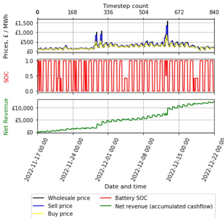
Figure 27 Winter case study (35 days), base case (1MW/2MWh) battery, “best cashflow” scenario. Timeseries of wholesale price, buy and sell prices, battery SOC and overall net revenue (accumulated cashflow). Parameters shown in Table 19
