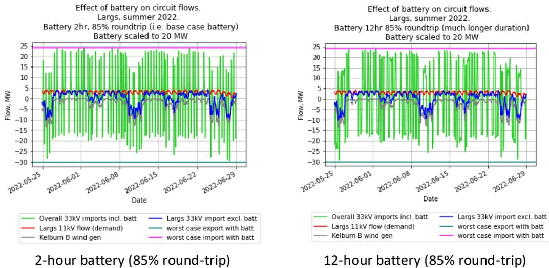
Figure 73 Effect of increasing battery duration from 2 hrs to 12 hrs (85% round trip). Largs, summer
