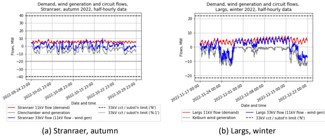
Figure 63 Time series 11kV substation flow, wind generation, and combined 33kV flows. Half-hourly resolution. (a) Stranraer, autumn 2022; (b) Largs, winter 2022
