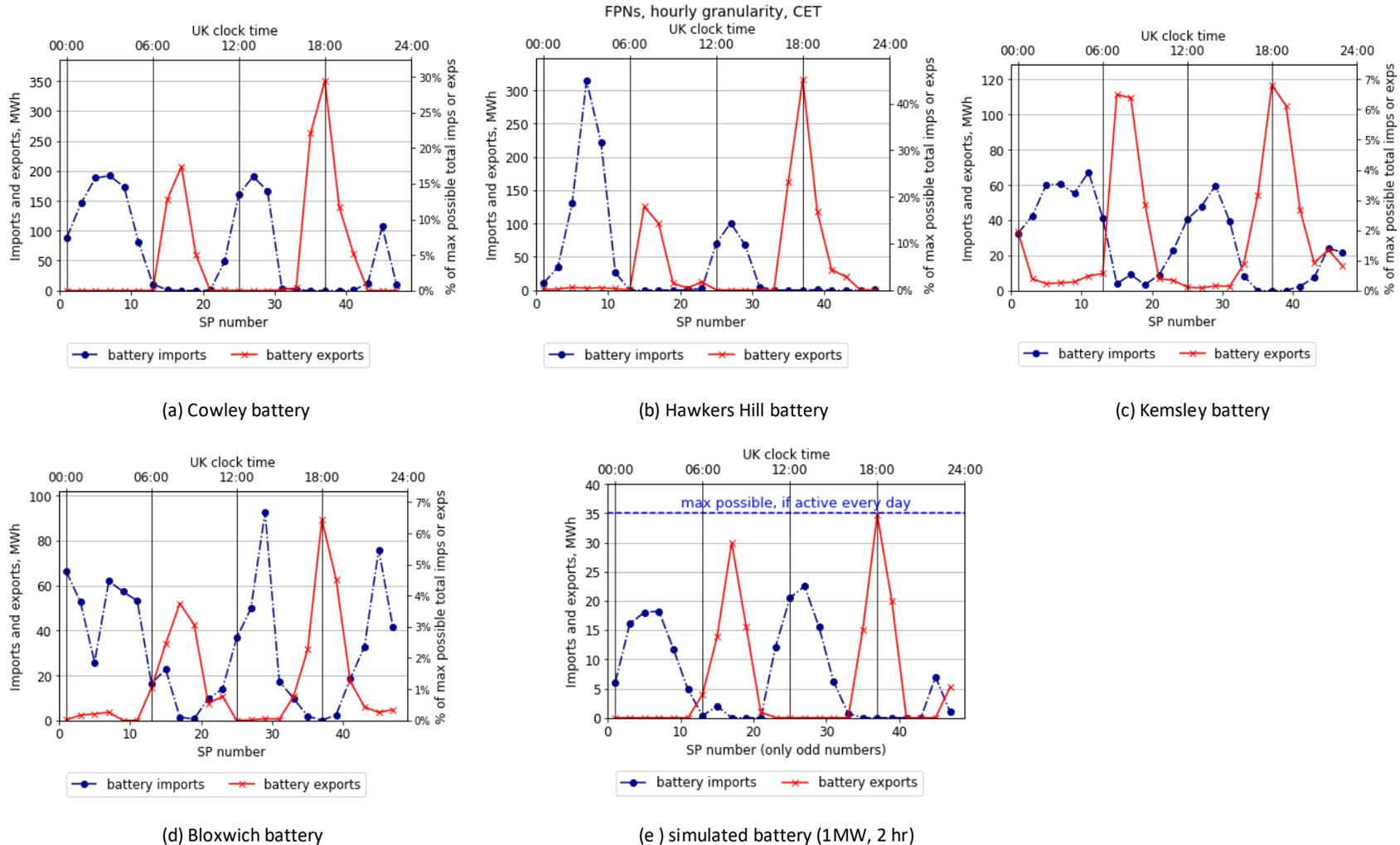
Figure 151 Autumn case study, diurnal battery activity. (a) – (d) real batteries, aggregate activity by SP, smoothed to 1-hour resolution for comparison with simulation; (e) simulated battery activity by SP. 1MW, 2 hr battery, “best cashflow” scenario.
