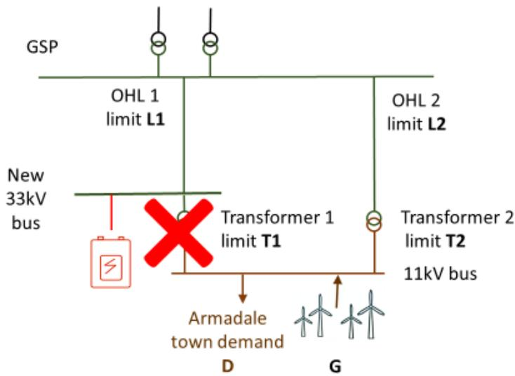
Figure 93 Armadale circuit. N-1 scenario 3: Transformer 1 unavailable
