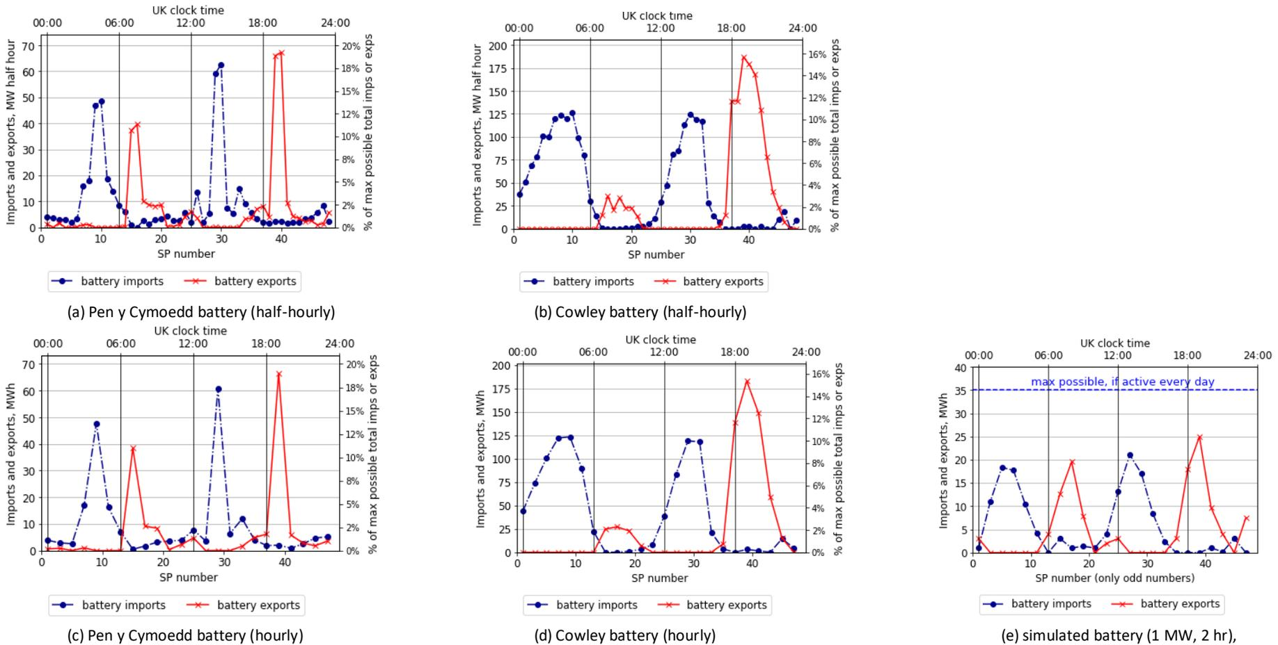
Figure 150 Summer case study, diurnal battery activity. (a) and (b) - aggregate activity by half-hour SP over the case study. (c) and (d) - aggregate activity by SP, smoothed to hourly resolution, for better comparison with simulated activity
