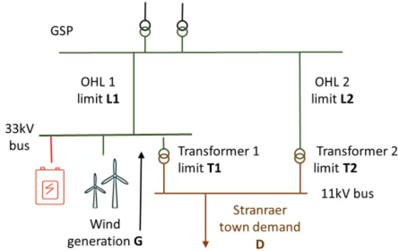
Figure 89 Circuit layout for Stranraer
