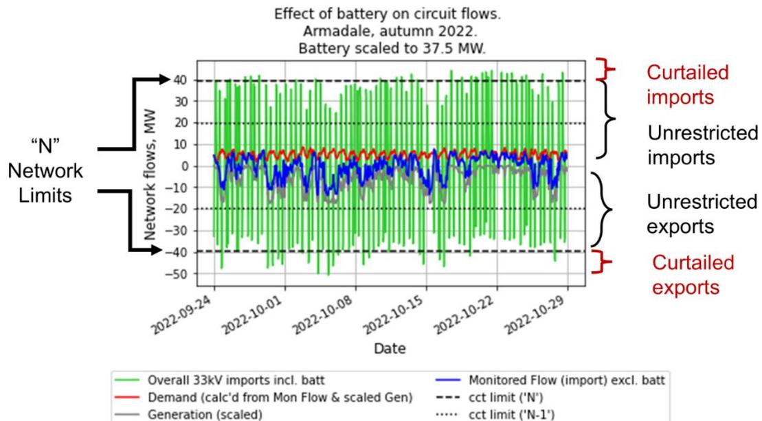
Figure 113 Timeseries network and simulated battery flows at Armadale, autumn. 2hr battery, 15 MW in excess of network headroom under ‘N’ conditions (37.5 MW). Showing unrestricted and curtailed imports and exports. Small degree of curtailment.
