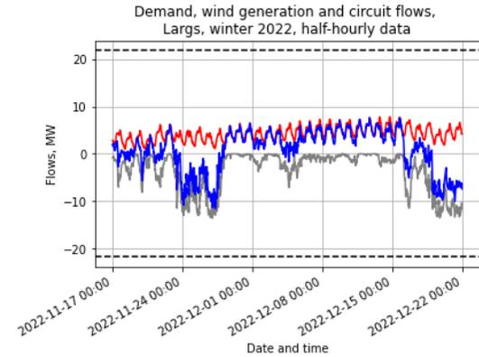
— Largs 11kV flow (demand) — Largs 33kV flow (11kV flow - wind gen)
