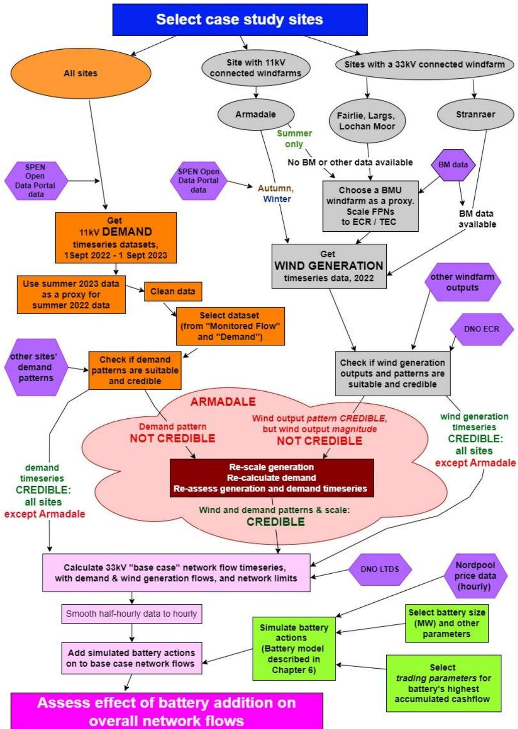
Figure 59 Overview of method for calculation of effect of a battery on DN power flows <sup>59</sup>
