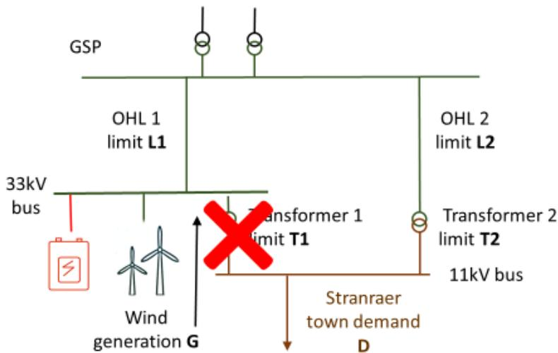
Figure 94 Stranraer circuit. N-1 scenario 3: Transformer 1 unavailable
