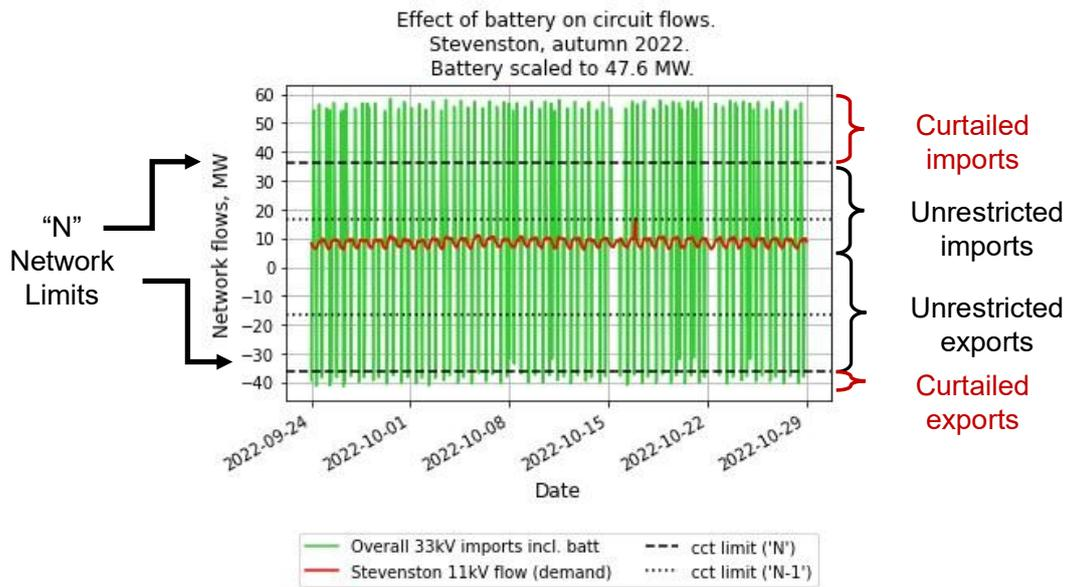
Figure 114 Timeseries network and simulated battery flows at Stevenston, autumn. 2hr battery, 25 MW in excess of network headroom (47.6 MW). Showing unrestricted battery trades would breach network import and export limits twice most days.
