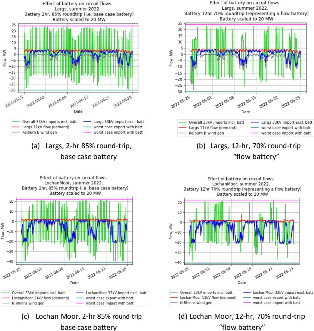
Figure 79 Comparing simulated lithium 2 hour and 12-hour flow battery actions on network flows at Largs (a, b) and Lochan Moor (c, d) SUMMER case study
