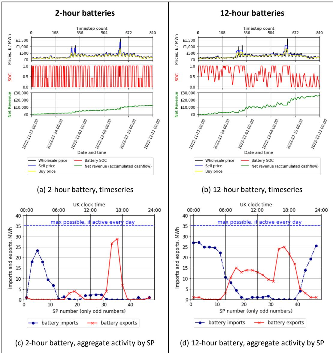
Figure 34 Comparing 2-hour and 12-hour battery simulations. Winter case study. Both batteries 85% round-trip efficiency. Plot of timeseries, and of aggregate activity by Settlement Period
