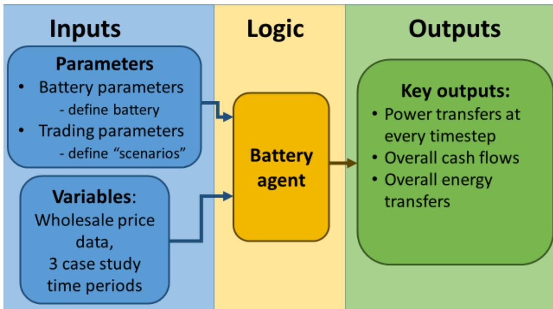
Figure 16 Schematic of battery model formulation
