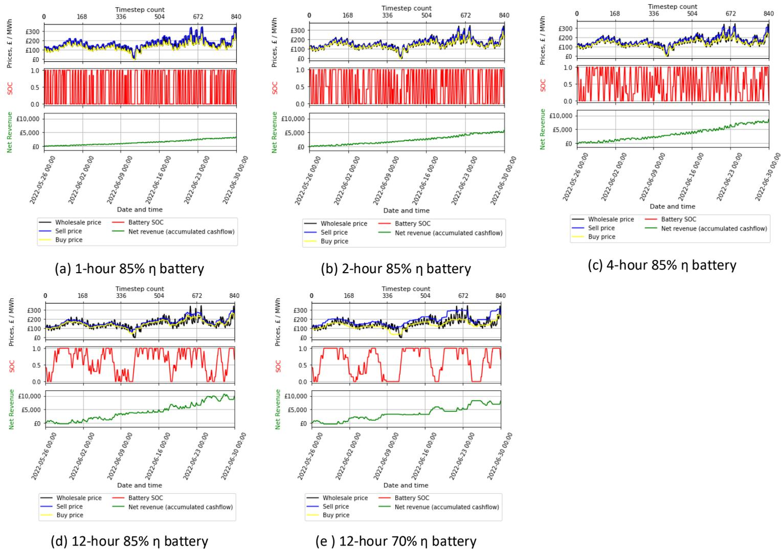
Figure 137 Timeseries plots of wholesale price, battery SOC and overall net revenue, for 1 MW battery (a) 1-hour, (b) 2-hour, (c) 4-hour, (d) and (e) 12-hour. (a) to (d) battery round-trip efficiency 85%; (e) 70%, Summer, all “best cashflow” scenarios.
