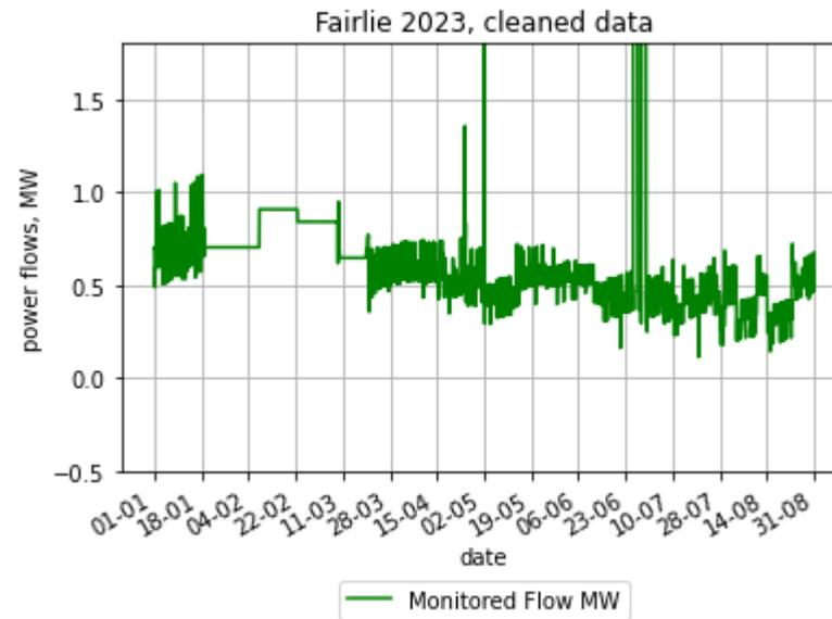
Lochan Moor flows: A combination of “Monitored Flows” flows from Auchneel and Barrhill 11kV buses, Sep 2022 – Aug 2023, as downloaded and after “cleaning”
