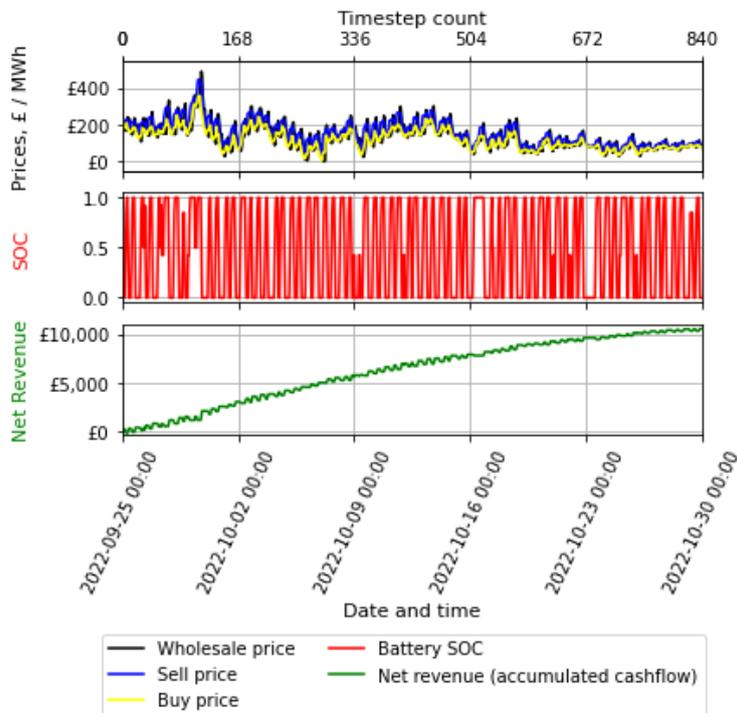
Figure 26 Autumn case study (35 days), base case (1MW/2MWh) battery , “best cashflow” scenario. Timeseries of wholesale price, buy and sell prices, battery SOC and overall net revenue (accumulated cashflow). Parameters as shown in Table 19
