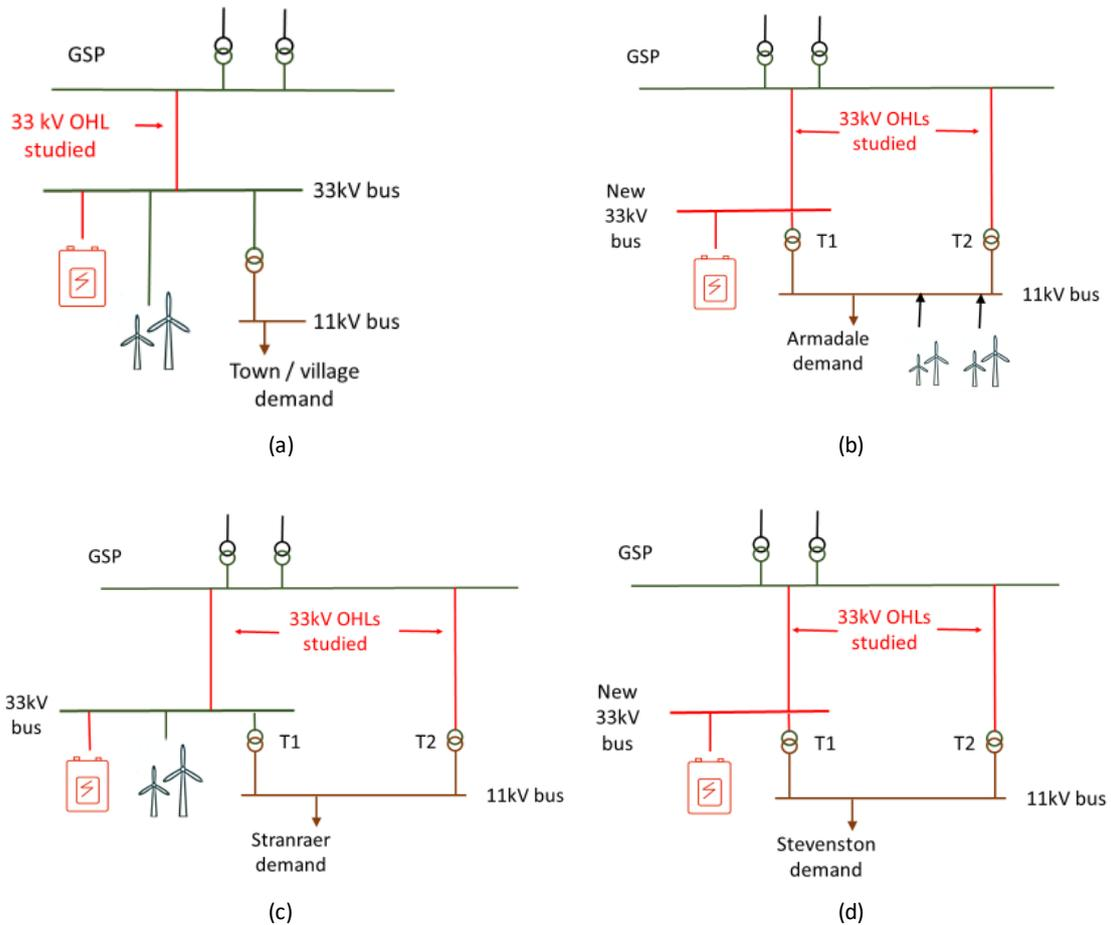
Figure 65 Battery locations, near (a) Fairlie, Largs and Lochan Moor; (b) Armadale; (c) Stranraer; (d) Stevenston
