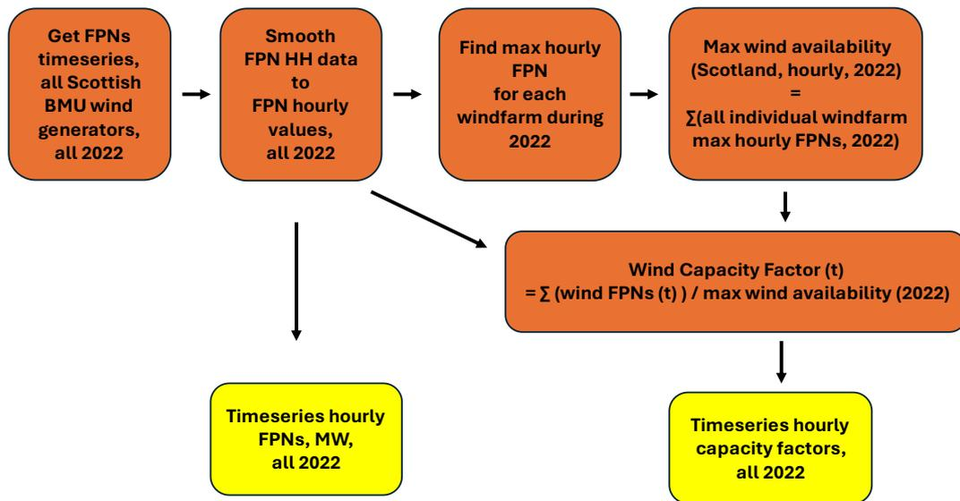
Figure 43 Schematic of approach to obtain timeseries wind availability timeseries in MW and as a capacity factor
