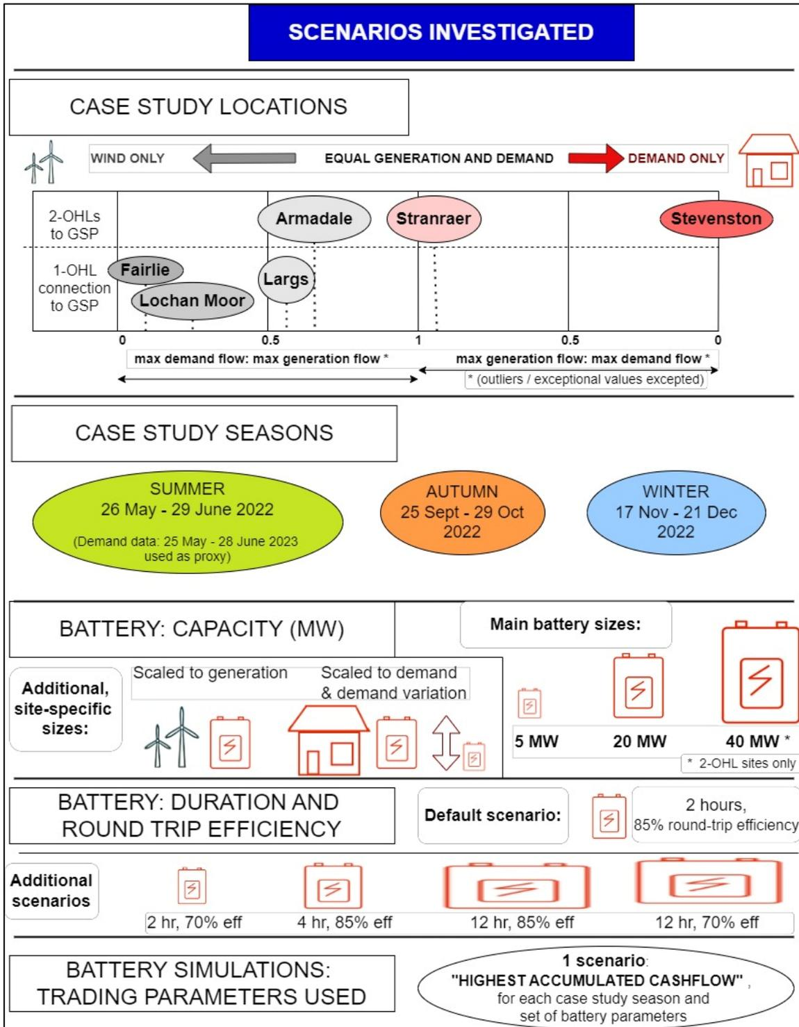
Figure 60 Overview of scenarios investigated: location, season, battery capacity and other batter parameters
