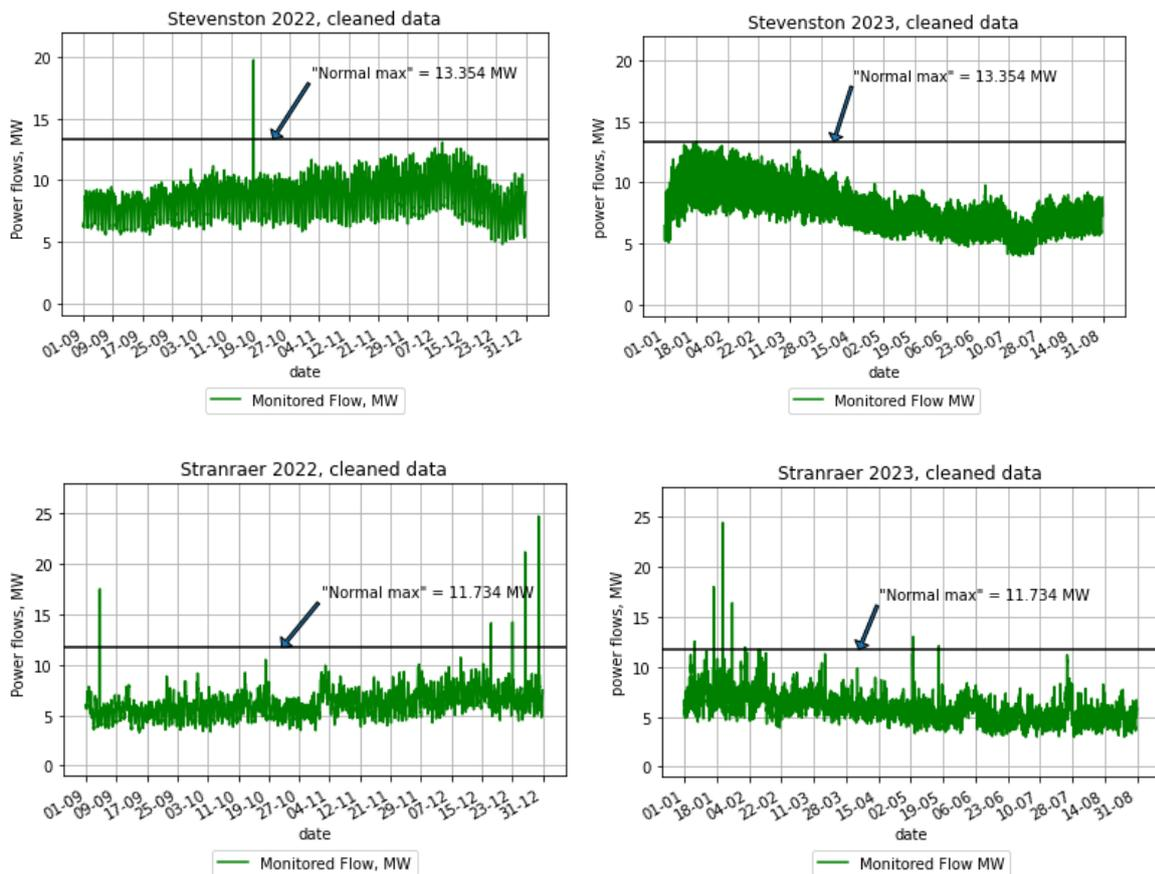
Figure 193 Monitored Flows at Stevenston and Stranraer (after cleaning), 2022 and 2023, showing “normal max” flows
