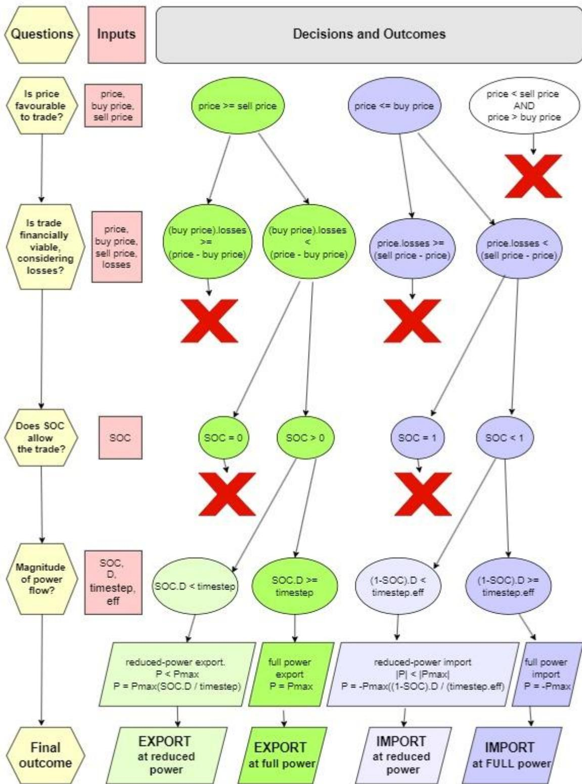
Figure 21 Battery agent heuristics for determining action at each time step.
