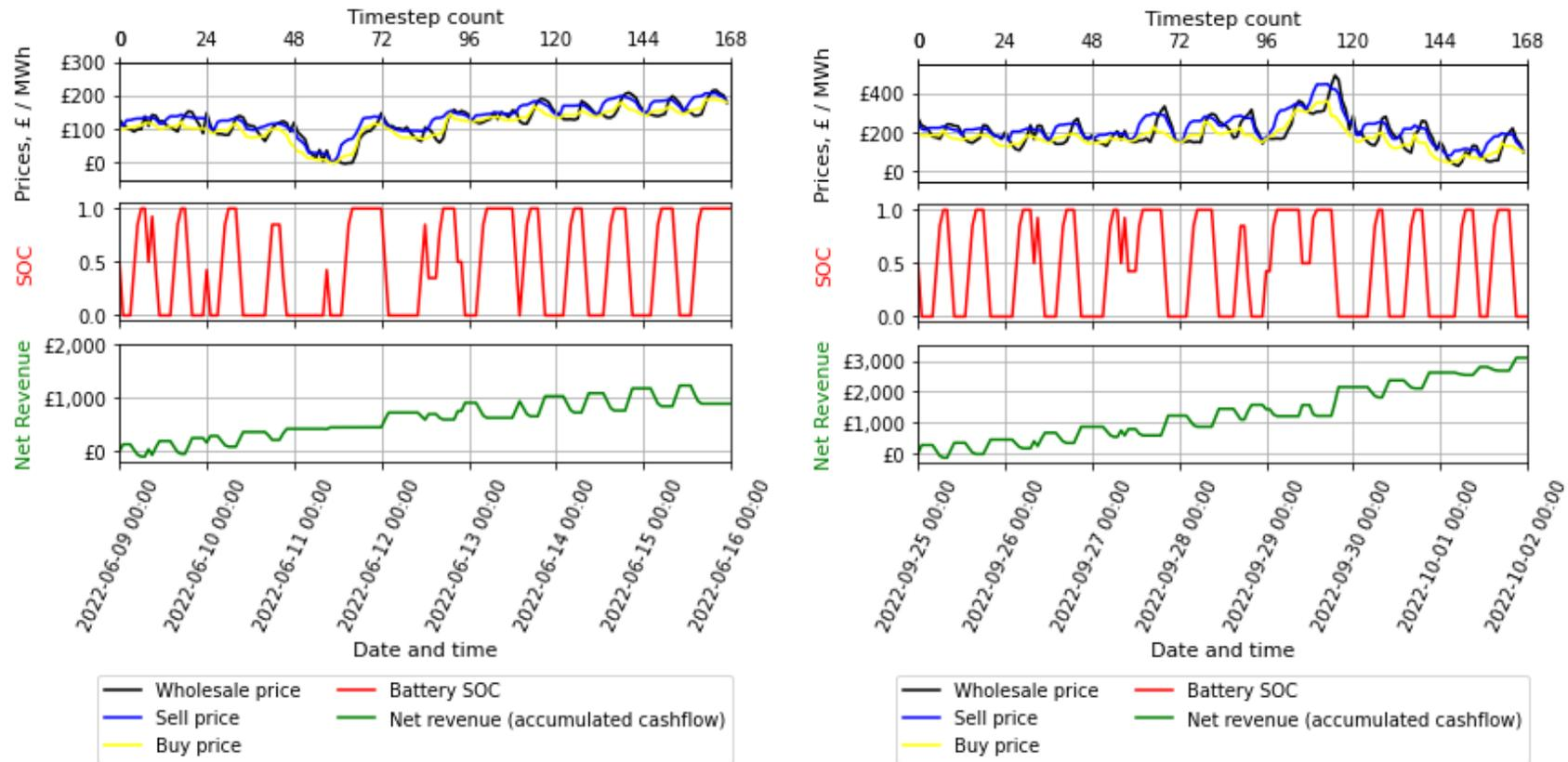
Figure 28 Two 1-week plots of battery simulation – illustrating changeable patterns of cycling. Summer, 3rd week, and Autumn, 1<sup>st</sup> week, respectively. Base case (1MW/2MWh) battery, “best cashflow” scenario in both cases.
