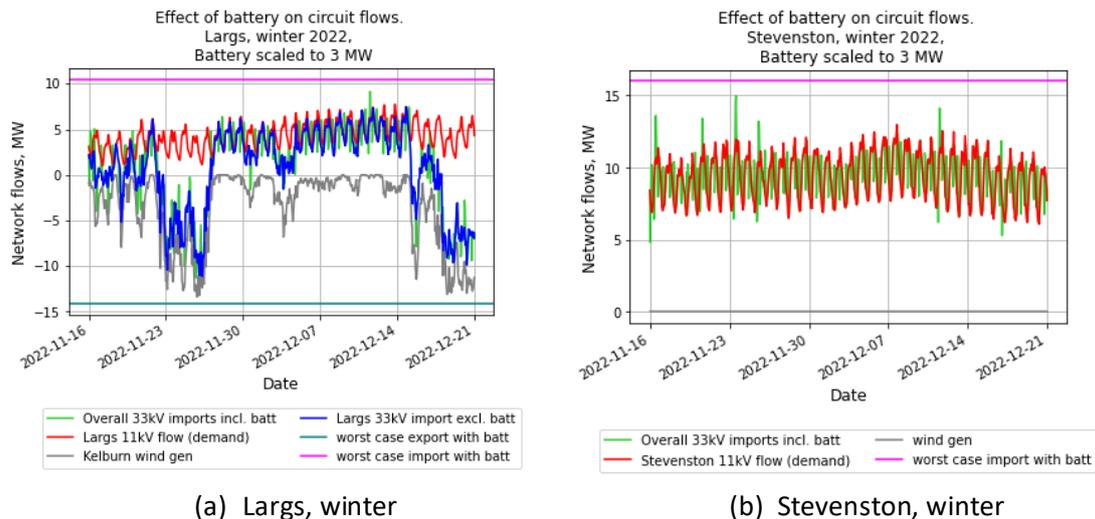
Figure 66 3 MW battery in winter, generally reducing network flows, Largs and Stevenston.
