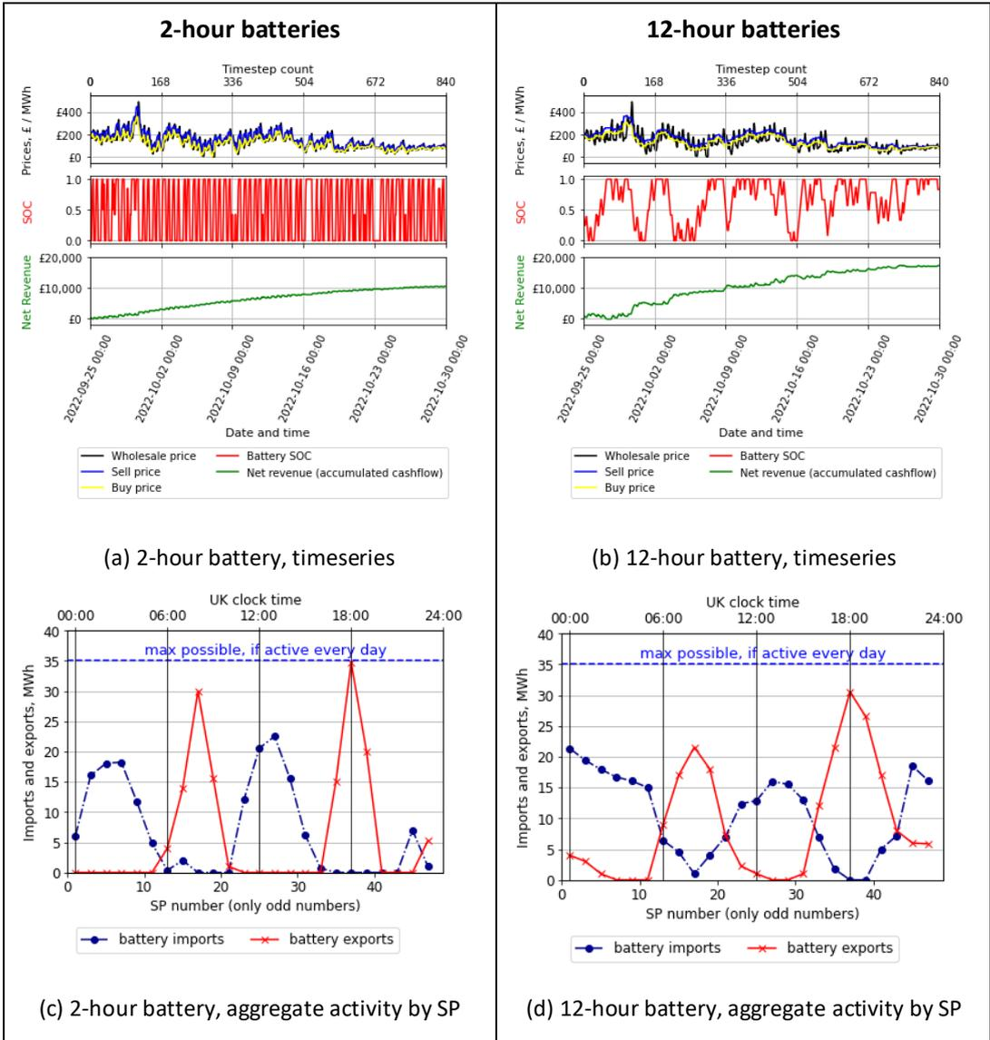
Figure 33 Comparing 2-hour and 12-hour battery simulations. Autumn case study. Both batteries 85% round-trip efficiency. Plots of timeseries, and of aggregate activity by Settlement Period
