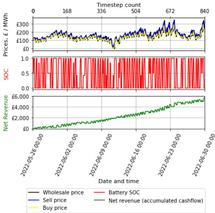
Figure 25 Summer case study (35 days), base case (1MW/2MWh) battery, “best cashflow” scenario. Timeseries of wholesale price, buy and sell prices, battery SOC and overall net revenue (accumulated cashflow). Parameters in Table 19
