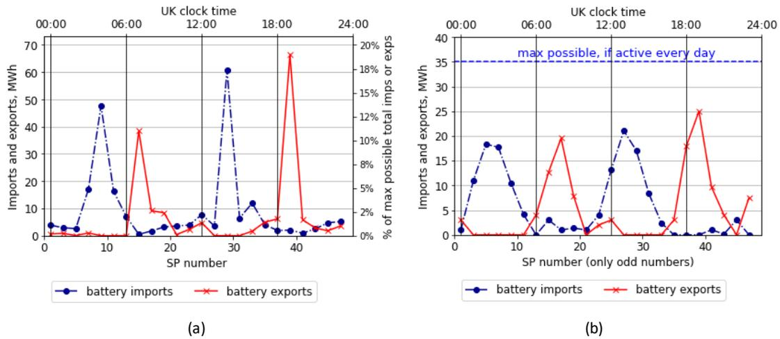
Figure 41 Summer: aggregate imports and exports by SP, (a) Pen y Cymoedd battery (1-hour resolution), and (b) 2-hour battery simulation (highest revenue scenario) as shown in Figure 30
