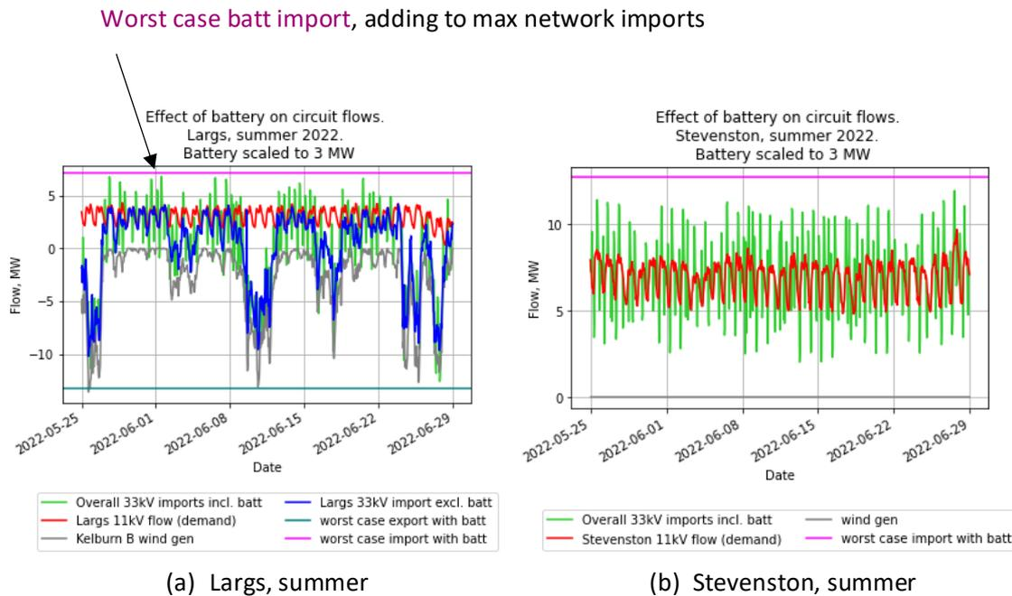
Figure 67 Effect of a 3 MW battery in summer, generally increasing network import flows, Largs and Stevenston.
