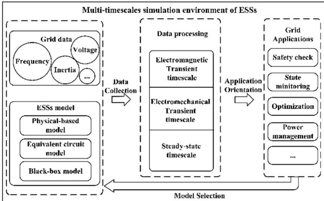
Figure 15 Multi-timescale simulation environment of energy storage systems. Reproduced from Mao et al [200]
