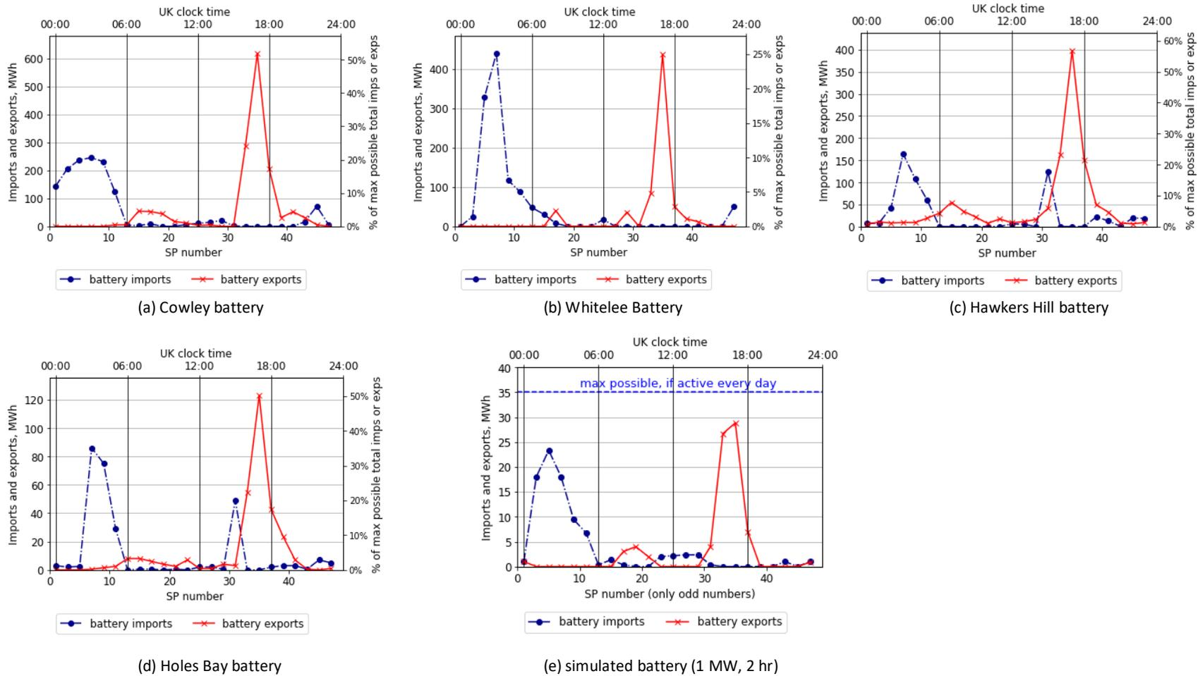
Figure 153 Winter case study. Diurnal patterns of battery activity, batteries with similar behaviour to simulations. (a) - (d) real batteries, aggregate activity by SP over case study. Activity smoothed to hourly resolution to match simulation. (e) simulated activity of 1 MW 2-hr battery, “best cashflow” scenario.
