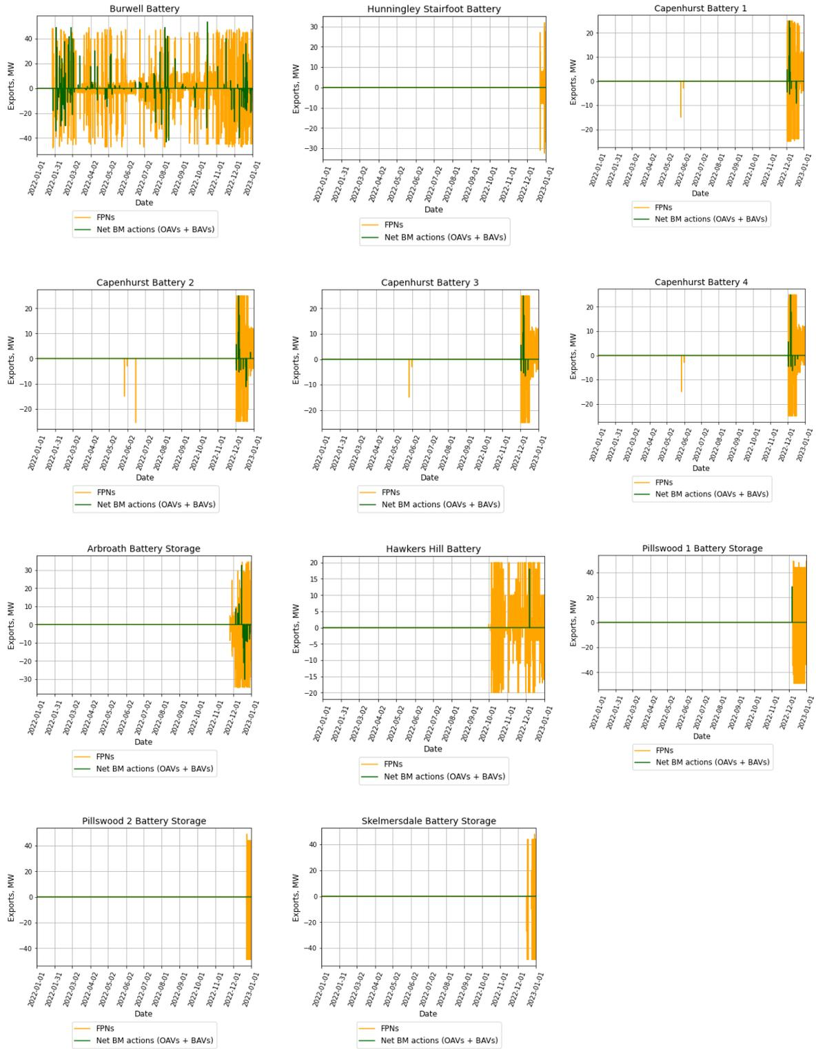
Figure 126 Timeseries charts of GB real battery FPNs and BM trades during 2022 [272]
