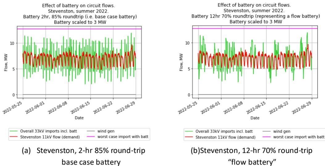
Figure 81 Comparing simulated lithium 2 hour and 12-hour flow battery actions on network flows at Stevenston, (charts a, b, respectively) in SUMMER.
