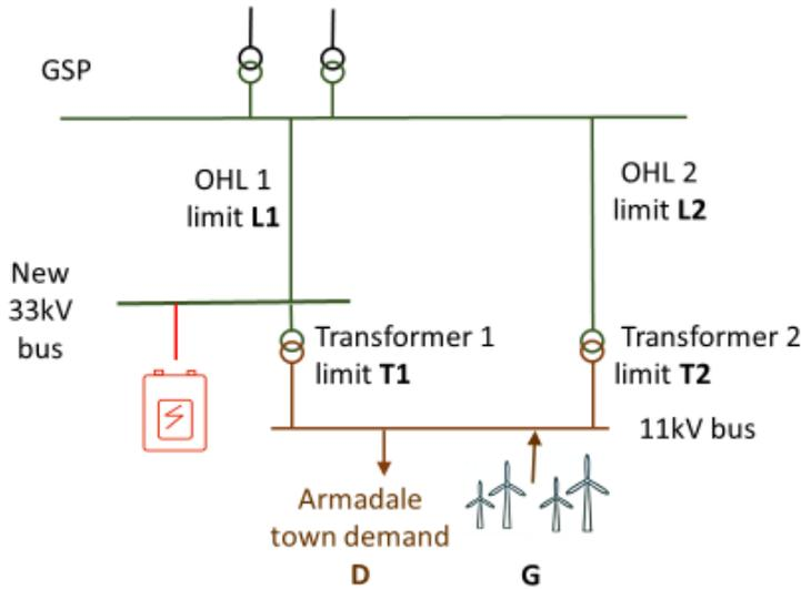
Figure 88 Circuit layout for Armadale
