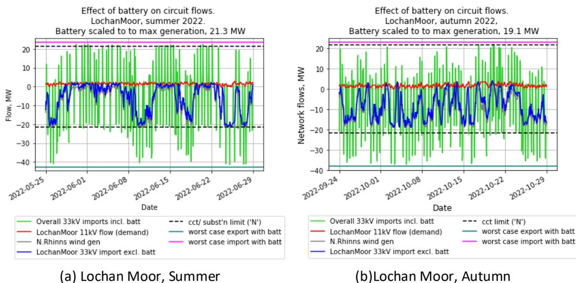
Figure 70 Effect of a battery, sized to the windfarm's capacity, on overall network flows. Lochan Moor, summer and autumn
