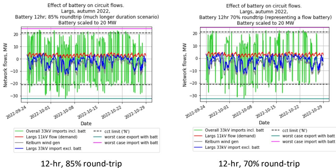
Figure 75 Effect of reducing the round trip efficiency of a 12-hr battery from 85% to 70%. Largs, autumn
