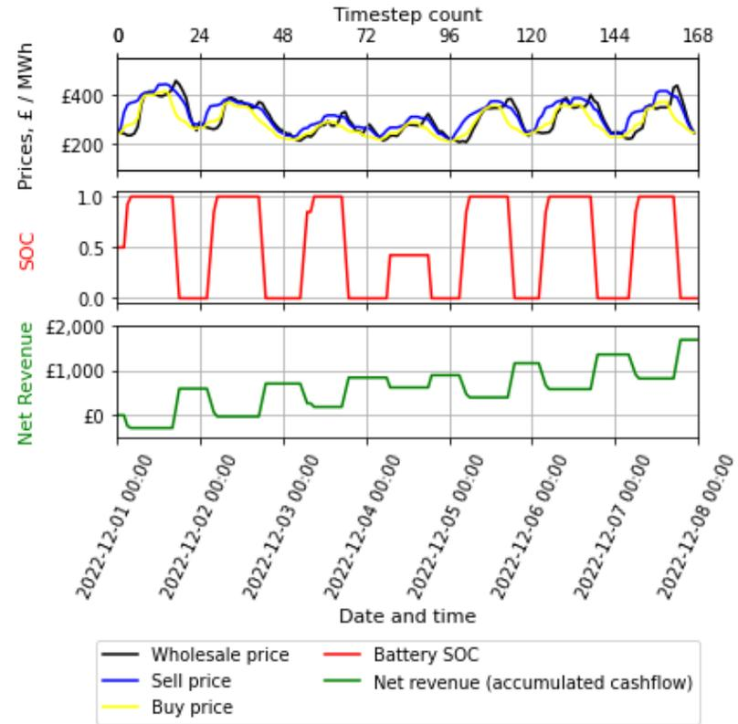
Figure 29 Two 1-week plots of battery simulation – illustrating regular trading patterns. Autumn, 2<sup>nd</sup> week, regular 2 cycles / day, and Winter, 3<sup>rd</sup> week, regular 1 cycle/ day. Base case (1MW/2MWh) battery, “Best cashflow” scenarios in both cases.
