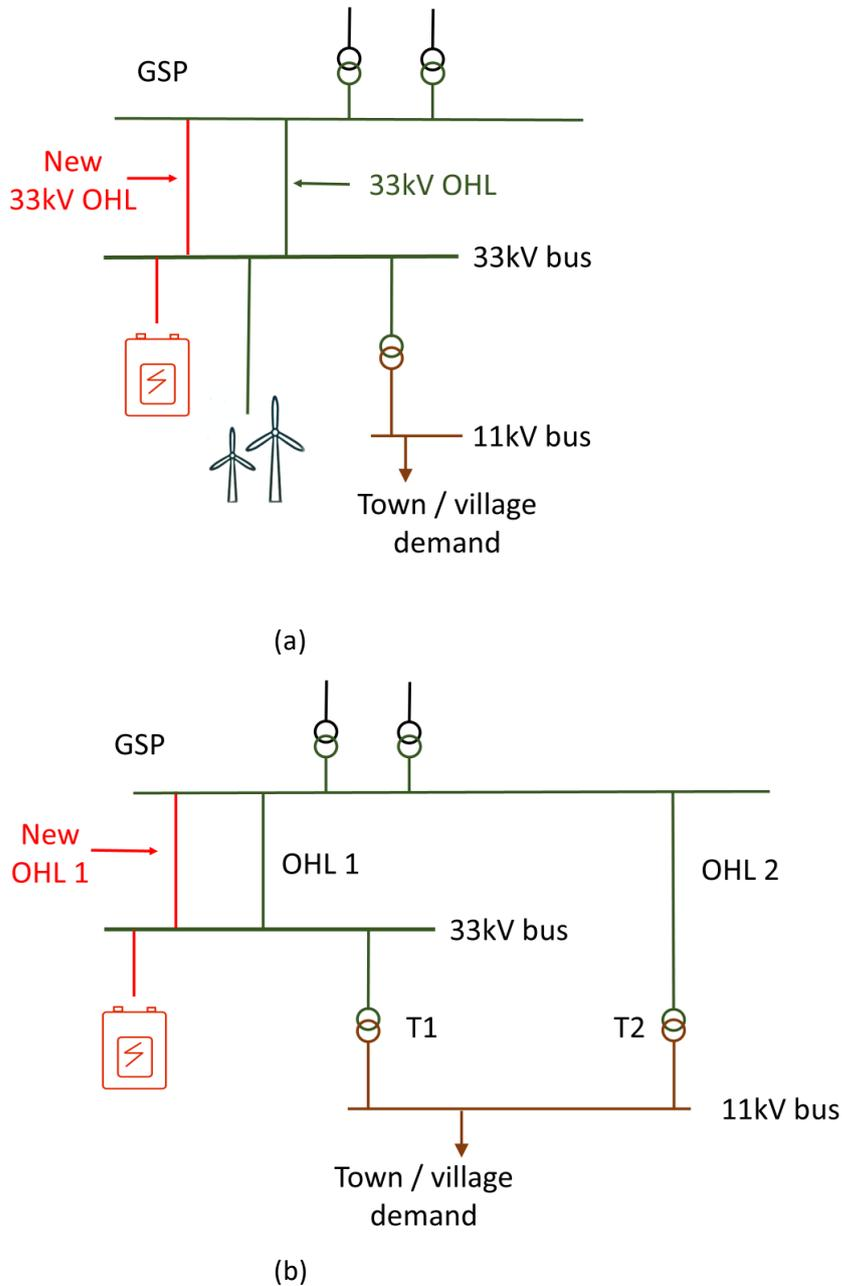
Figure 118 Reinforcement scenario considered for (a) the single-OHL case study locations; (b) the 2-OHL case study locations
