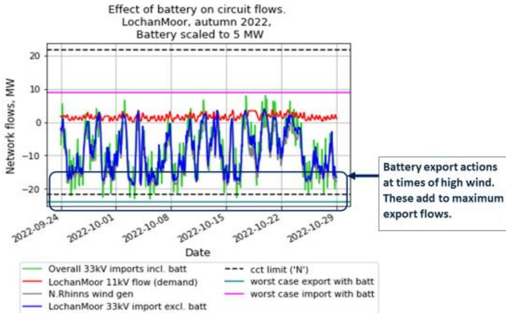
Figure 78 Effect of a 5 MW 2-hour battery on network flows at generation-dominated Lochan Moor. Autumn case study.
