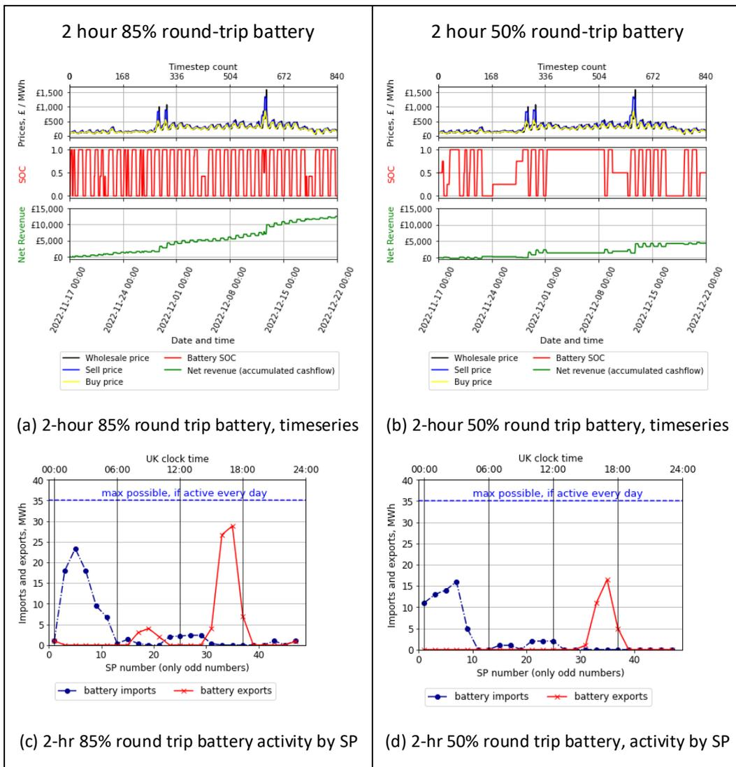
Figure 36 Winter case study. Effect of round-trip efficiency on activity of 2 hour battery, “best cashflow” scenario. Plots of battery activity timeseries, and activity by Settlement Period, for 85% and 50% round-trip batteries.
