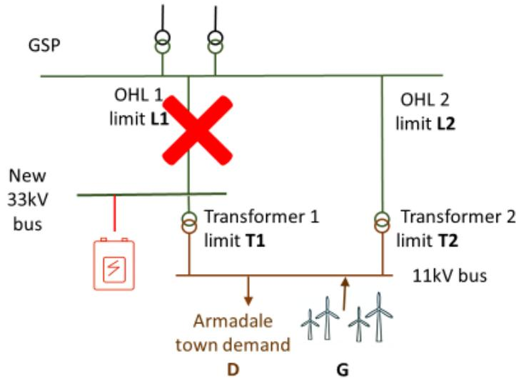
Figure 91 Armadale circuit arrangement. N-1 scenario 2: OHL line 1 unavailable
