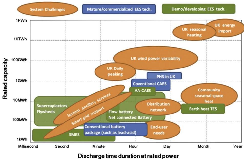
Figure 2 Electrical energy storage technologies with challenges to the UK energy systems. Reproduced from [56]
