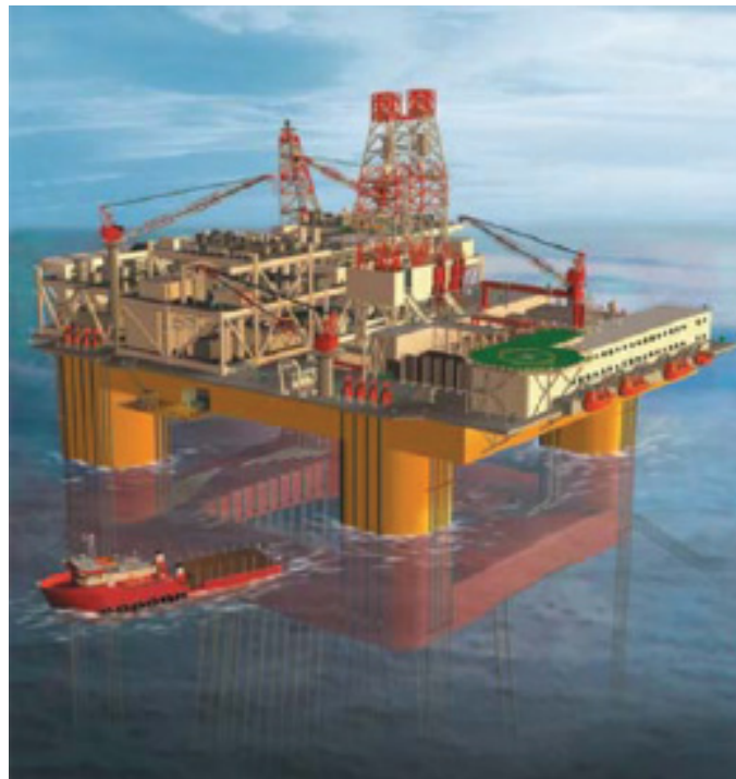
Figure 1.4—4 Semisubmersible floating system (Arnold, 2007)
