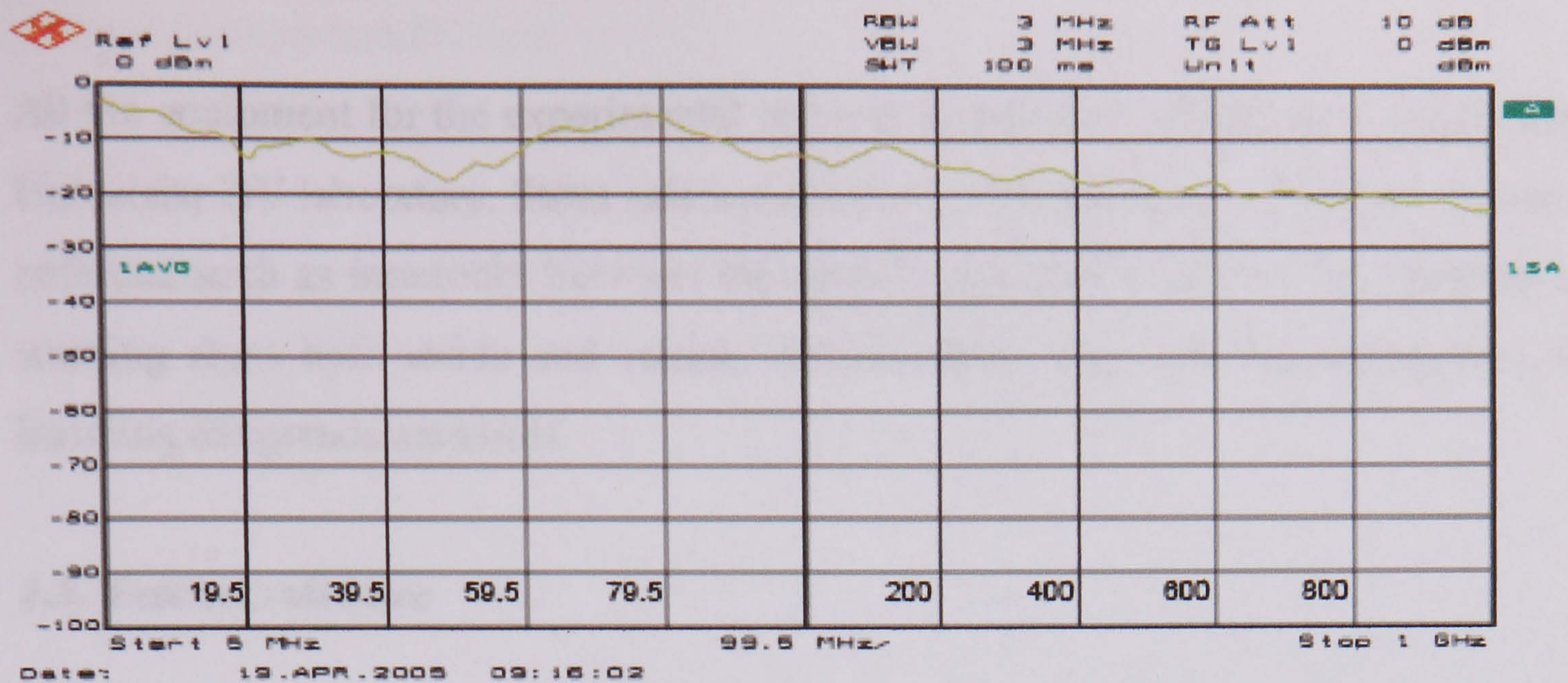
Figure 4.11. Frequency response of the protection box with the improved circuit.
