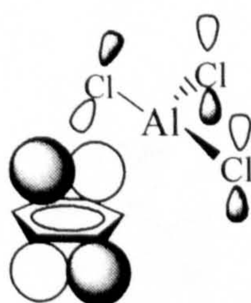
Figure 2.7 Backbonding from the 3p Cl orbital to the benzene HOMO
