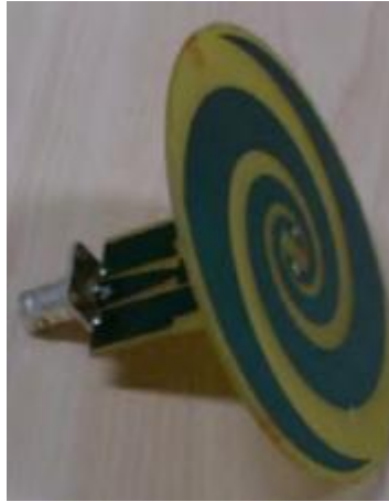
Figure 3.12 : Experimental spiral UHF PD sensor that was immersed in an oil-filled tank [101].
