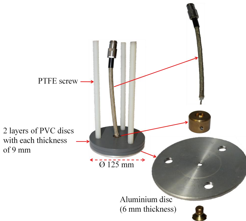
Figure 5.5: Experimental disc-type UHF PD sensor.
