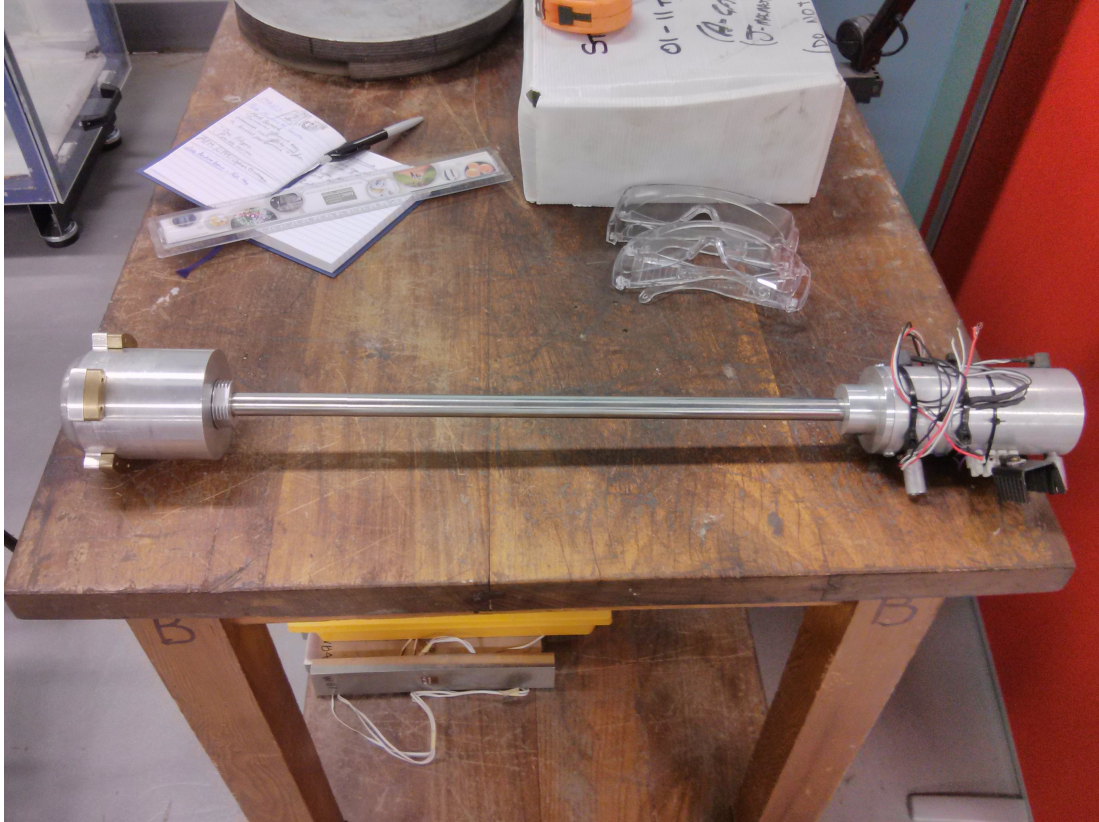
Figure 4.2: Detachable barrel with light gates affixed for measurement of velocity.
