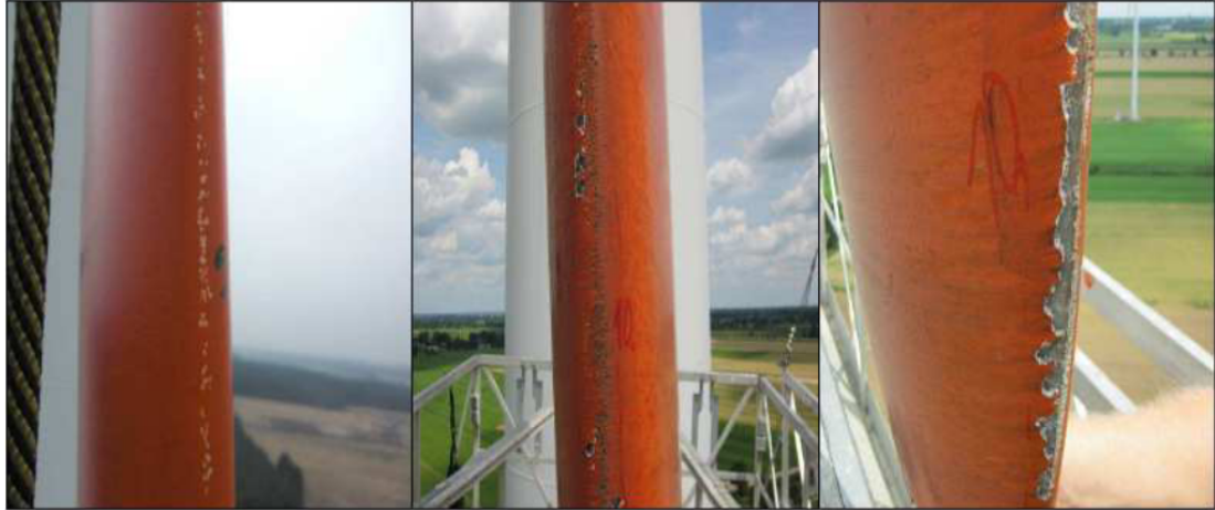
Figure 2.11: Progression of leading edge erosion. 1 - coating removal, 2 - damage of the matrix 3 - delamination and fibre damage [9].
