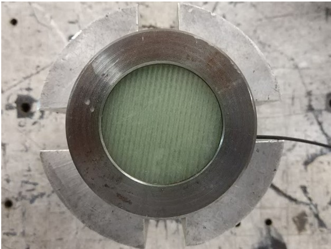
Figure 4.17: A composite sample in the clamping arrangement.
