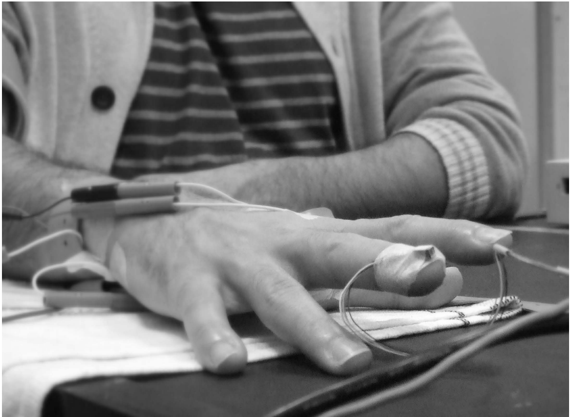
Figure 4.9: Illustration of the third contraction task; extension of the fore-finger and middle finger while the rest of the hand is supported on the table. Note the accelerometer positioned on the end of the middle finger.
