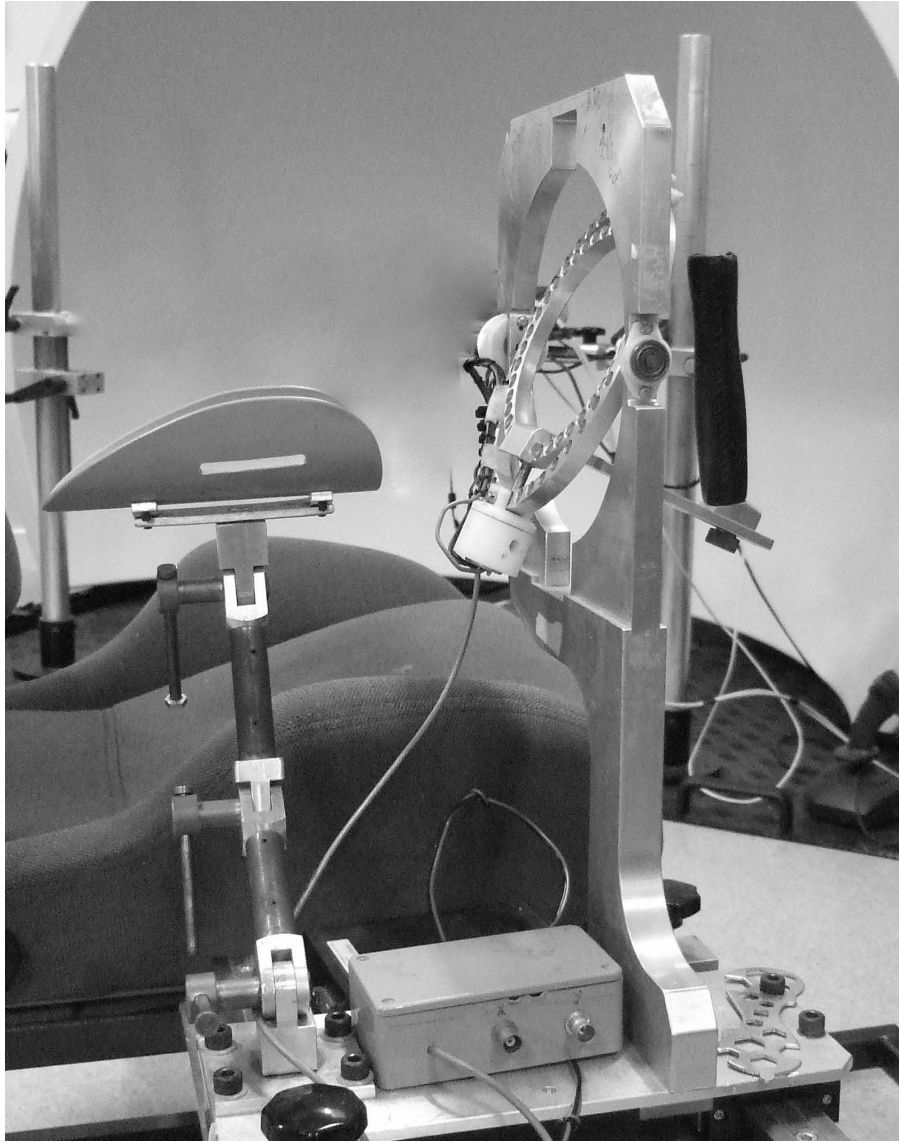
Figure 4.7: Manipulandum device used in the first and second contraction task to encourage participants to co-activate all the muscles of interest.
