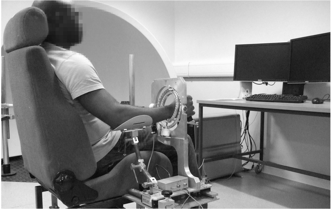
Figure 4.8: Participant's position during the fist and second contraction tasks. Participant is relaxed, the elbow is supported and the hand grips the joystick to activate all the muscles of interest.
