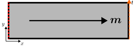
Figure 5.1: Experiments of Section 5.5.2: View from above of the FeCoSiB bar of dimensions (20\ell_{\text{ex}}, 6\ell_{\text{ex}}, 6\ell_{\text{ex}}) .
