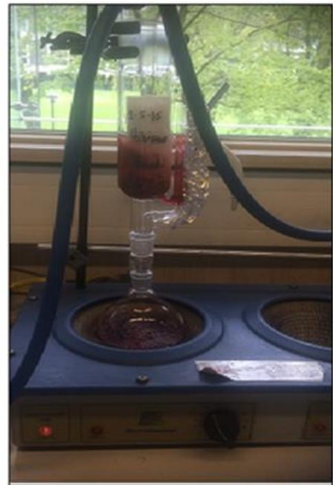
**Figure 2.1: Soxhlet apparatus.** (A) Assembly of the apparatus (B) Photograph of the Soxhlet apparatus used for the extraction of the fine powdered dried calyces of *H. sabdariffa*.
