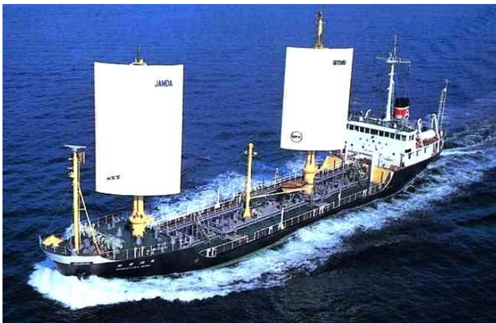
Figure 4 - Tanker ‘‘Shin-Aitoku Maru’’fitted with wingsails (Ariffin et al., 2020).
