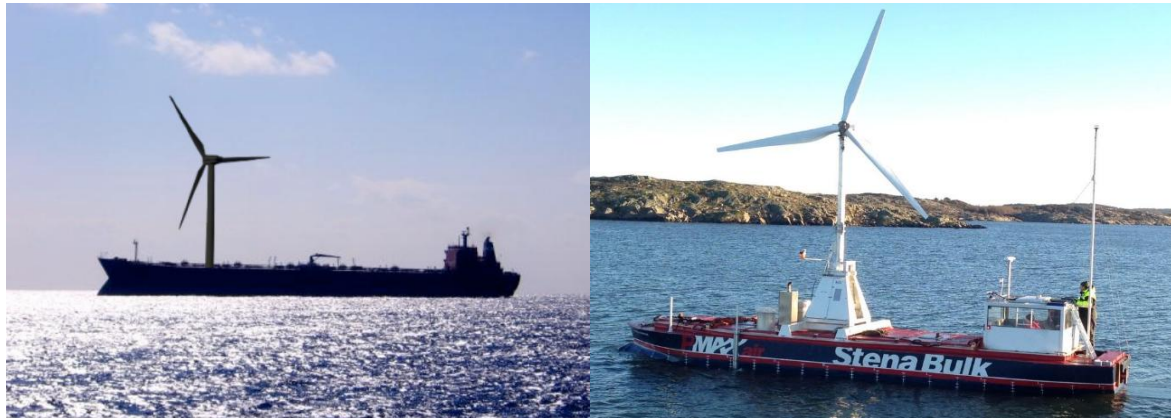
Figure 9. Illustration of a Vestas V39/600 wind turbine onboard a 150m tanker (Bockmann and Steen, 2011) and model tanker "Airmax" (Carlson and Nilsson, 2015).
