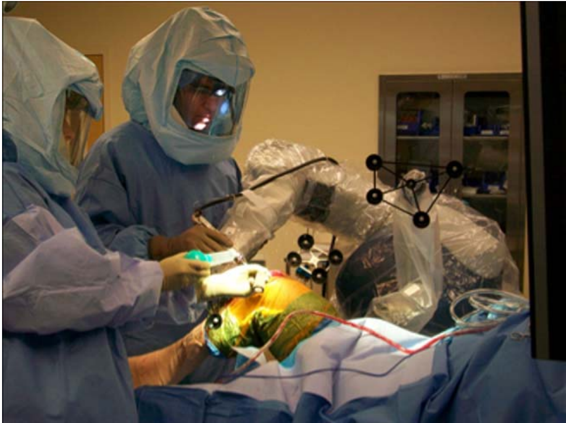
Figure 2.13 A semiactive haptically-guided robotic arm used in total knee arthroplasty—“Makoplasty” (Mako Surgical) (K. Logishetty et. al 2010).
