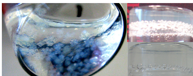
Figure 5.7 (left) Particulate appearance of the P5YL system; (right) representative hydrogel examples (top) P4YL , (bottom) F4YL . Similar in appearance to other hydrogel systems.
