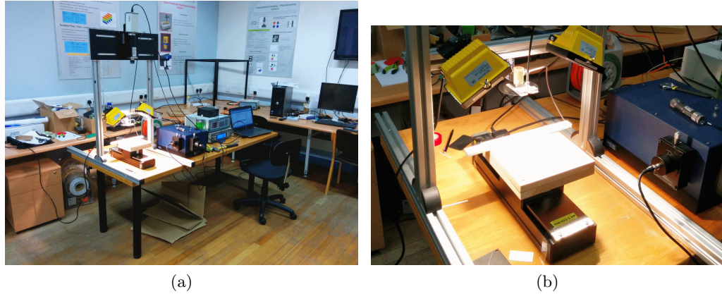
Figure 5.2: HSI system used for imaging the sponges. (a) Entire setup. (b) Close up of a sponge being imaged on the translation stage.
