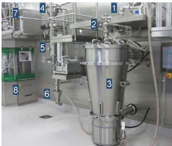
Figure 1.7. Continuous manufacturing platform Consigma™-25. 1) powder feeding system, 2) twin-screw granulator, 3) fluid bed dryer, 4 and 5) post-processing area of granules including sieving, 6 and 7) blenders for the addition of extragranular excipients and 8) tablet press. Reproduced from (Vercruyse et al., 2013)
