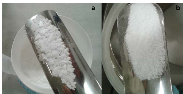
Figure 3.1. Image of PEG 6000 as flakes before milling (a) and as granules after milling (b)
