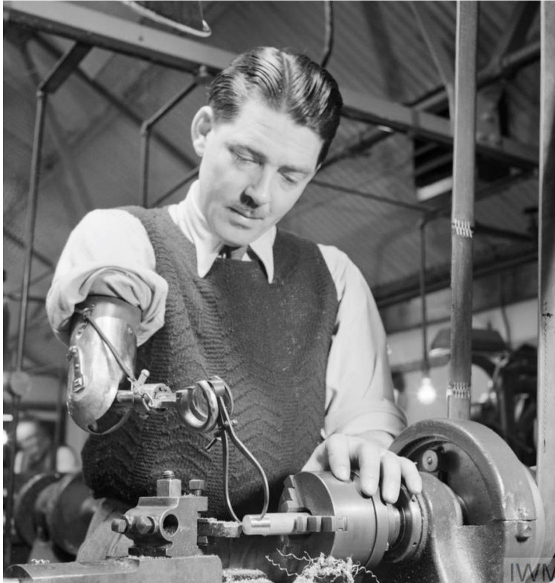
Figure 2.4: Mr T. G. Phillips operates a lathe at a factory somewhere in Britain. He is producing artificial limbs and uses his own artificial arm to work the lathe (1944). Photograph taken by Ministry of Information Photo Division, IWM, Catalogue No.D17829.
