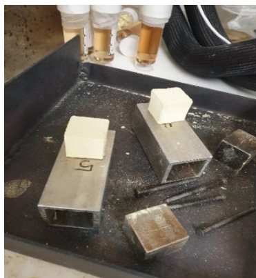
Figure 5.4. A photograph of the tooling used to consolidate the particles and produce the stock shape samples after demoulding
