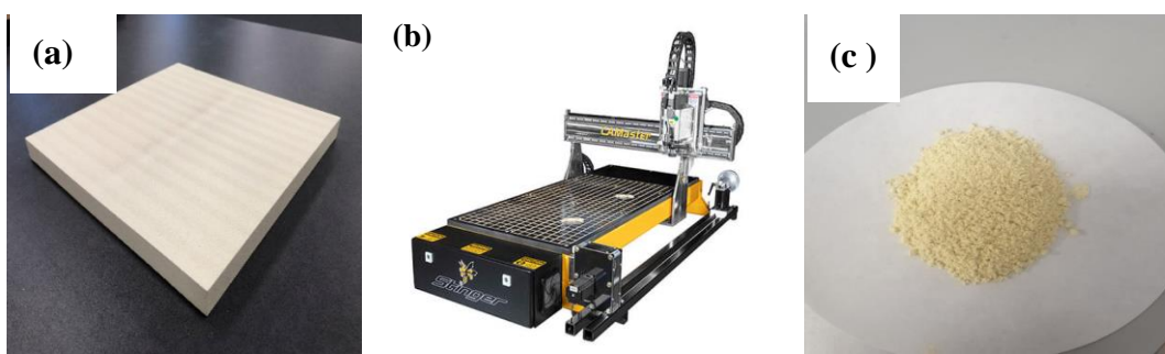
Figure 4.4 (a) PI stock shape, (b) stinger for milling the PI stock shape, and (c) PI powder aerogel produced through dry milling of PI stock shape
