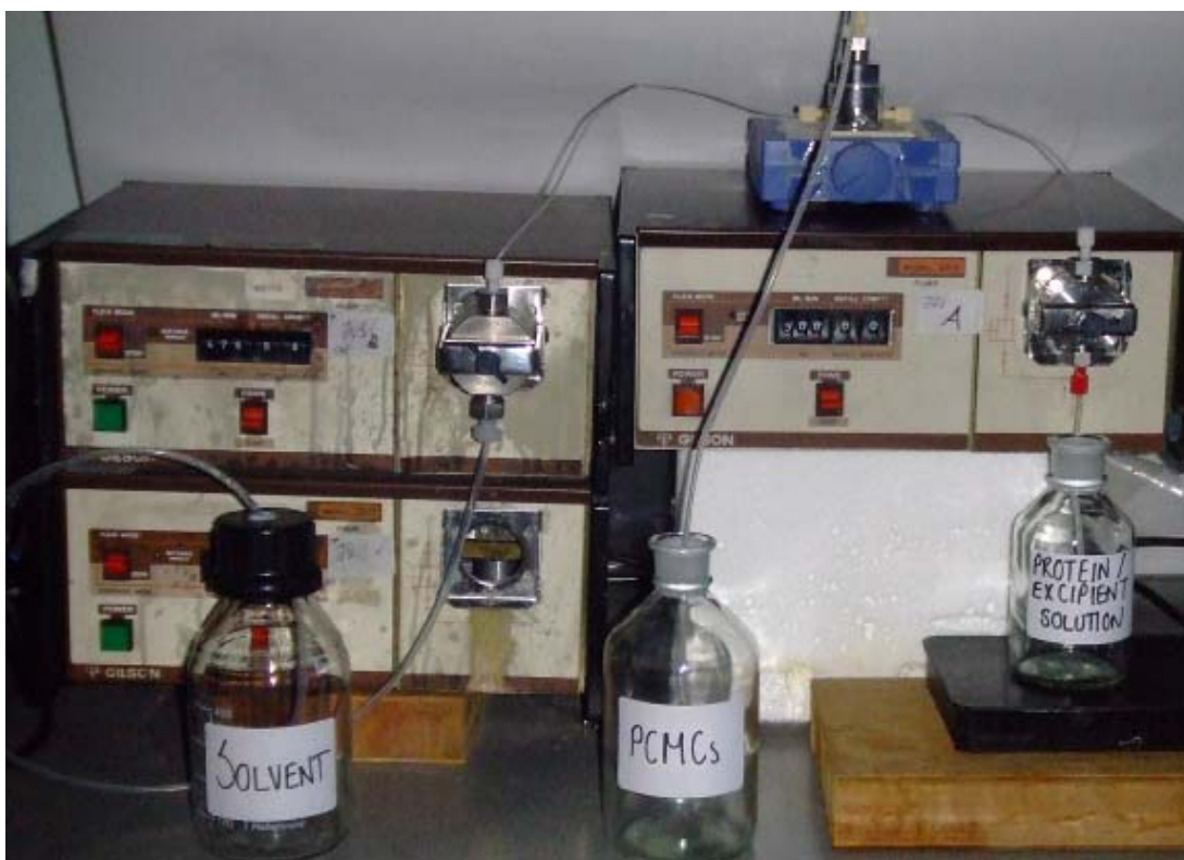
Figure 3.2: Photographic Representation of the Continuous-Flow Precipitator Used for the Preparation of PCMCs
