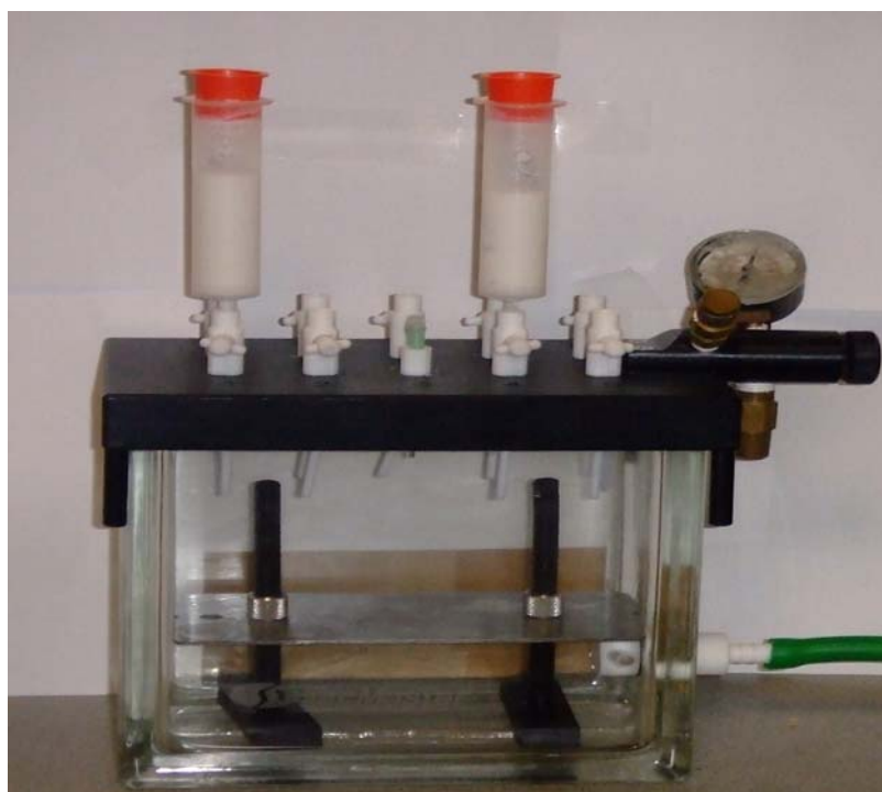
Figure 2.3: SPE Vacuum Manifold with Double-Fritted Filtration Columns for use in Molecularly Imprinted Solid-Phase Extraction
