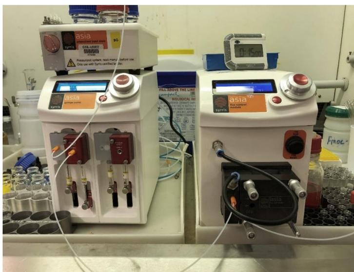
**Figure S4:** Syrris Asia pump and Syrris FLUX electrochemical module used for the adaption of the batch electrochemical reaction into flow.
