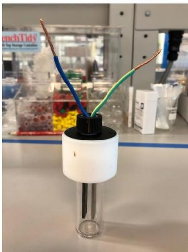
**Figure S6:** The complete vial used for experiments that involved the use of a voltmeter.
