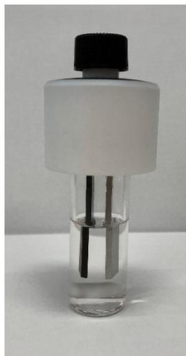
**Figure S2:** Complete electrochemical cell, ready to be subjected to electrolysis on ElectraSyn 2.0.
