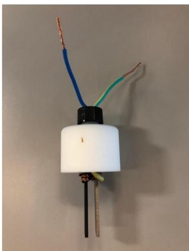
**Figure S5:** Wires for the voltmeter were wrapped around the anode and cathode and fed up through the lid of the ElectroSyn vial.
