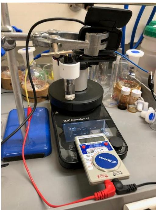
**Figure S8:** An alternative view of the experimental set up for recording the observed and actual potential difference of the electrochemical reaction.
