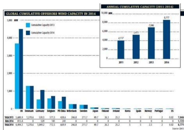
Figure 1.4 Annual and cumulative installations of offshore wind (MW) (Global Wind Energy Council, 2015)
