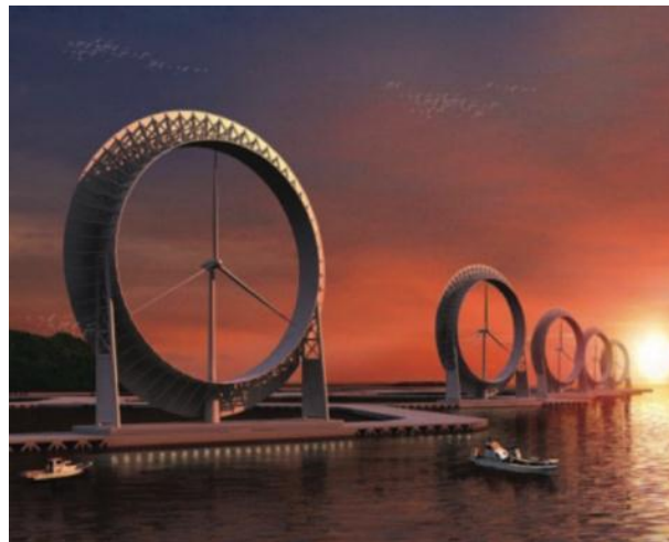
Figure 1.15 Prof Ohta's concept of pontoon-type wind turbine with rotor shroud nozzle (Wang, 2010)
