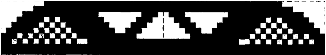
Figure 2.22: An example of checkerboarding, showing how a part with this structure has low stiffness, and is difficult to manufacture [52]
