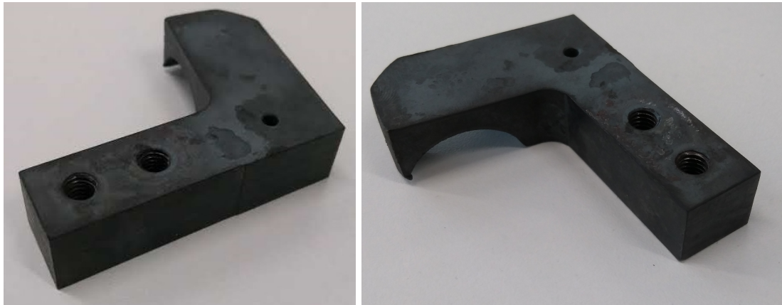
Figure 6.2: Gripper, as taken from hot forging cell robot arm
