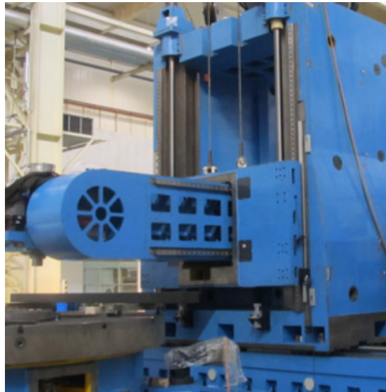
Figure 2.9: Finalised manipulator ram arm installed on friction stir welder [20]
