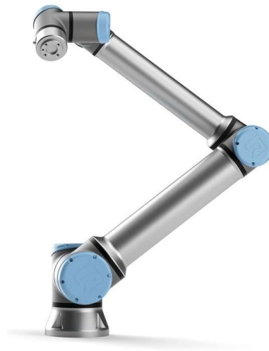
Figure 2.2: A modern robot, showing circular cross section links [10]
