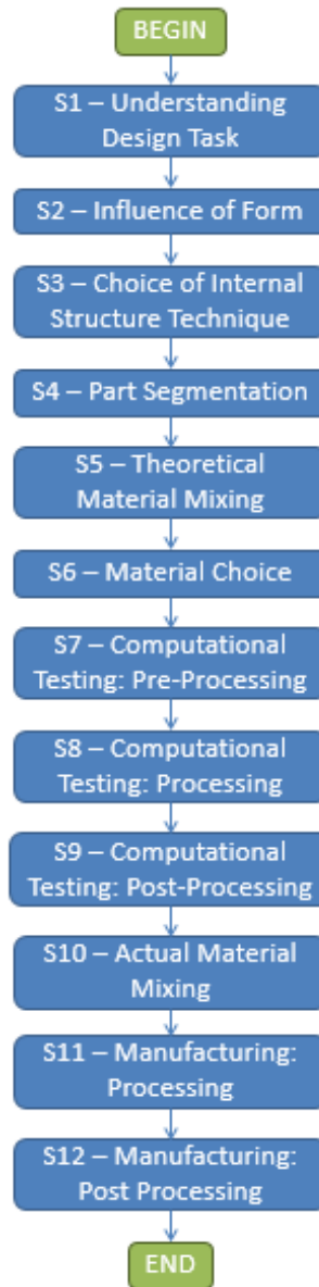
Figure 5.62: Diagram of complete design guidelines
