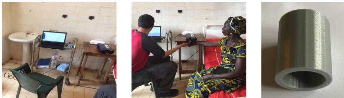
Figure 5.3 Photos of the instrumental set up (left), measurement set up (centre) and Raman adaptor (right) to keep measurement protected from the light and to keep a constant focal point.
