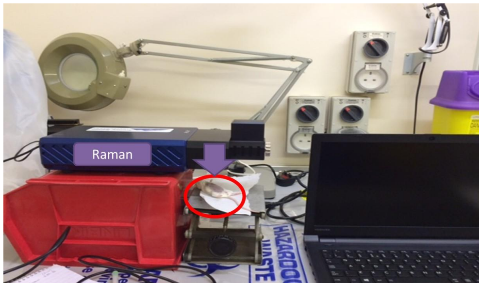
Figure 4.1 Illustration of the instrumental set-up of a benchtop Raman instrument for in situ mouse analysis.
