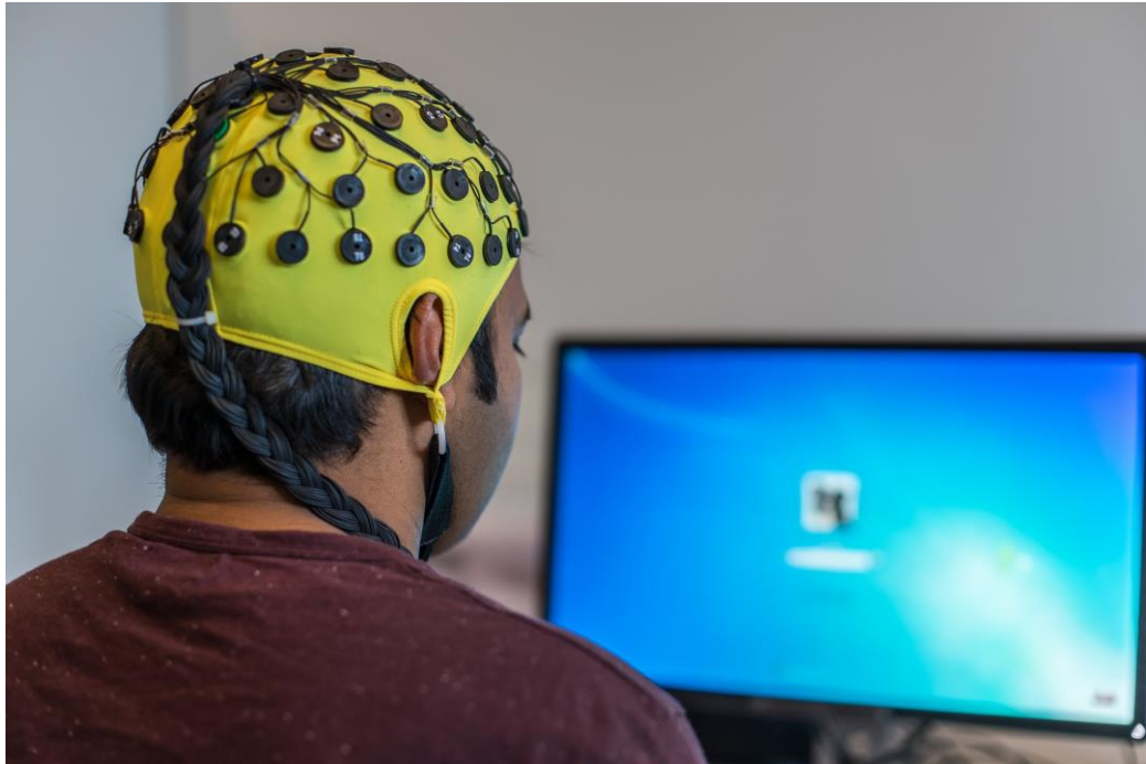
Figure 2.3: An EEG cap with electrodes being used in a typical BCI set-up.
