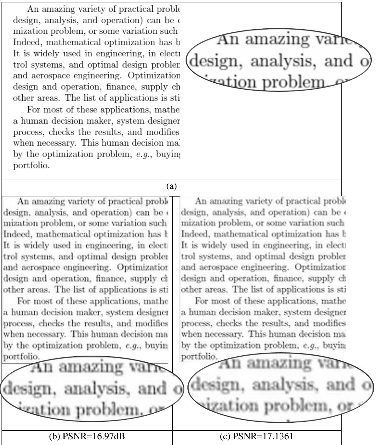
Figure 6-12: Super-resolution results for image ‘text’ and its PSNR (a) Original image (b) Method of (Zeyde et al., 2010)(c) The proposed method
