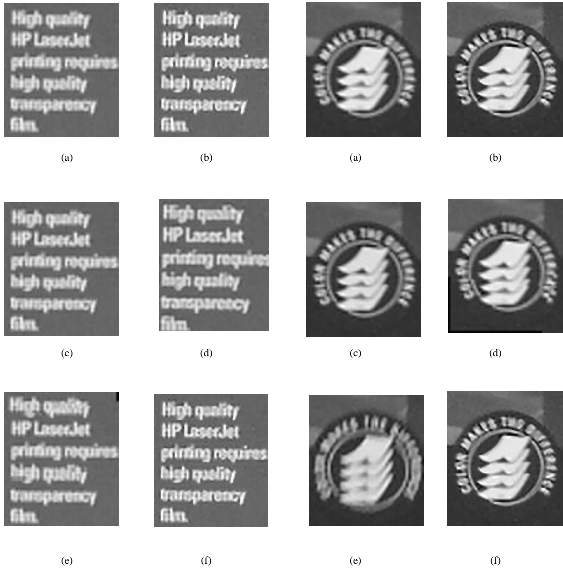
Figure 5-10: Super-resolution results with: (a) bicubic interpolation, (b) method of (Kim and Kwon, 2008), (c) the SIFT-BP-RANSAC registration method with bicubic interpolation, (d) the SIFT-BP-RANSAC registration method with the method of (Kim and Kwon, 2008) without fusion (e) Method of (Zomet et al., 2001), (f) the proposed super-resolution method with the method of (Kim and Kwon, 2008)
