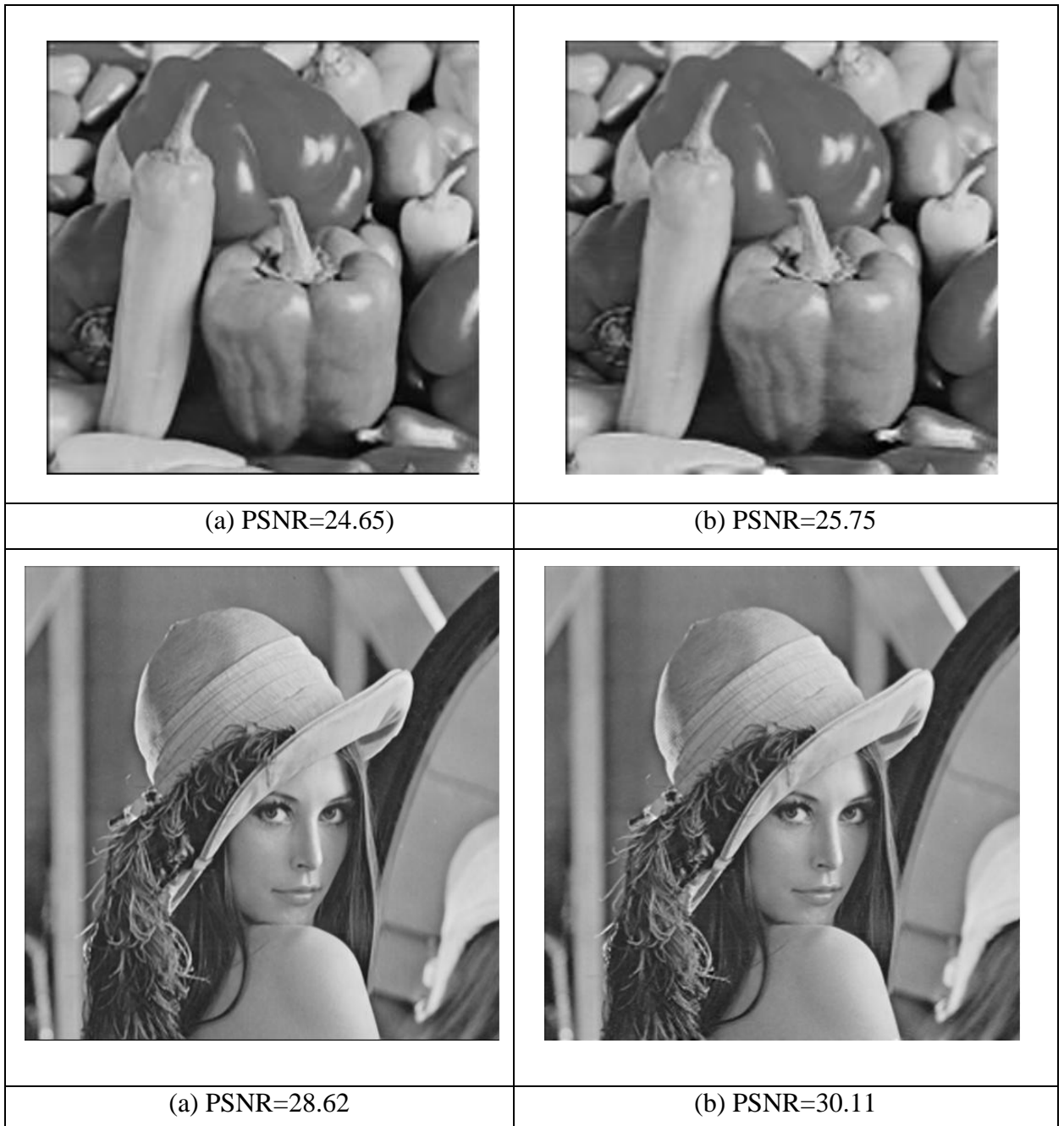
Figure 6-13: Super-resolution results and its PSNR: (top) ‘peppers’ (bottom) ‘lena’ (a) Method of (Zeyde et al., 2010) (b) The proposed method
