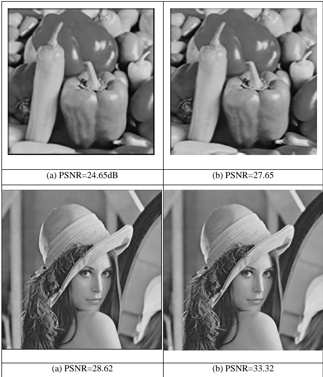
Figure 6-9: Super-resolution results and its PSNR: (top) ‘peppers’ (bottom) ‘lena’ (a) Method of (Zeyde et al., 2010) (b) The proposed method
