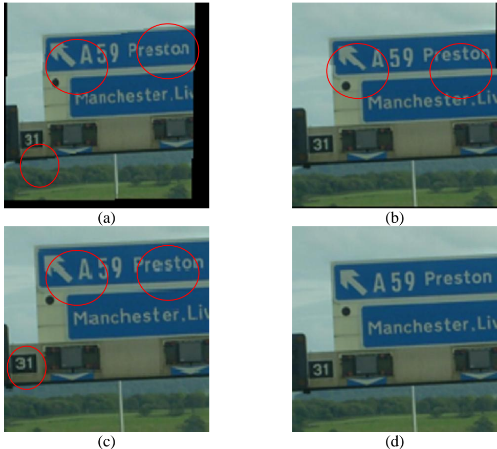
Figure 4-17: Super resolution results with (a) SIFT (b) SIFT-RANSAC (c) SIFT-BP (d) the proposed method
