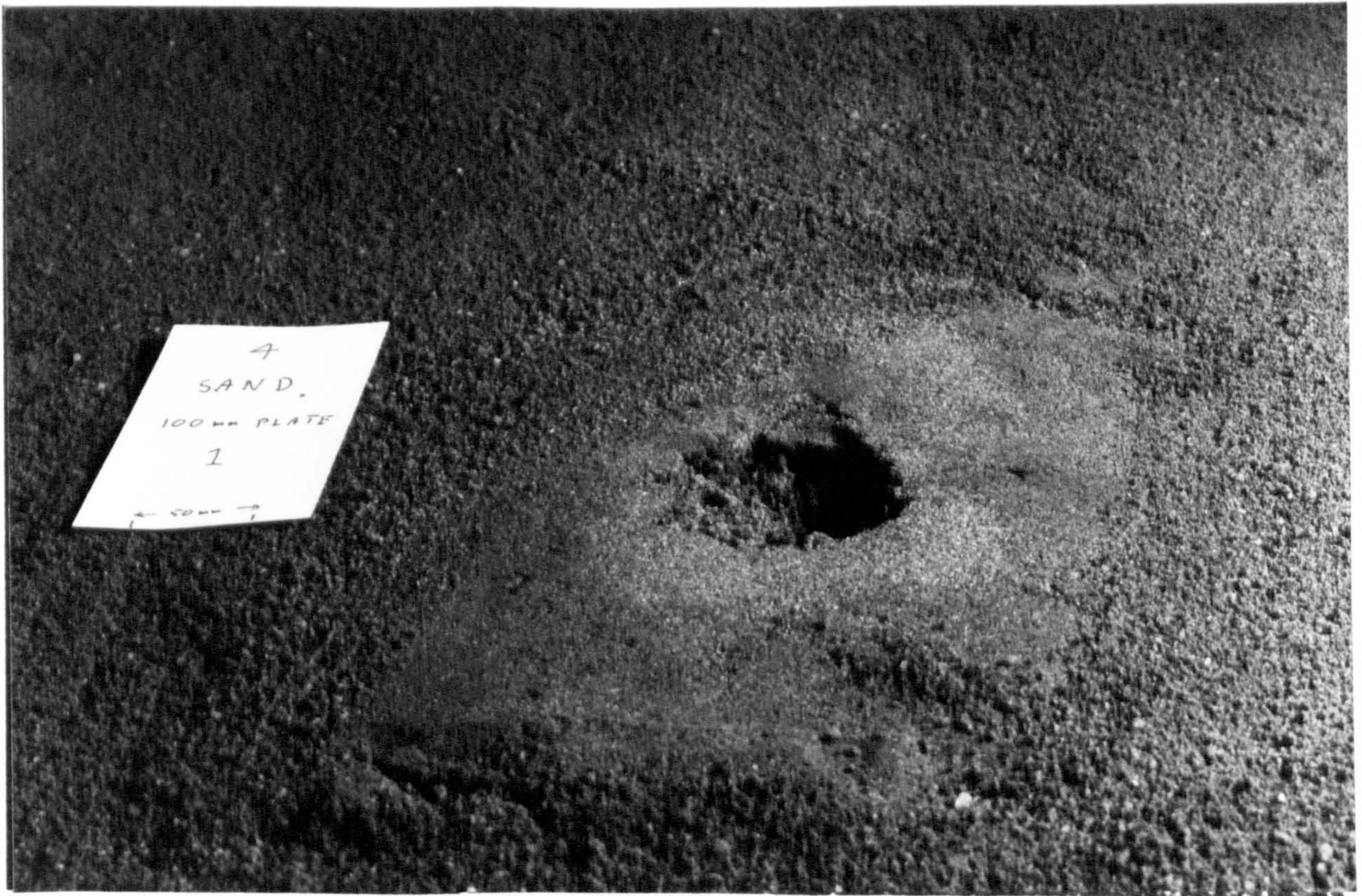
PLATE E.7 100 mm Diameter Hole After Plate-Load Bearing Tests of Sand
