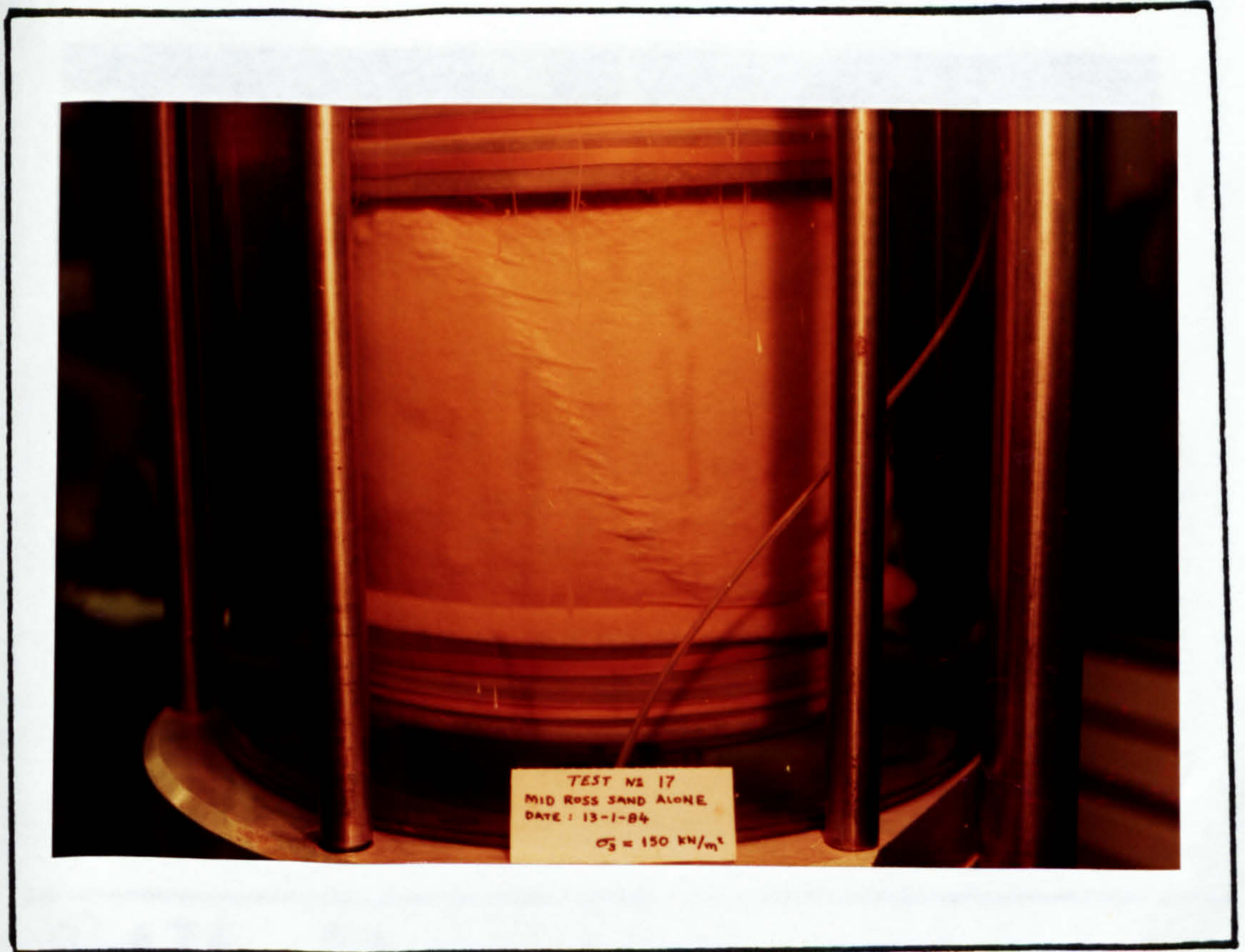
PLATE 21 The Deformed Triaxial Sample at Large Strains Consisting of Soil Alone
