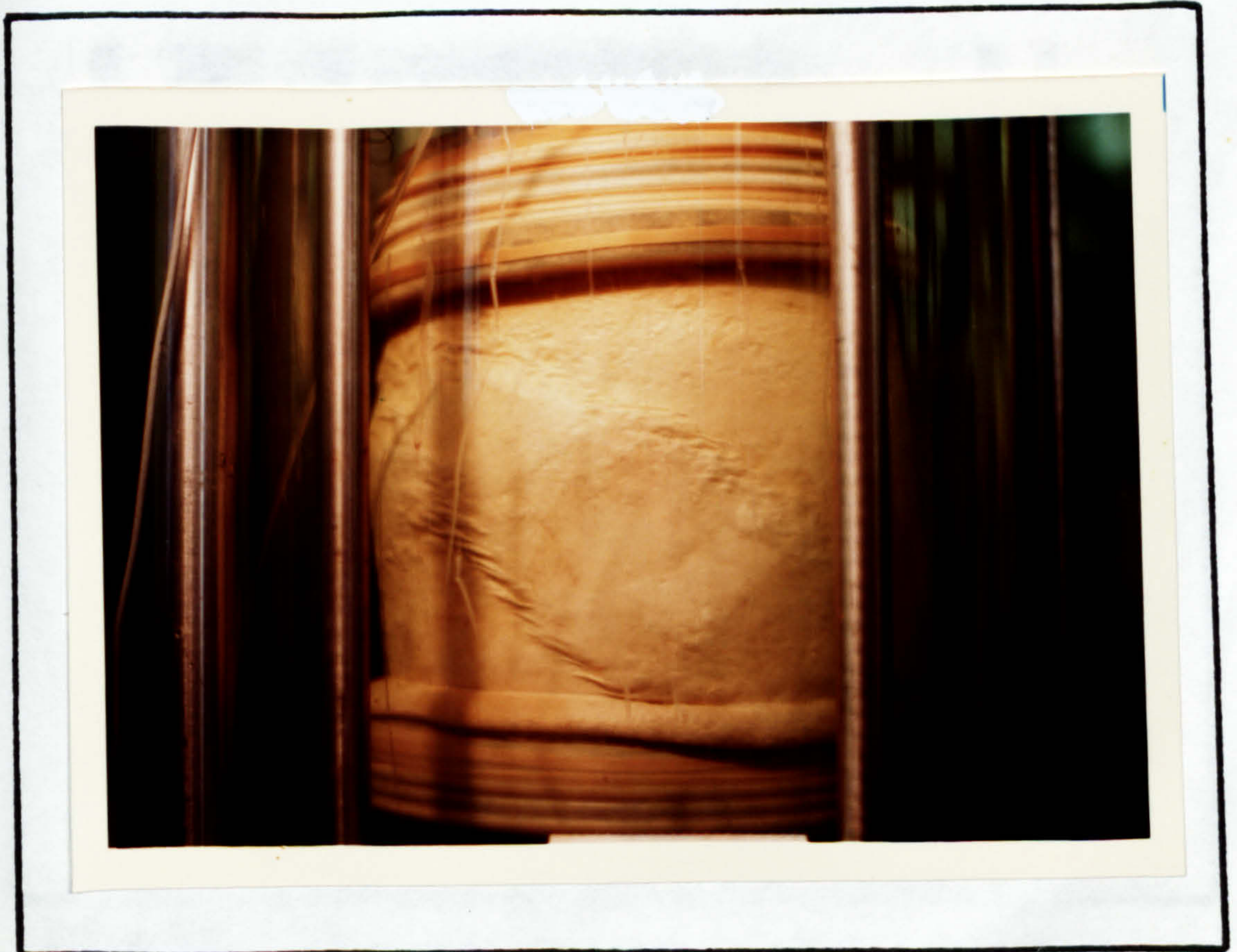
PLATE 22 The Deformed Triaxial Sample at Large Strains Consisting of Soil Mixed With Mesh Elements
