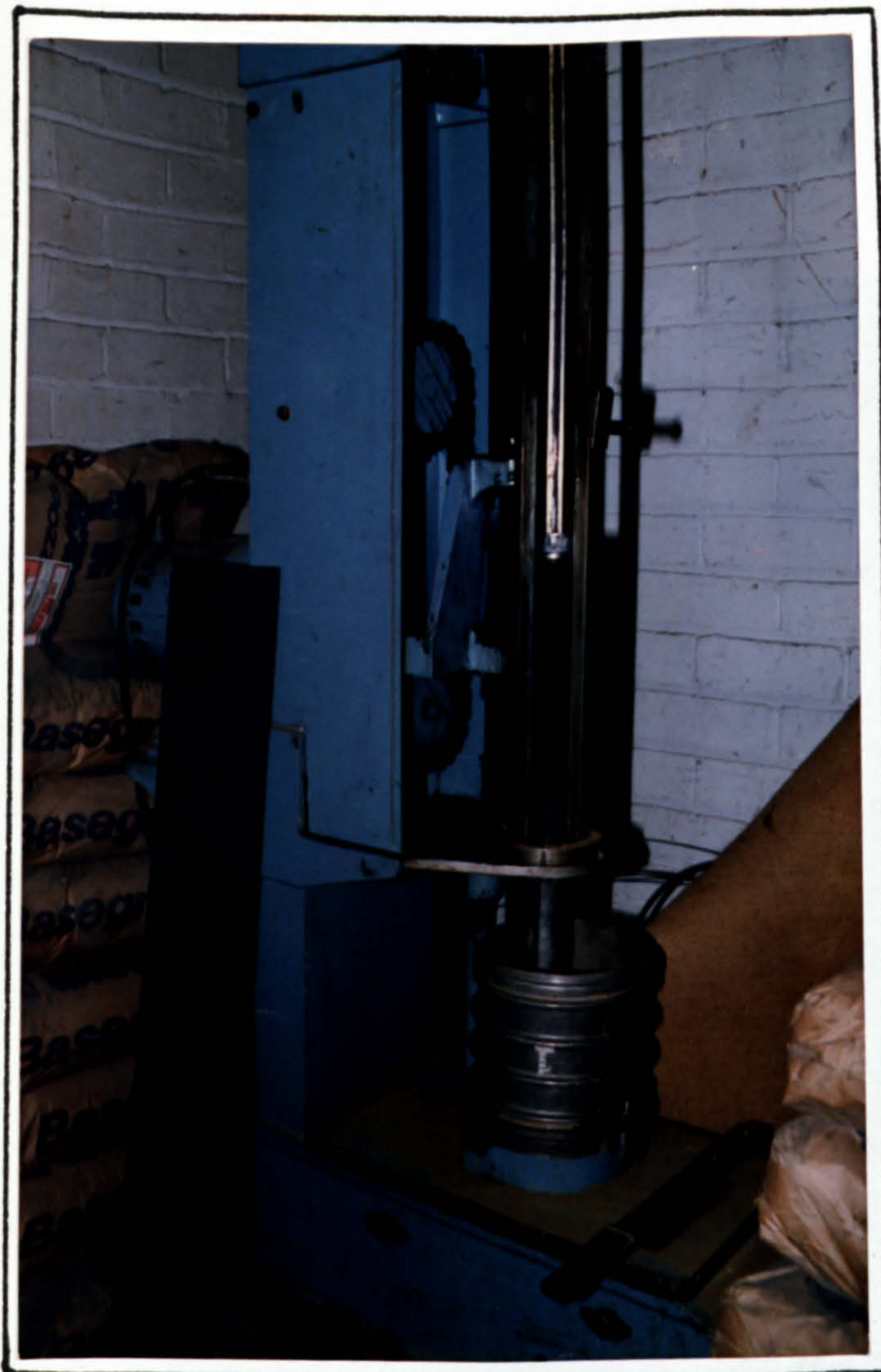
PLATE 3 The automatic Compaction machine
