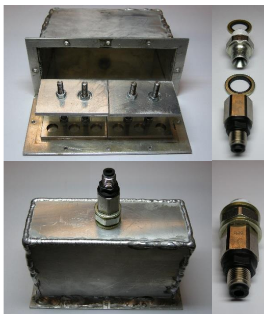
Figure 5.14: Metal frame and chamber with the gas connection.
