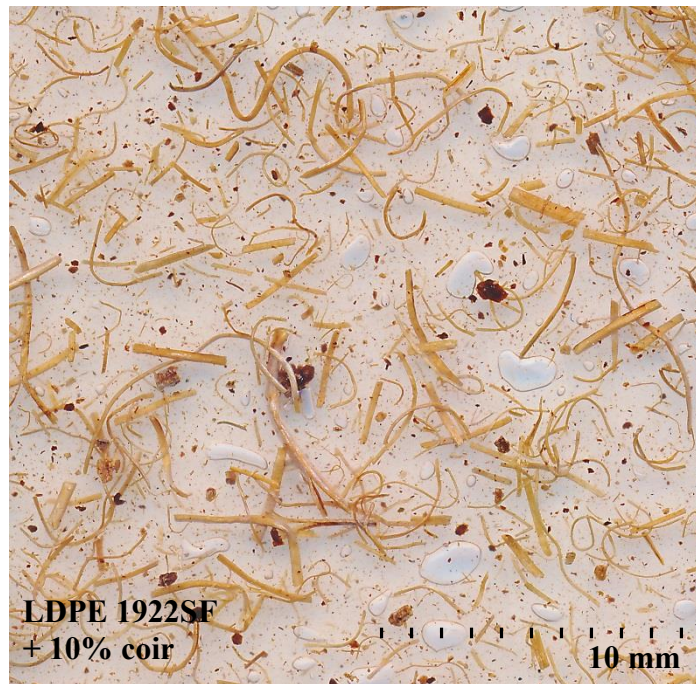
Figure 6.8: Scanned image of a LDPE 1922SF + 10% coir film.
