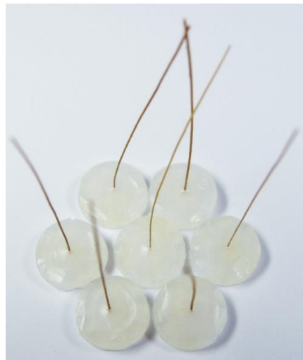
Figure 5.17: PP579S cylindrical pull-out samples.
