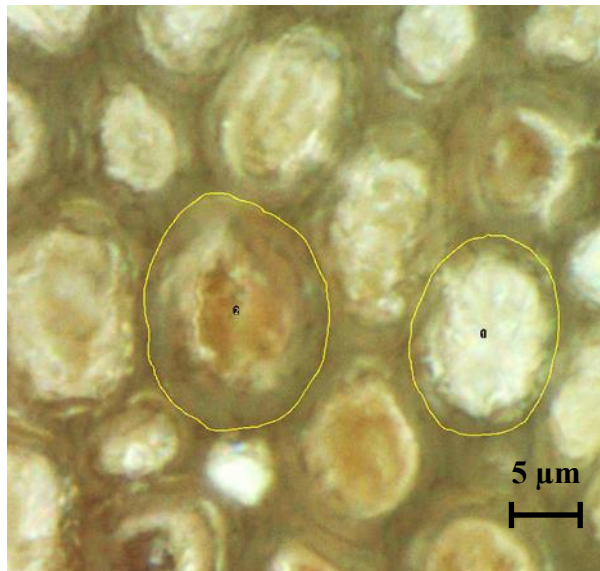
Figure 2.15: Detail of the CSA of palm fibre. Measurement of elementary fibres.
