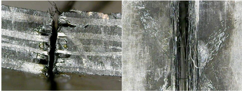
Figure 113: Microscope images of edge side (left) and top side (right) of laser cutting test 63.
