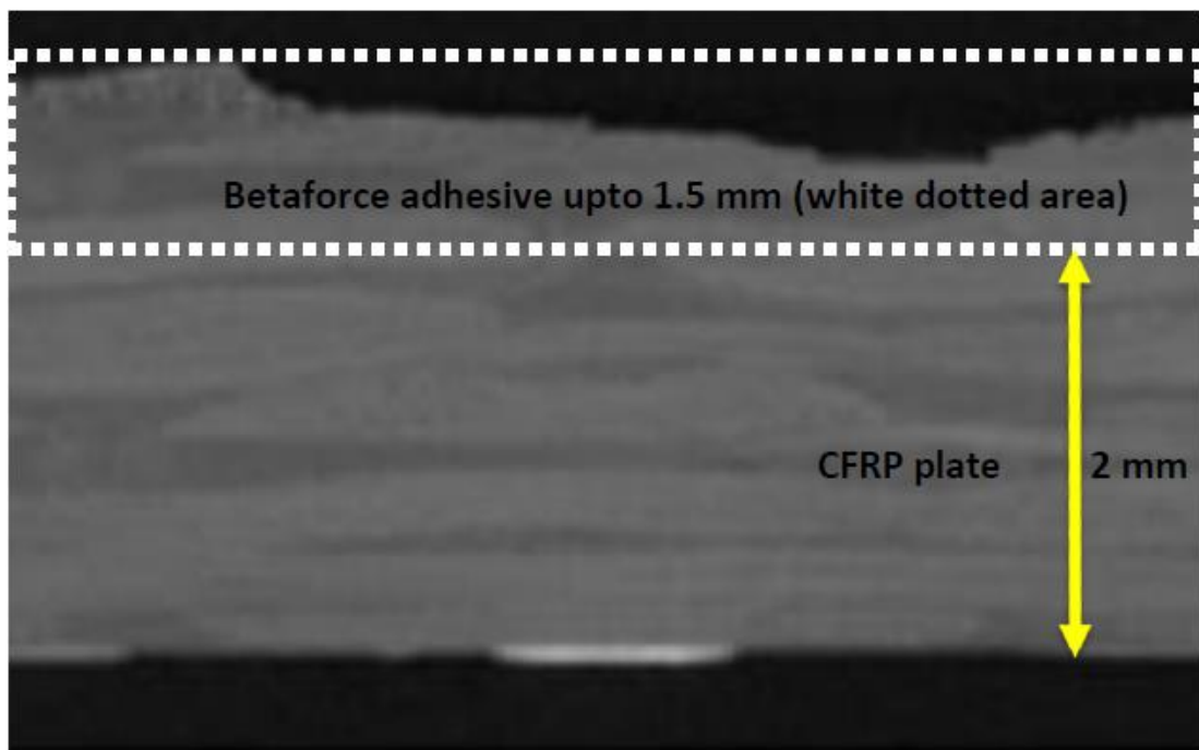
Figure 160: Slice of 3D XCT scan of PU adhesive glue on CFRP sample.
