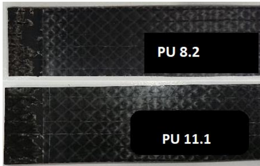
Figure 135: CFRP samples 8.2 (top) and 11.1 (bottom) after laser cleaning of PU adhesive.
