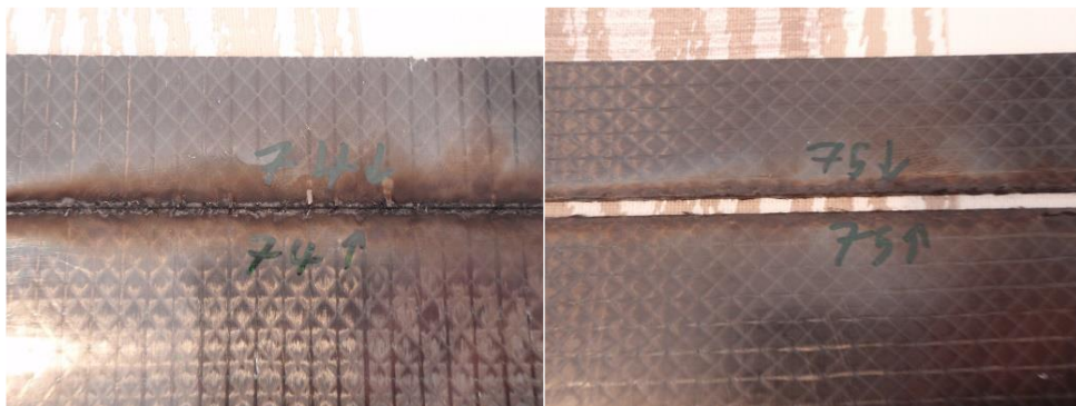
Figure 95: Images of top side laser cut surfaces of tests 74 (left) and 75 (right).
