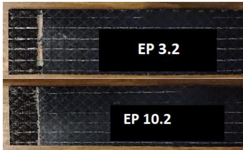
Figure 136: CFRP samples 3.2 (top) and 10.2 (bottom) after laser cleaning of EP adhesive.
