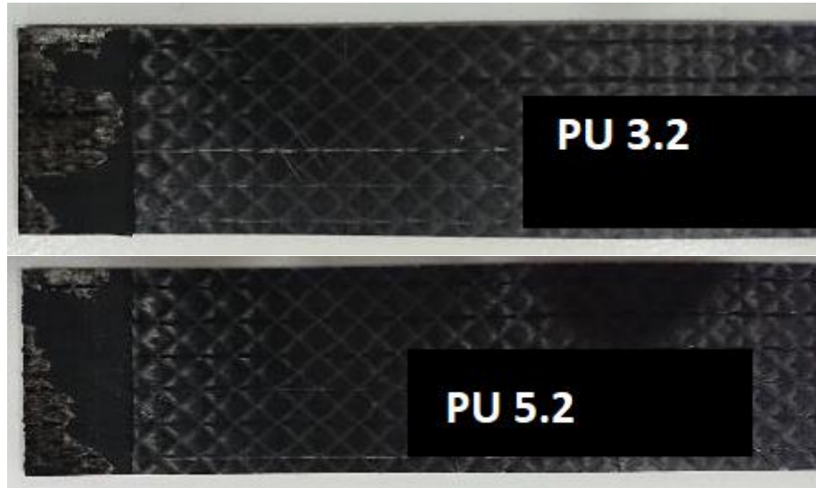
Figure 134: CFRP samples 3.2 (top) and 5.2 (bottom) after laser cleaning of PU adhesive.
