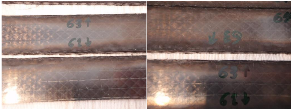
Figure 89: Images of top side laser cut surfaces of tests 62 (left) and 63 (right).
