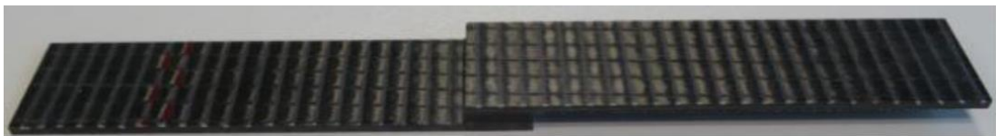
Figure 146: CFRP-CFRP sample bonded using PU adhesive.
