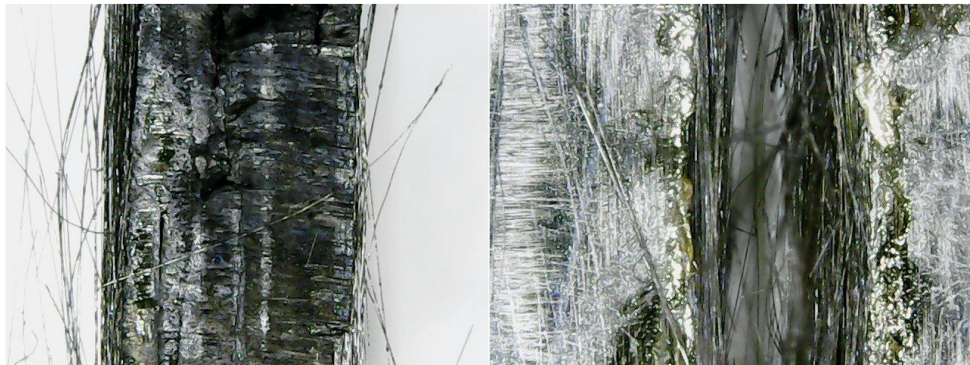
Figure 109: Microscope images of edge side (left) and top side (right) of laser cutting test 59.
