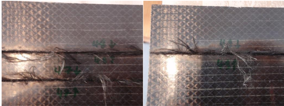
Figure 82: images of top side laser cut surface of tests 48 (left) and 49 (right).
