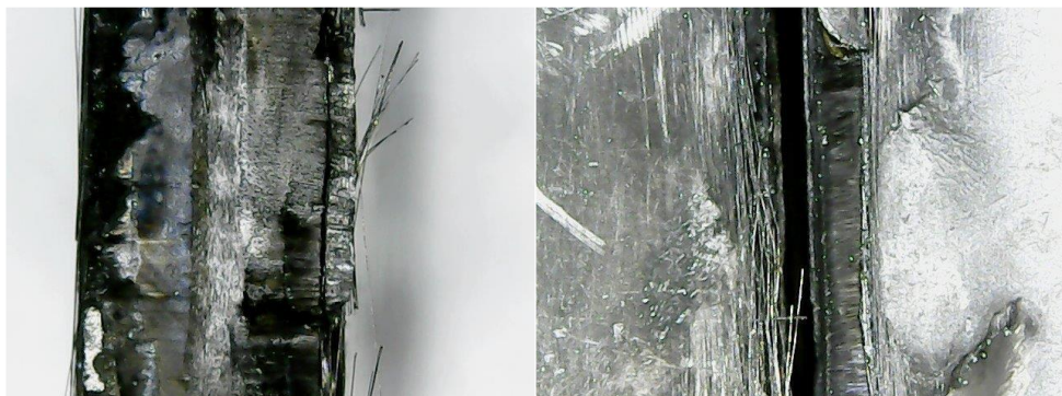
Figure 118: Microscope images of edge side (left) and top side (right) of laser cutting test 68.
