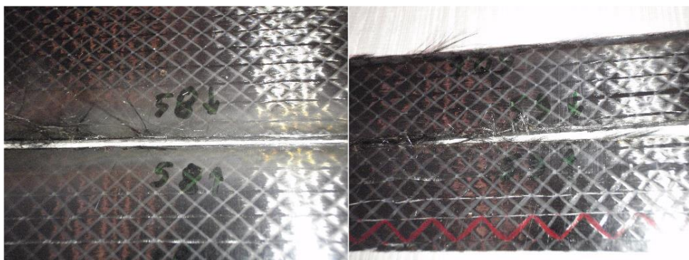
Figure 87: Images of top side laser cut surfaces of tests 58 (left) and 59 (right).
