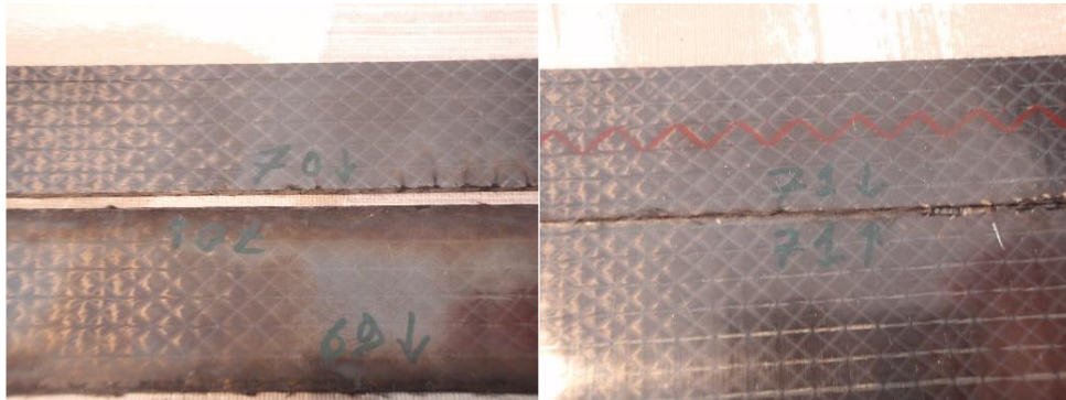
Figure 93: Images of top side laser cut surfaces of tests 70 (left) and 71 (right).
