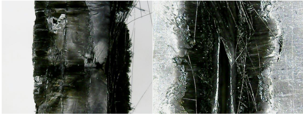
Figure 101: Microscope images of edge side (left) and top side (right) of laser cutting test 51.
