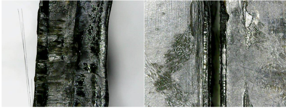
Figure 115: Microscope images of edge side (left) and top side (right) of laser cutting test 65.
