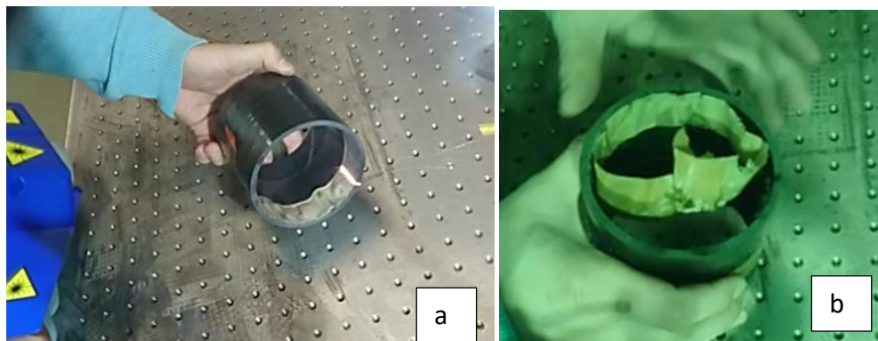
Figure 75: (a) Handheld laser detachment of EP adhesive, (b) EP adhesive peeled from the cylinder surface.
