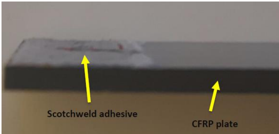
Figure 161: Image of EP adhesive on CFRP sample.
