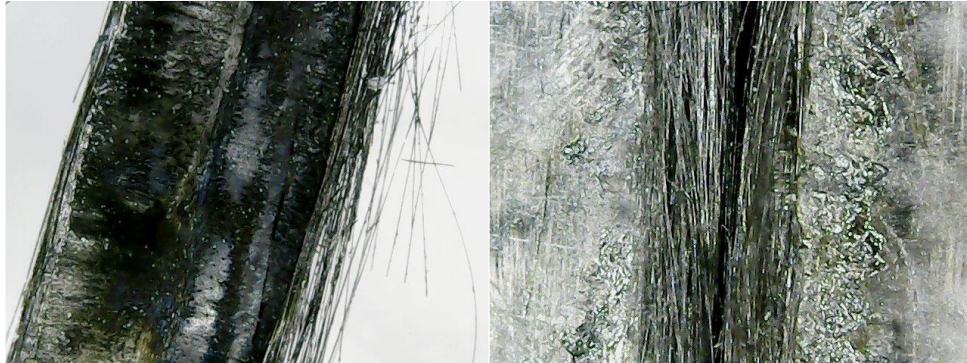
Figure 96: Microscope images of edge side (left) and top side (right) of laser cutting test 46b.
