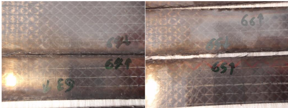
Figure 90: Images of top side laser cut surfaces of tests 64 (left) and 65 (right).
