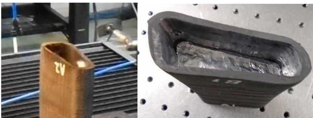
Figure 74: Sustained flame inside the insert, fuelled by the existence of the filler foam material (left), Aluminium foil placed inside the shaped insert to cover the flammable material form laser irradiation (right)
