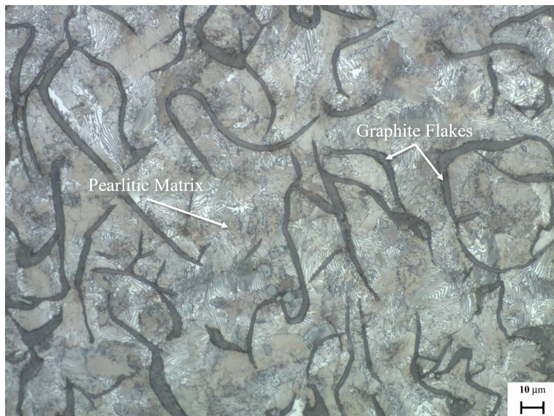
Figure 3.1 - Microstructure of G350 grey cast iron [x500 – etched].
