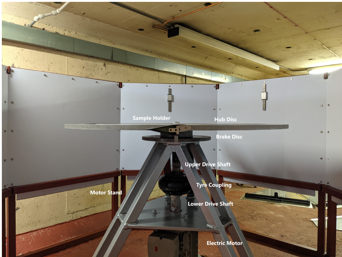
Figure 6.21: Displayed here are the Motor Stand, the Hub Disc, the Aerofoil Sample Holders, the Brake Disc, the Upper Drive Shaft, the Tyre Coupling, the Lower Drive Shaft and the Electric Motor, correctly assembled and configured.
