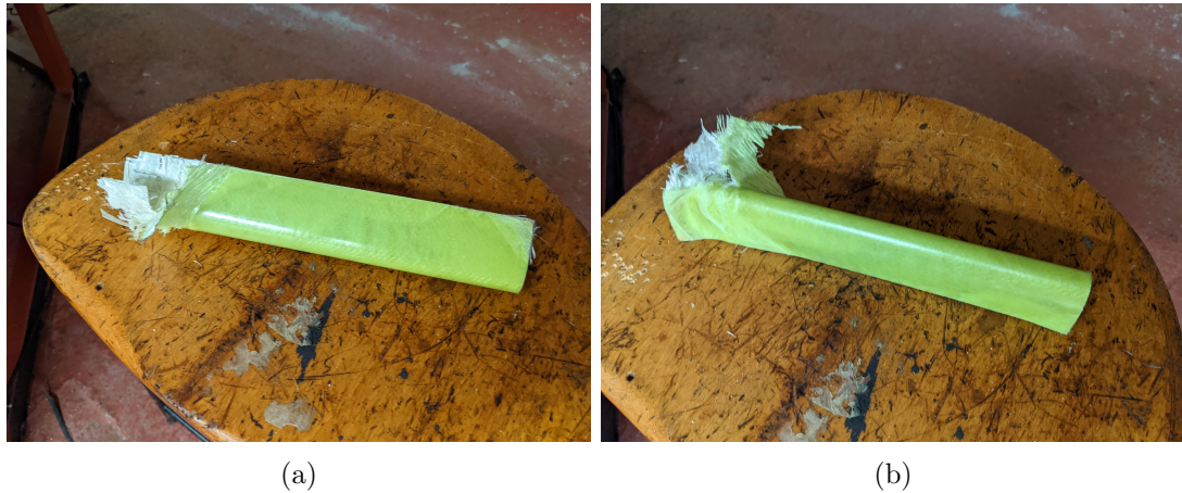
Figure 6.40: Figures 6.40a and 6.40b show the impact damage to S1.
