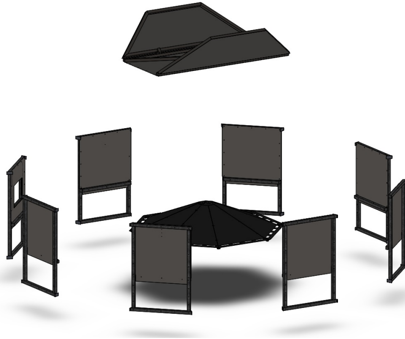
Figure 6.15: Displayed here is the Full Enclosure, including the coned drainage system and lid, however in this diagram the door was omitted.
