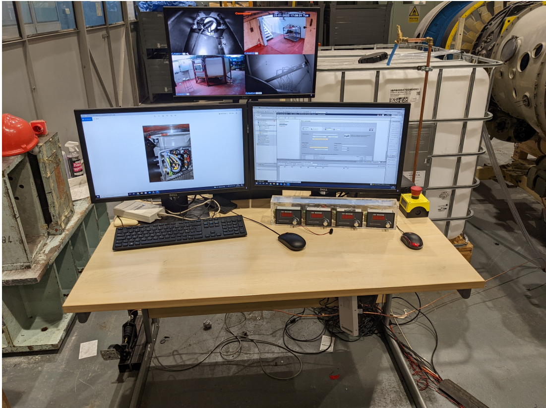
Figure 6.27: Displayed here is the control station. The red emergency power button can be seen on the right, the foot brake situated underneath the desk on the left, the CCTV screen above the central two computer monitors used to operate and monitor the rig and the peristaltic pump control units below the screen on the right-hand side.
