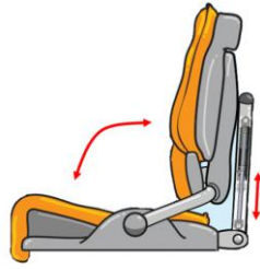
Figure 0.1 Dynamic backrest: the gas spring put inside the back tube
