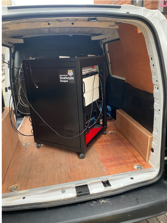
Figure 4.11: An image of the system in the back of a van on the day of the field trials. The system is powered by the car battery. The laser was found to on the day unlock consistently, resulting in only brief periods of cold atoms being achieved during the trials..
