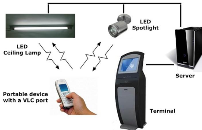
FIGURE 5.15: Illustration of an envisaged visible light communications network, from [31].
