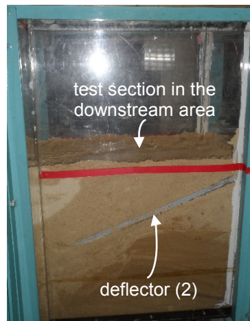
Figure 5.72: Deflector (2) with a slope of 1/2.50 installed within the downstream test section.
