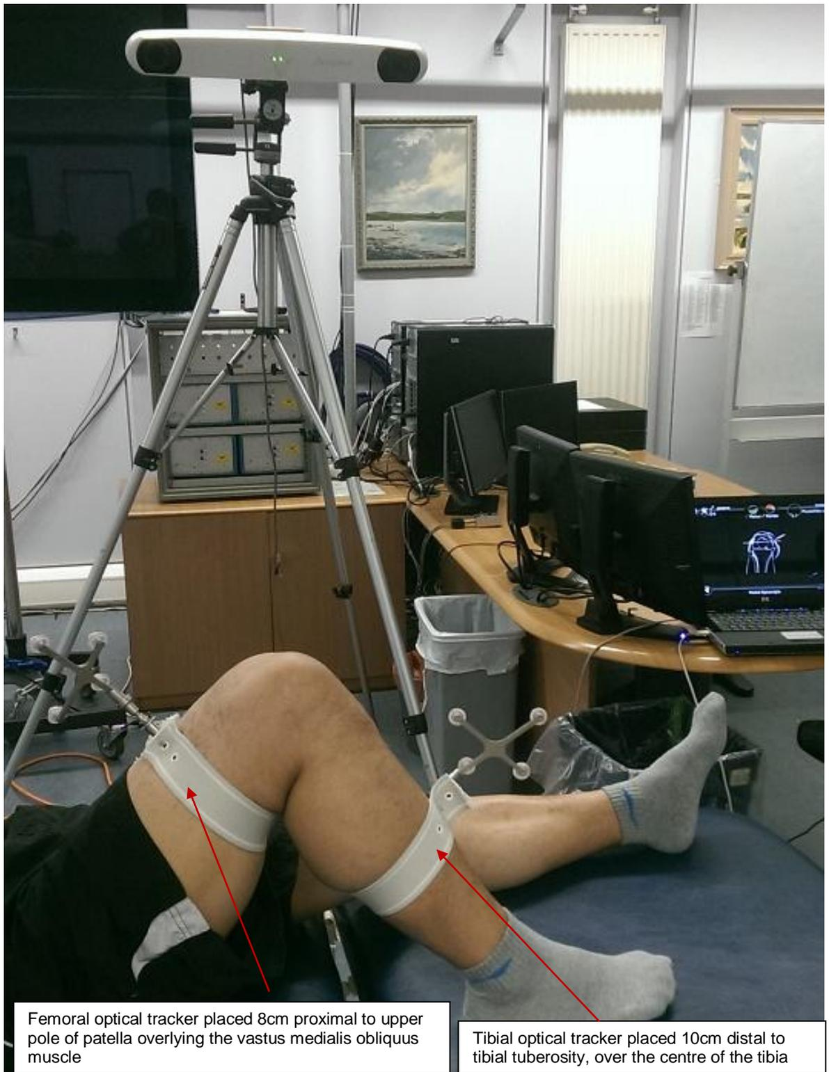
**Figure 5.2** An example of the set-up of each volunteer assessment; with the volunteer relaxed whilst lying supine in short trousers. Passive optical trackers mounted on the femur and tibia using fabric straps to secure the base plate holding the optical tracker in place, with the laptop visible for the Examiner to perform volunteer testing
