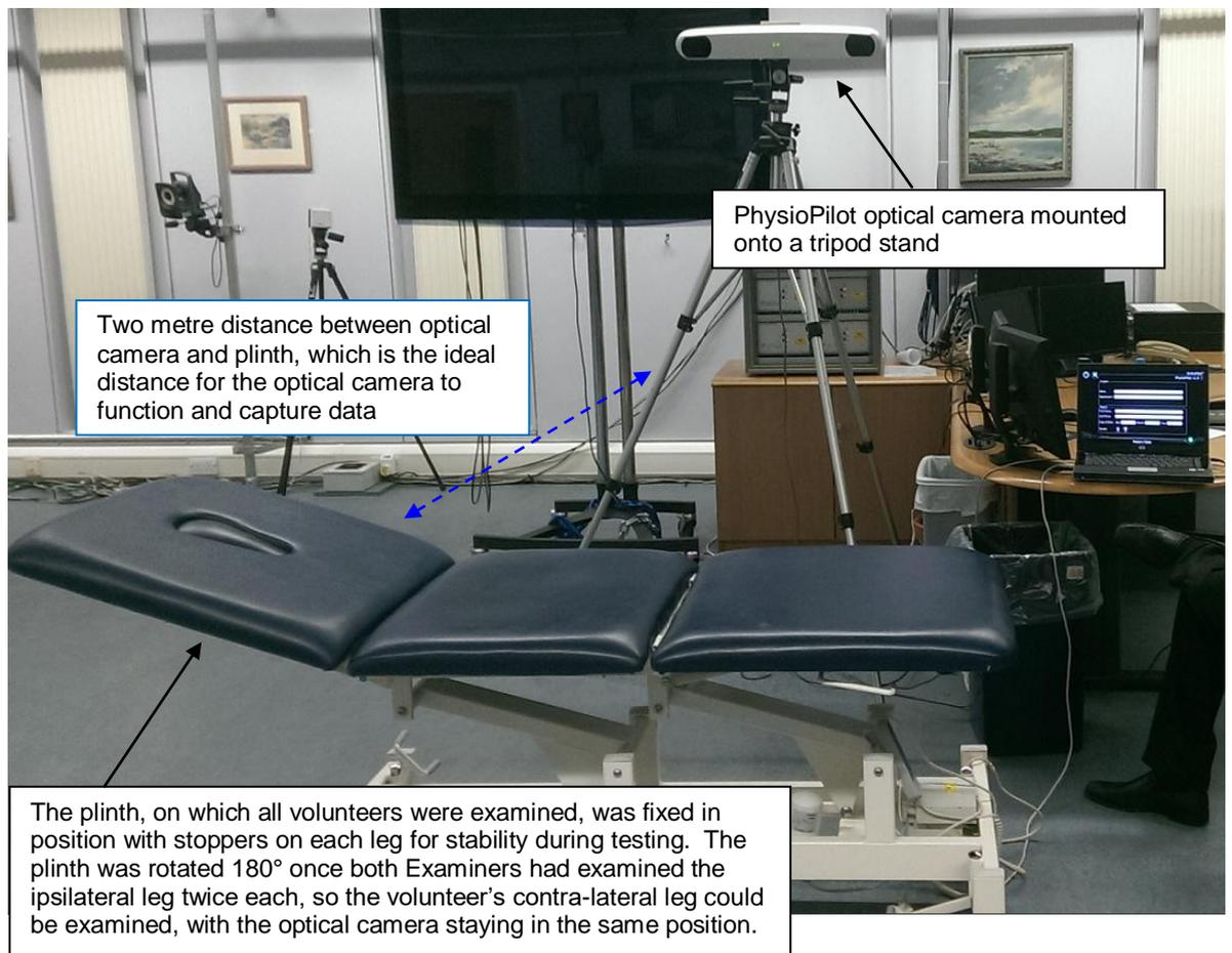
**Figure 5.1** Image depicting the layout of the PhysioPilot optical camera, positioned two metres away from the plinth, with a laptop connected to the optical camera
