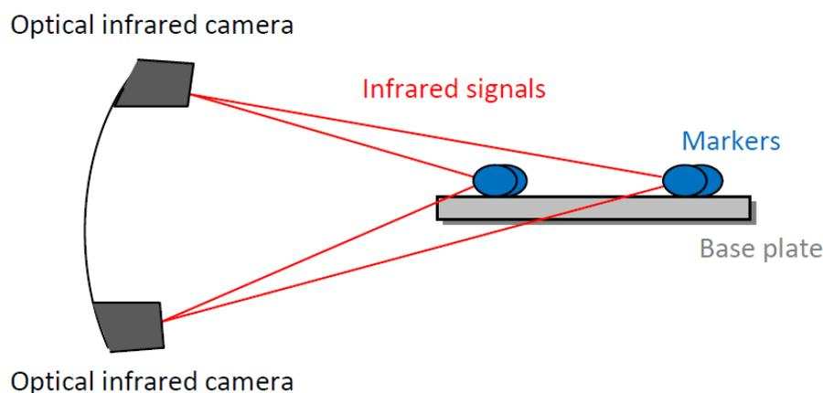
**Figure 7.1** Image depicts optical camera sending infrared signals which only detect 2 of the new optical tracker markers, due to the markers mounting positioning flat on the base plate.
