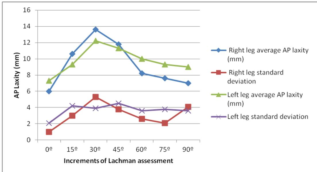
**Graph 3** Demonstrating pattern of AP laxity from 0° to 90° using new optical tracker set
