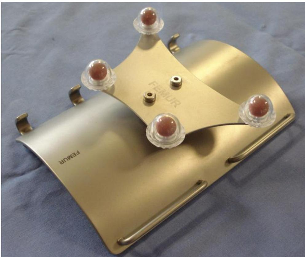
**Figure 3.4** The femoral new optical tracker with the surface metal plate containing four optical markers mounted on top of a curved metal base plate, with metal attachments for where the fabric straps were incorporated
