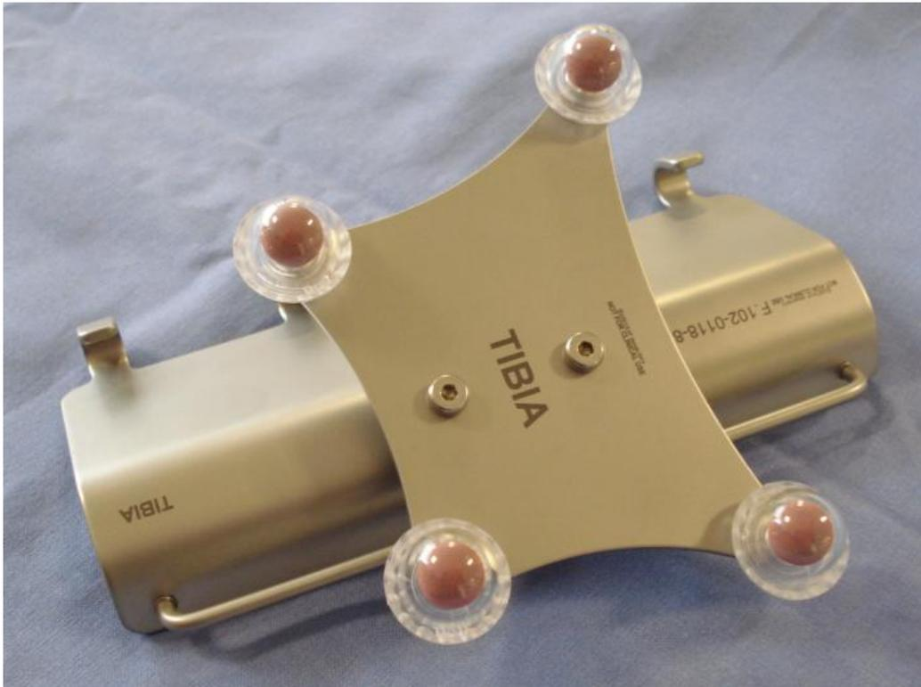
**Figure 3.5** Tibial new optical tracker, with surface plate and mounted markers and curved metal base plate which was designed to fit around the tibia
