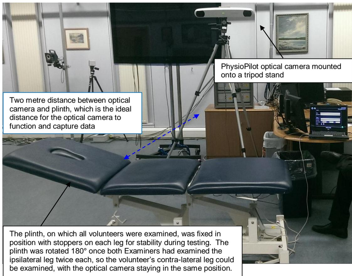
**Figure A** Image depicting the layout of the PhysioPilot optical camera, positioned two metres away from the plinth, with a laptop connected to the optical camera
