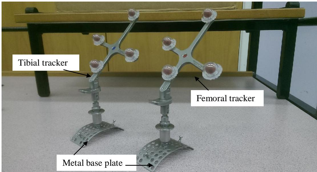
**Figure 3.1** This images shows the pre-validated set of optical trackers mounted on their metal base plates (femoral tracker has a red dot and the tibial tracker a blue dot in the centre of trackers)
