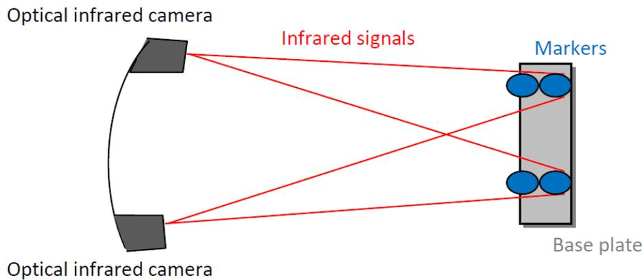
**Figure 7.2** Image depicts optical camera sending infrared signals which detect all 4 of the pre-validated optical tracker markers, due to the markers mounting positioning at 60° on the base plate.
