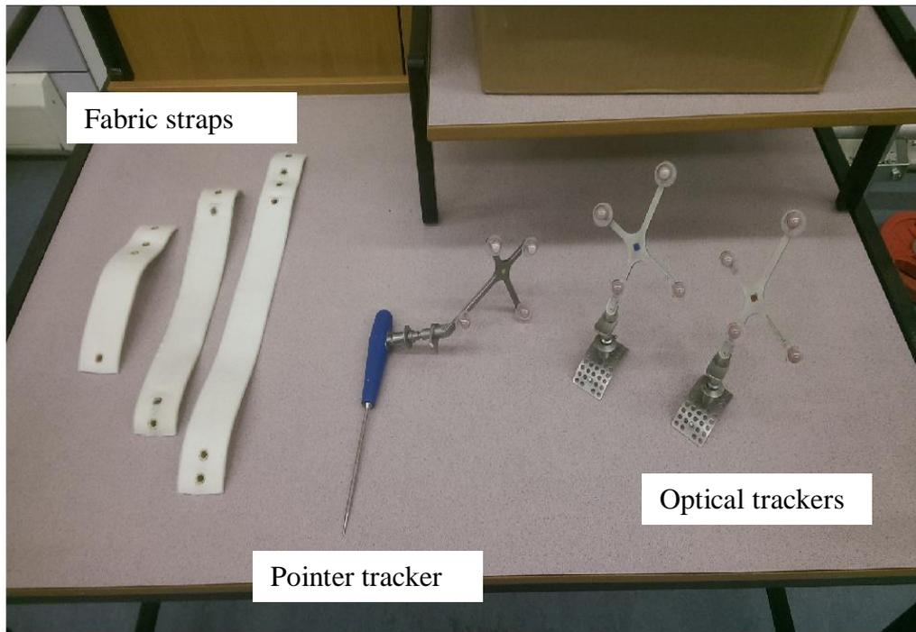
**Figure 3.3** Image showing the pre-validated set of optical trackers mounted on metal base plates, pointer tracker and fabric straps with rivets at the ends of the straps to mount the base plates to the examined legs.
