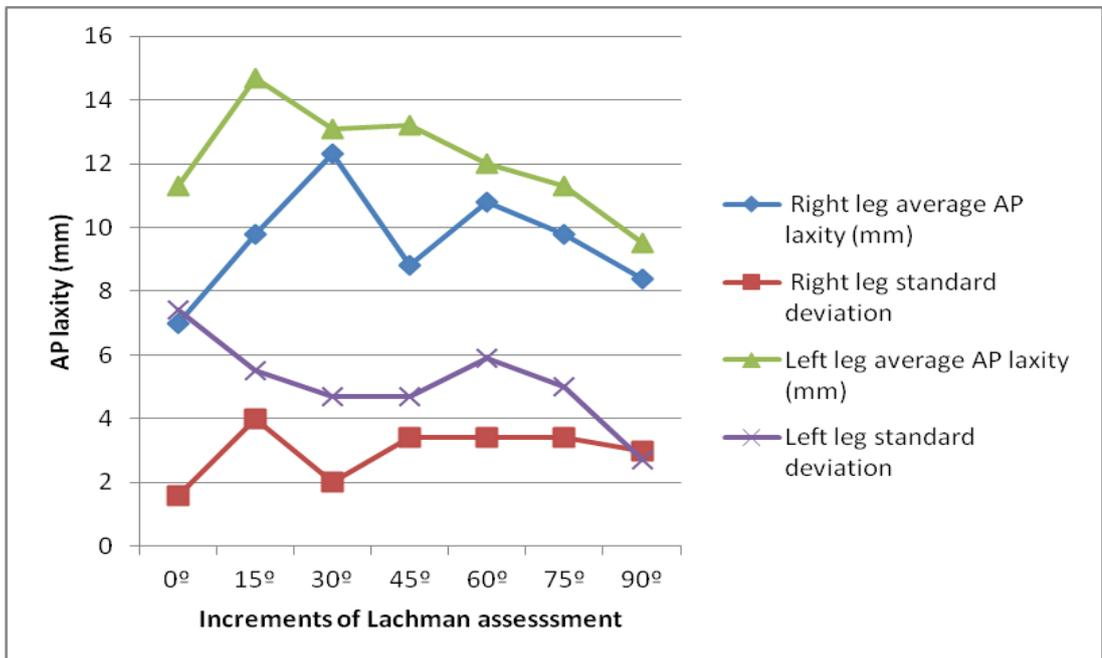
**Graph 7** Demonstrating pattern of AP laxity from 0° to 90° using new optical tracker set
