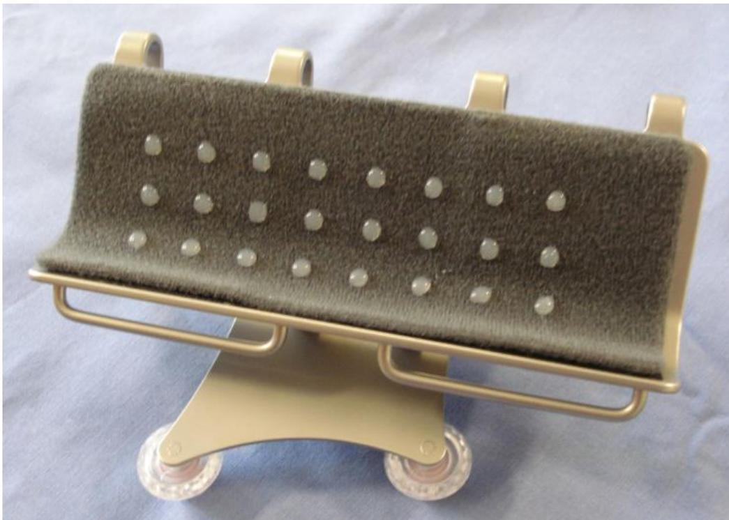
**Figure 3.6** The padding present under the curved metal base plate of the tibial tracker which was also present on femoral new optical tracker
