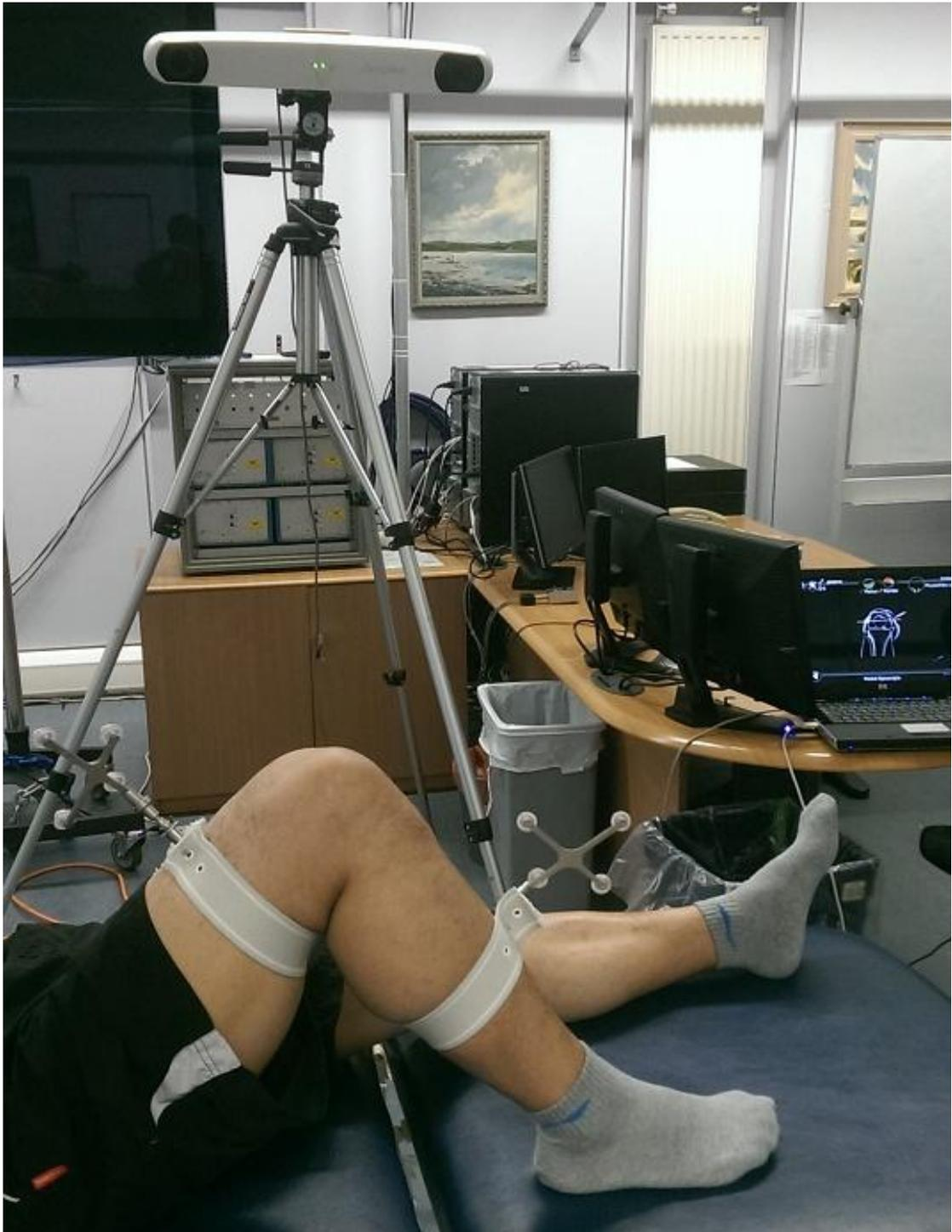
**Figure 3.2** Depicts an example of the set-up of each volunteer assessment. The pre-validated passive optical trackers are mounted on the femur and tibia using fabric straps to secure the base plate holding the optical tracker in place
