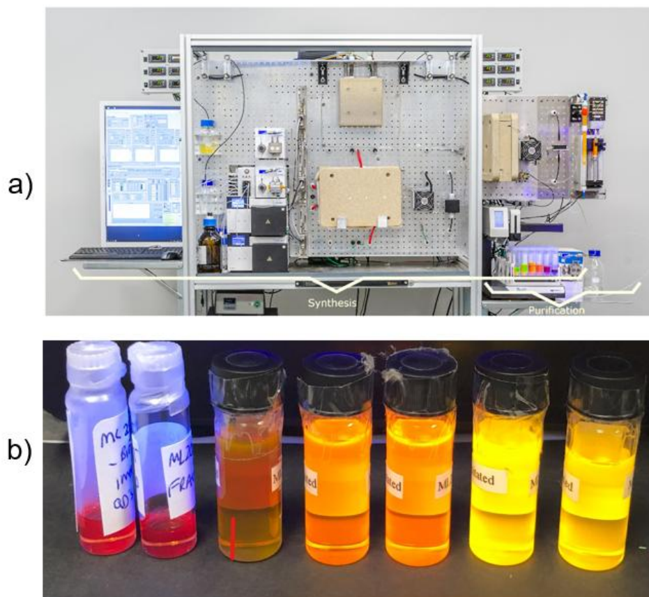
Fig. 2-10 a) Image of continuous synthesis reactor as seen in [43] from project collaborator, Fraunhofer IMM., reproduced under CC BY 4.0. b) quantum dots made using continuous synthesis from Fraunhofer IMM collaborator excited under ultraviolet light
