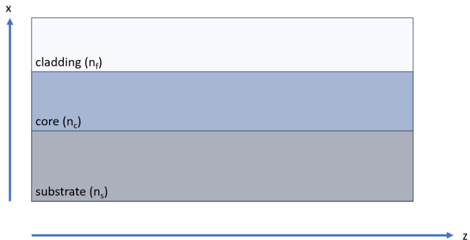
Fig. 2-12 schematic of planar dielectric waveguide, with the core surrounded by two other refractive index materials known as the core and cladding.
