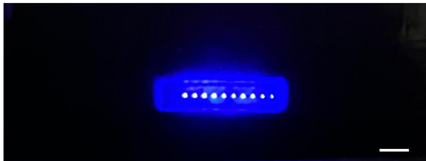
Fig. 3-4 Image of GaN \mu LED showing 1 x 10 pixel array design. Scale bar show is 2 mm.
