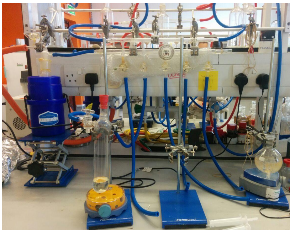
Figure 7.1. A typical laboratory Schlenk line in use.
