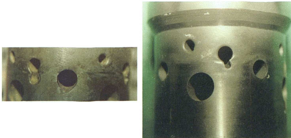
Figure 1.4 Typical erosion scars on a flow control tip.
