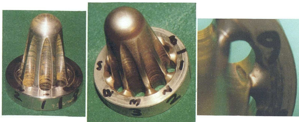
Figure 6.14 Erosion of fluted restrictor: AISI 4130.
