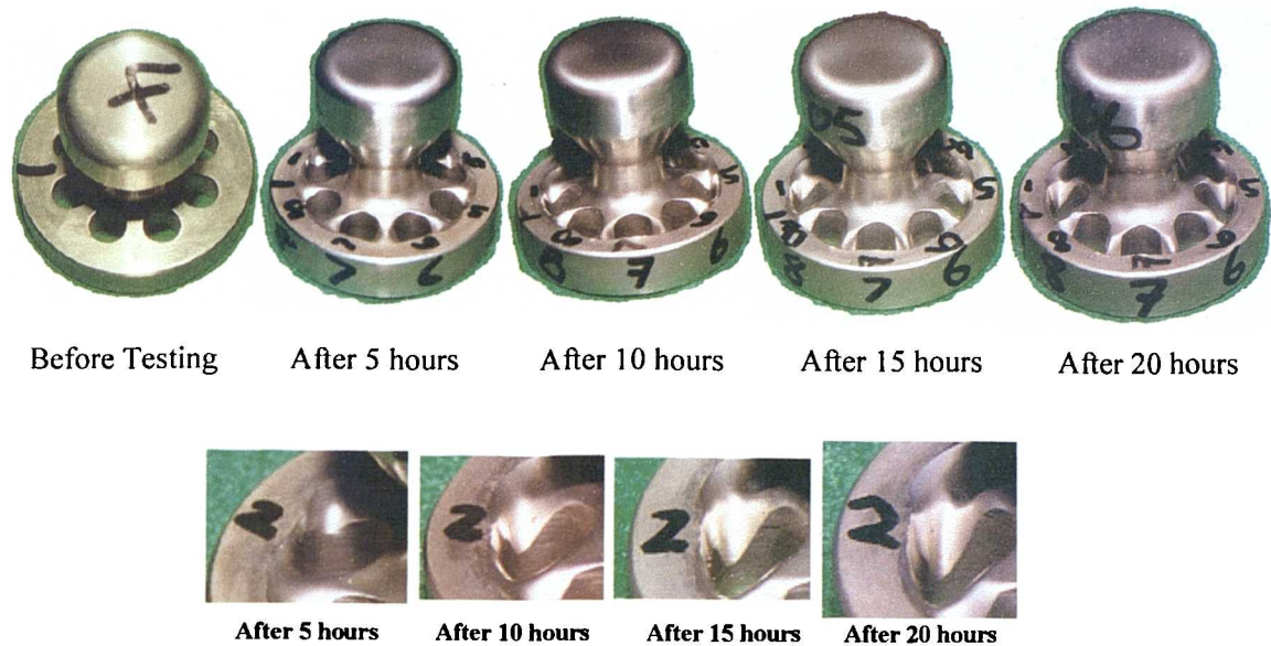
Figure 6.13 Photos of Duplex F51 Upstand restrictor during multiple erosion tests.
