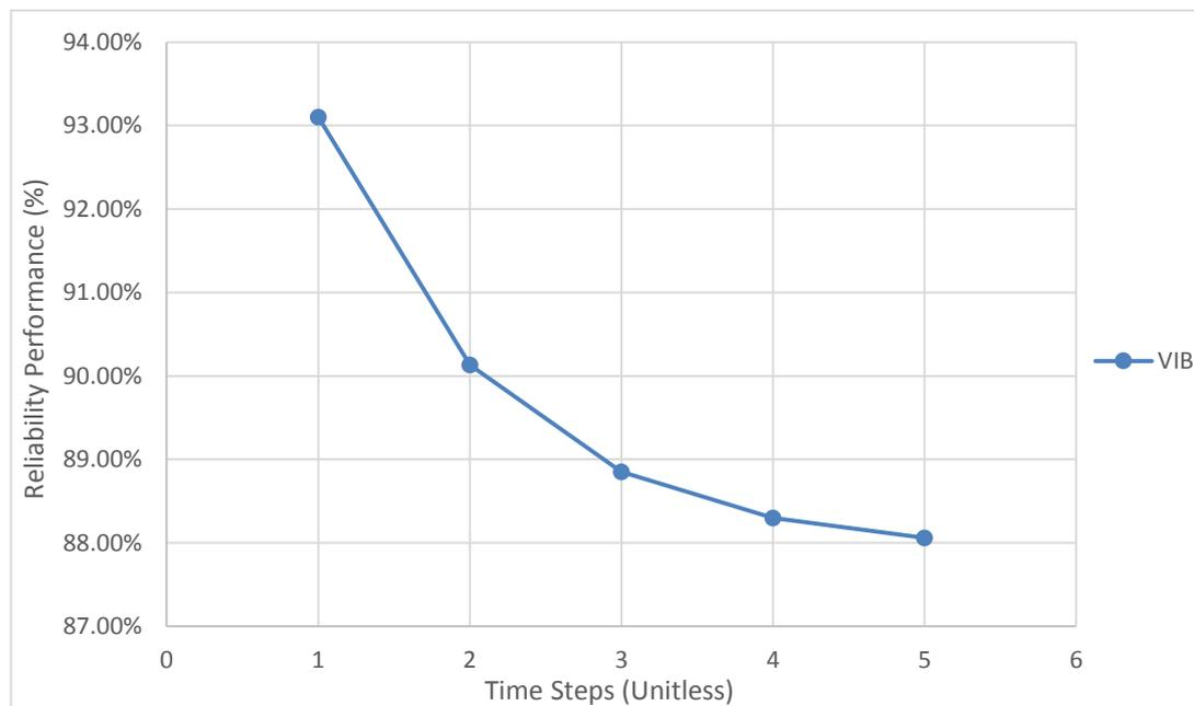
Figure 7.7 Reliability performance of Diesel Generator (D/G) pistons
