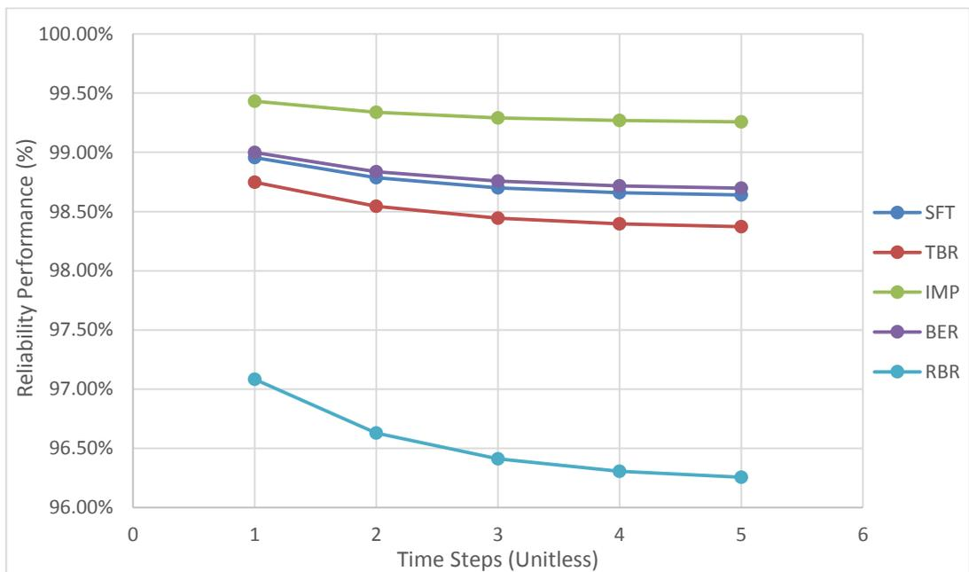
Figure G.51 Reliability performance of crude oil handling pump mechanical power subsystem
