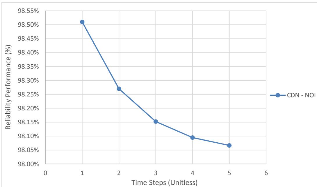
Figure G.39 Reliability performance of Cooling Water Pump (CW) coupling driven
