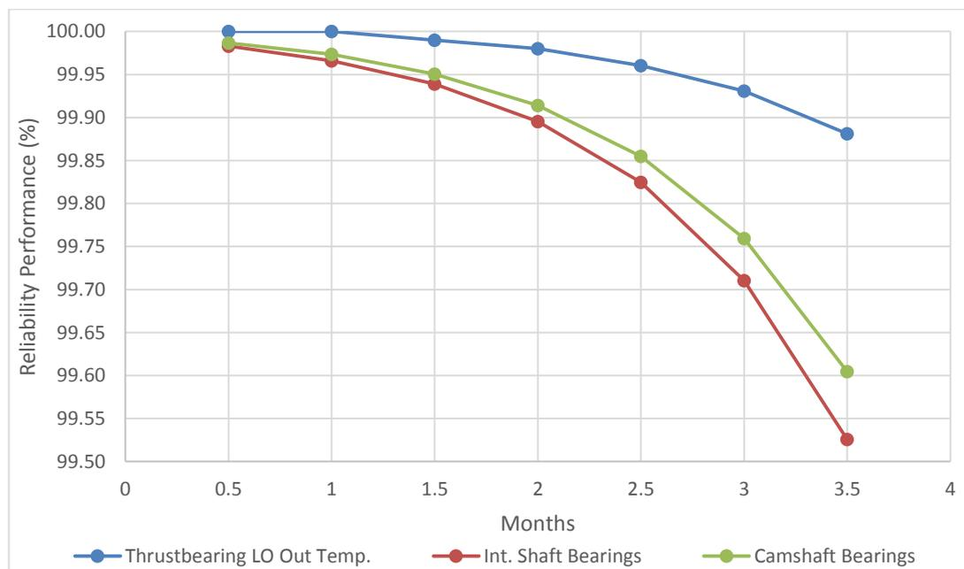
Figure 7.29 Reliability performance of bearing drive system – raw data
