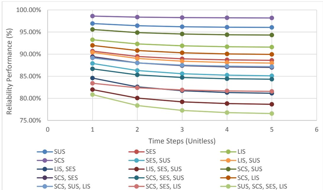
Figure G.1 Reliability performance of Diesel Generator (D/G) starting subsystem
