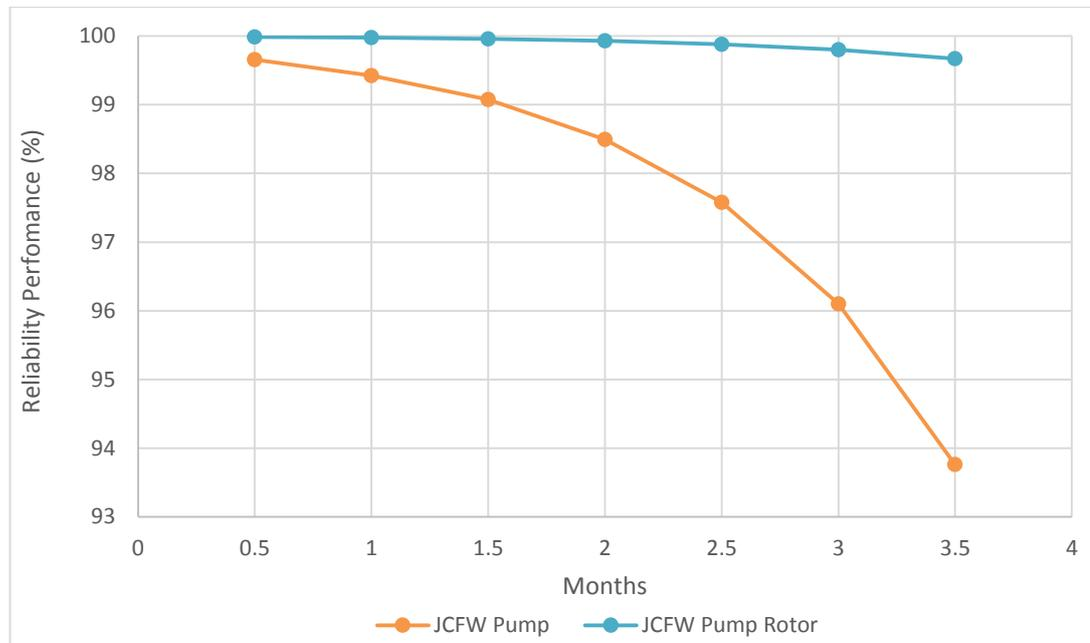
Figure 7.26 Reliability performance of jacket cooling fresh water system – raw data
