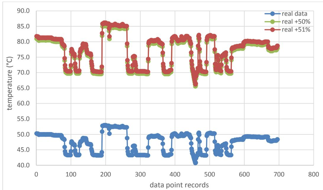
Figure 8.5 Thrust bearing lube oil outlet temperature scenarios analysis
