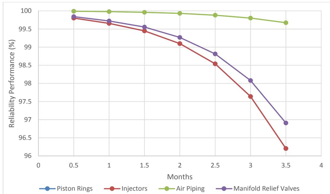
Figure 7.28 Reliability performance of air supply system – raw data
