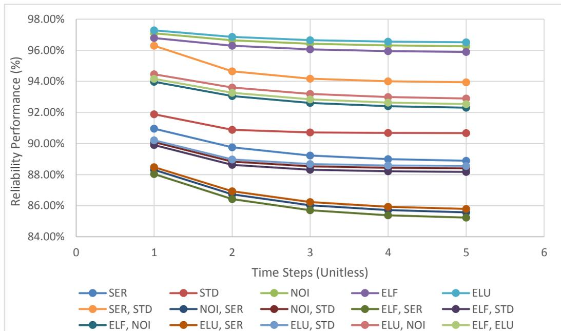
Figure G.13 Reliability performance of Diesel Generator (D/G) exhaust (involving one and two components)
