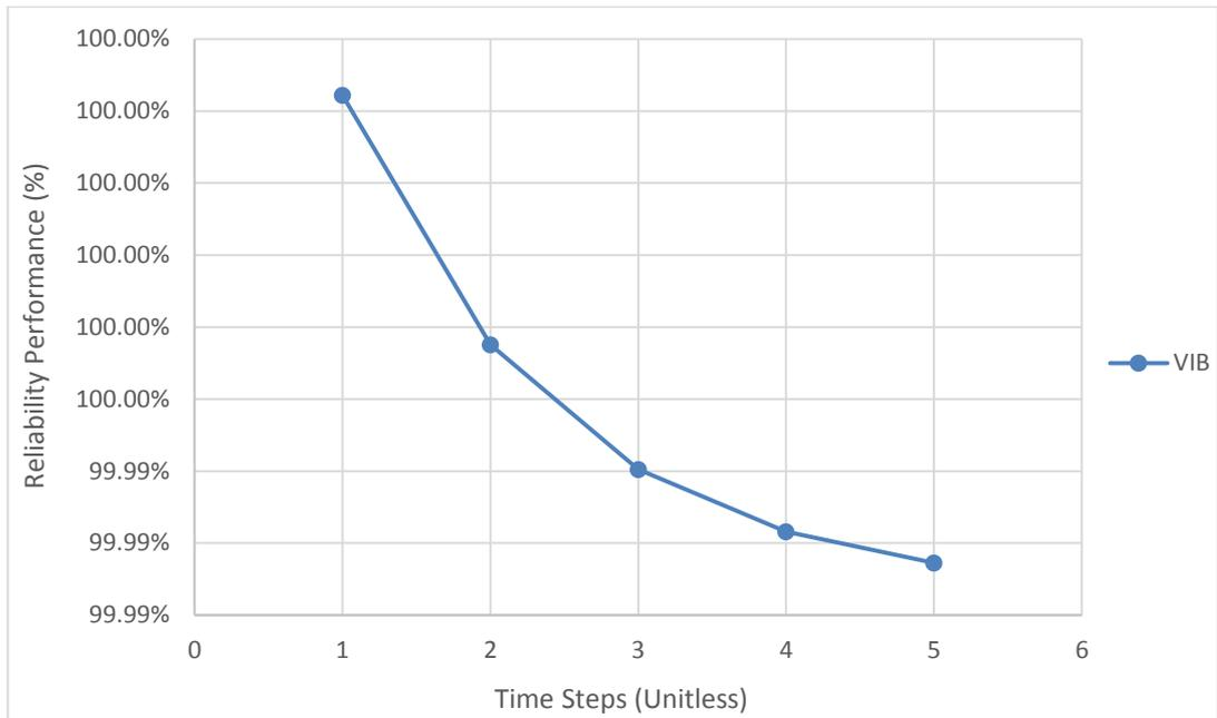
Figure G.26 Reliability performance of seawater lift pump coupling driver
