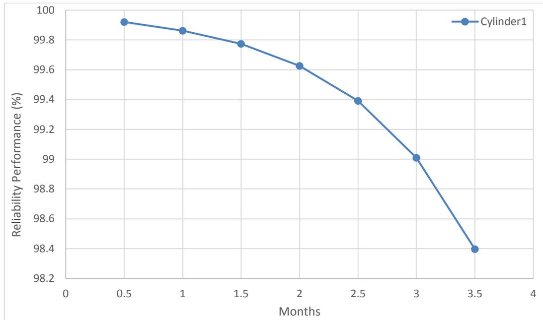
Figure 7.30 Reliability performance of cylinder 1 – raw data
