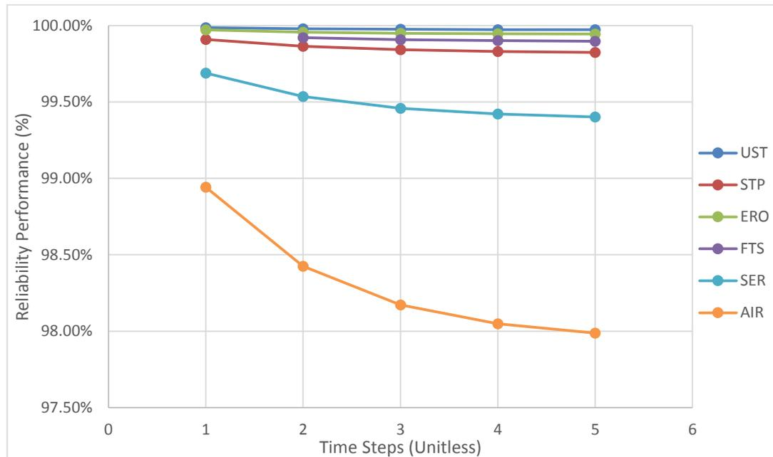
Figure 7.22 Reliability performance of Firefighting Pump (FP) control unit
