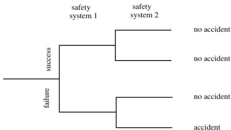
Figure 4.7 Sample of event tree structure (Bedford and Cooke, 2001)
