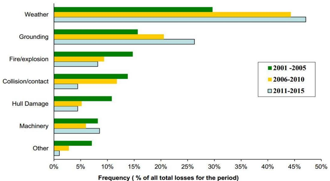
Figure 1.3 Ship total losses by cause for all vessel types 2000-2014 vessels 500 GT and above (IUMI, 2016b)
