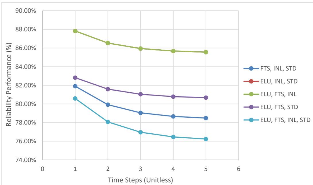
Figure G.11 Reliability performance of Diesel Generator (D/G) cylinders (involving three and four components)
