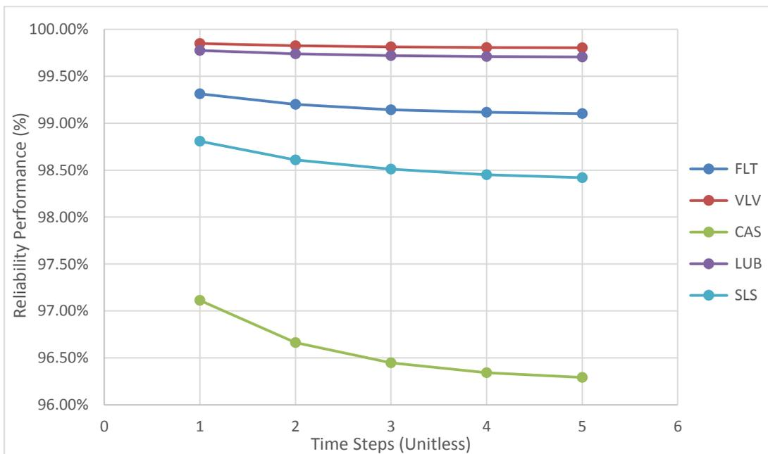
Figure G.32 Reliability performance of oil export pump shell subsystem
