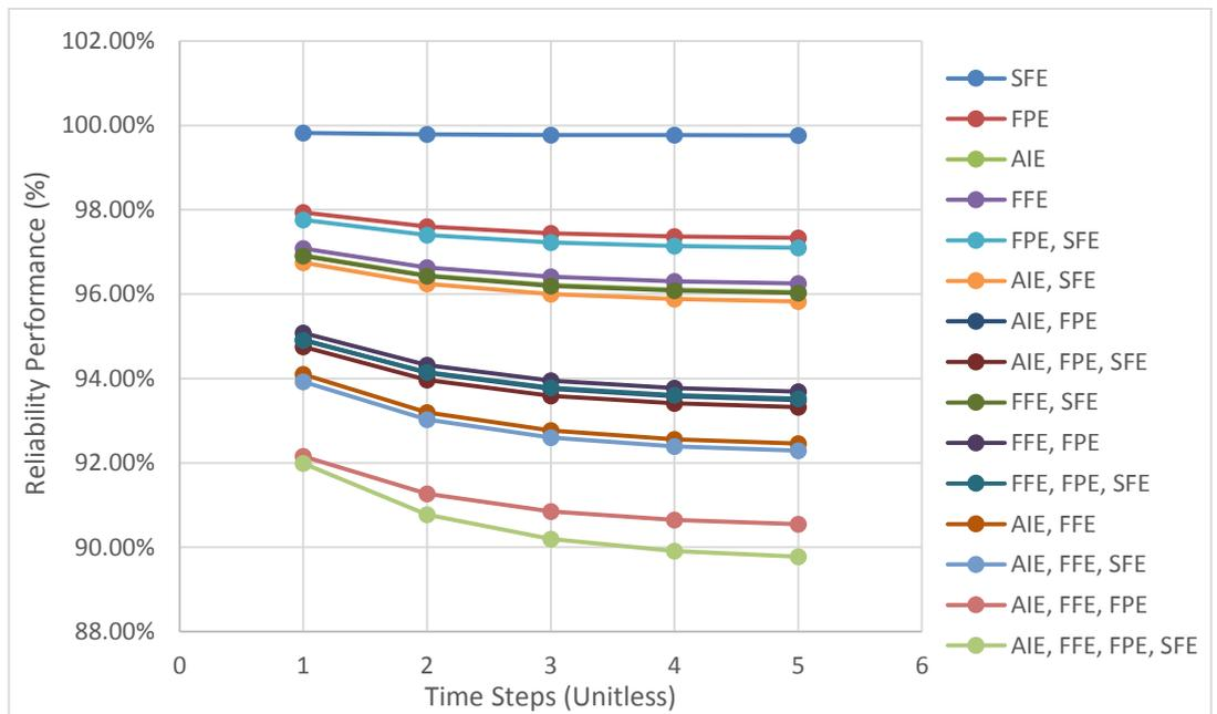
Figure G.4 Reliability performance of Diesel Generator (D/G) engine external components subsystem
