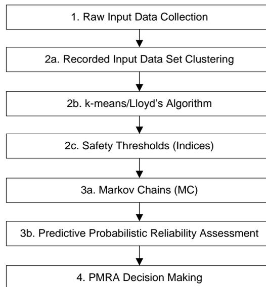
Figure 4.3 PMRA strategy method and tool selection flow diagram for raw data
