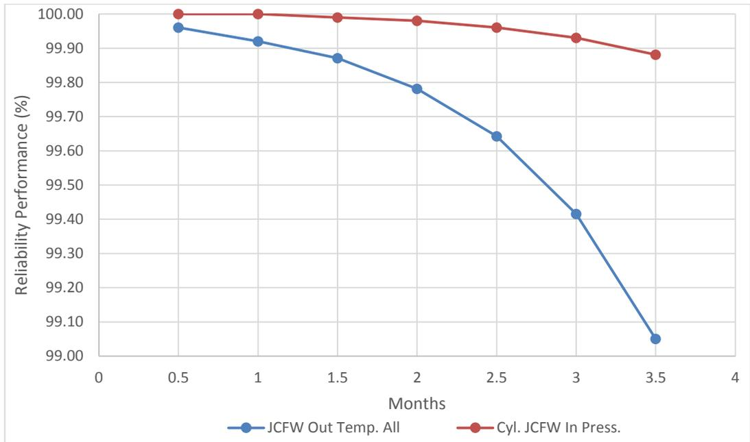
Figure G.64 Reliability performance of JCFW pump housing – raw data
