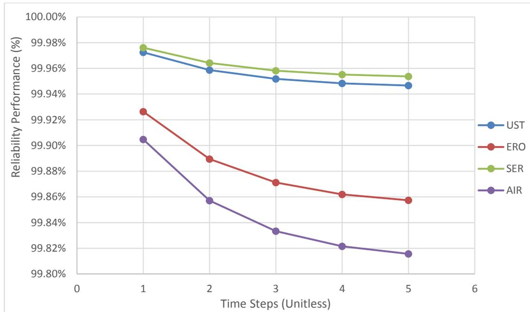
Figure 7.24 Reliability performance of crude oil handling pump control unit
