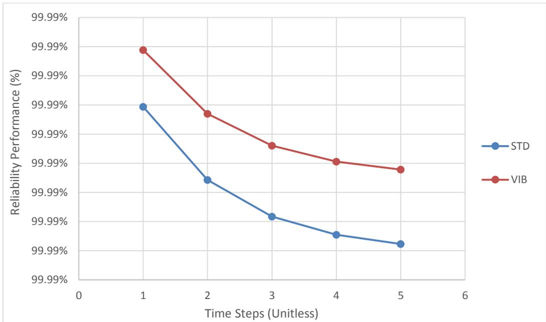
Figure G.35 Reliability performance of oil export pump impeller
