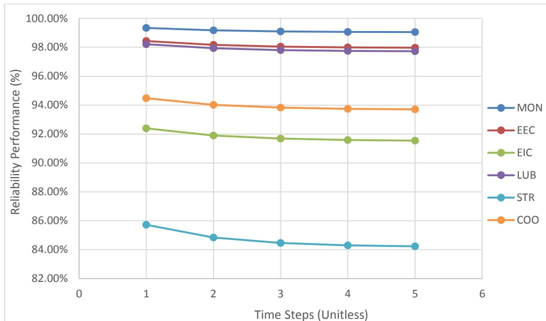
Figure 7.1 Reliability performance of diesel generator (D/G) subsystem level
