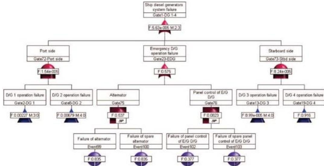
Figure 4.6 Sample of Fault Tree structure (Lazakis, 2011)
