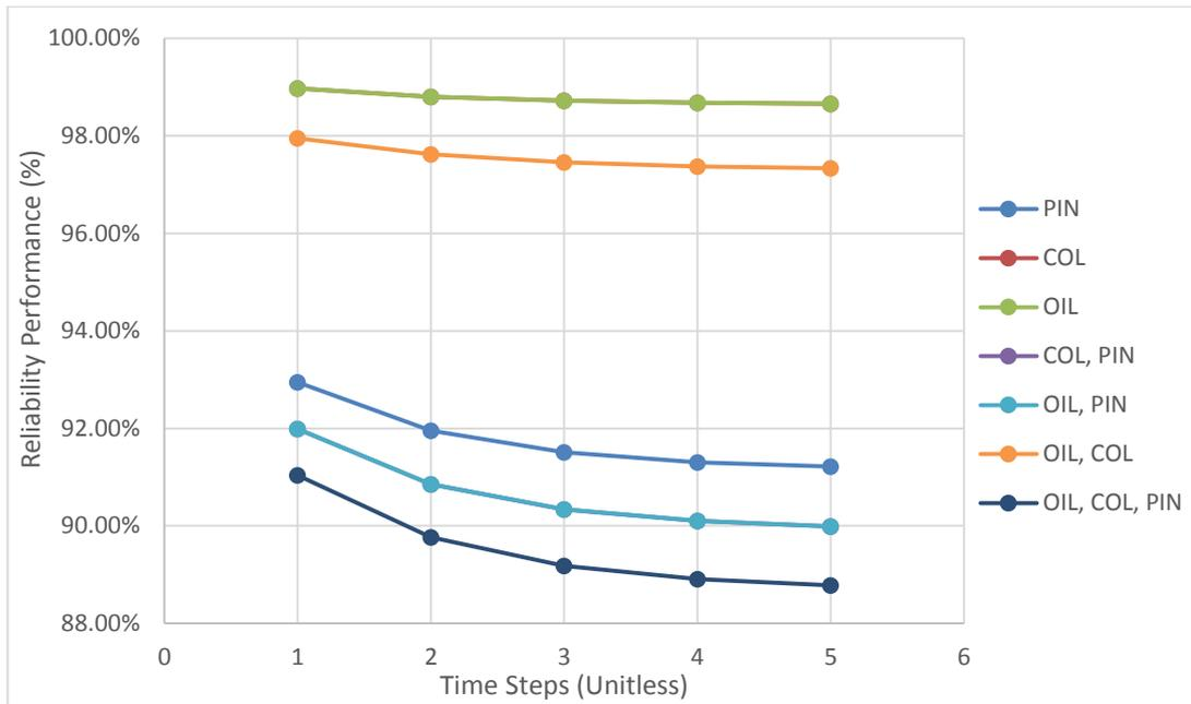
Figure G.2 Reliability performance of Diesel Generator (D/G) lubrication subsystem
