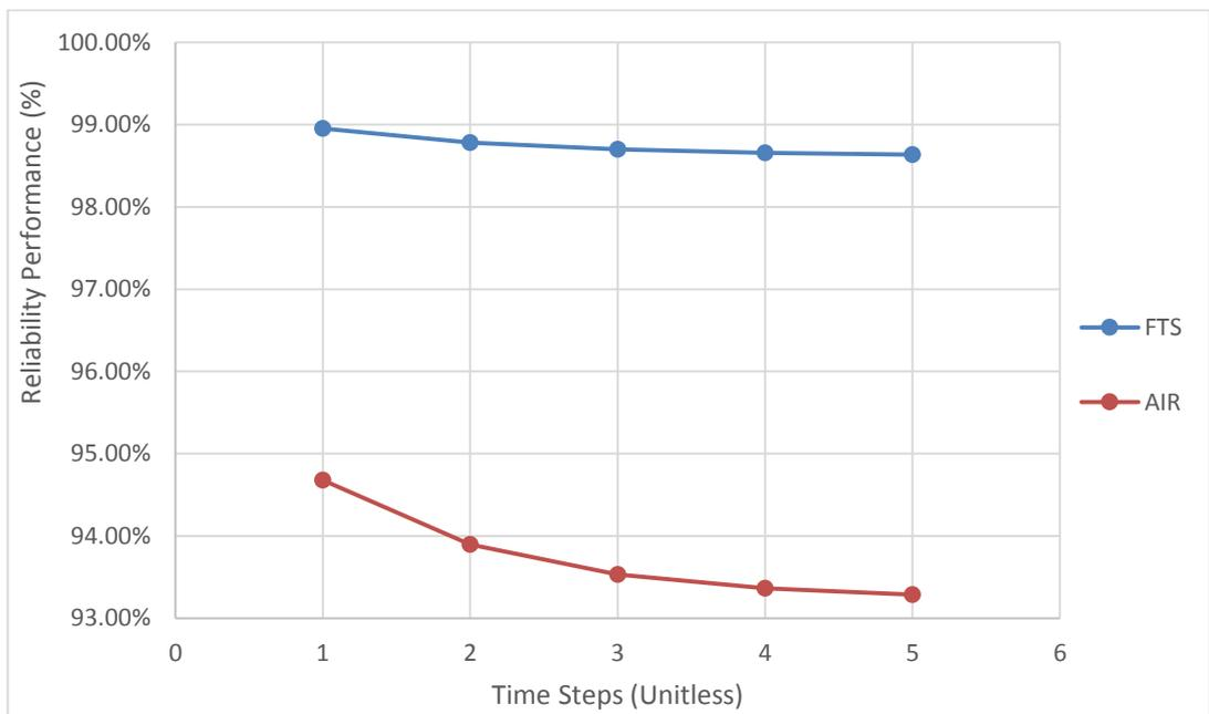
Figure G.9 Reliability performance of Diesel Generator (D/G) control unit
