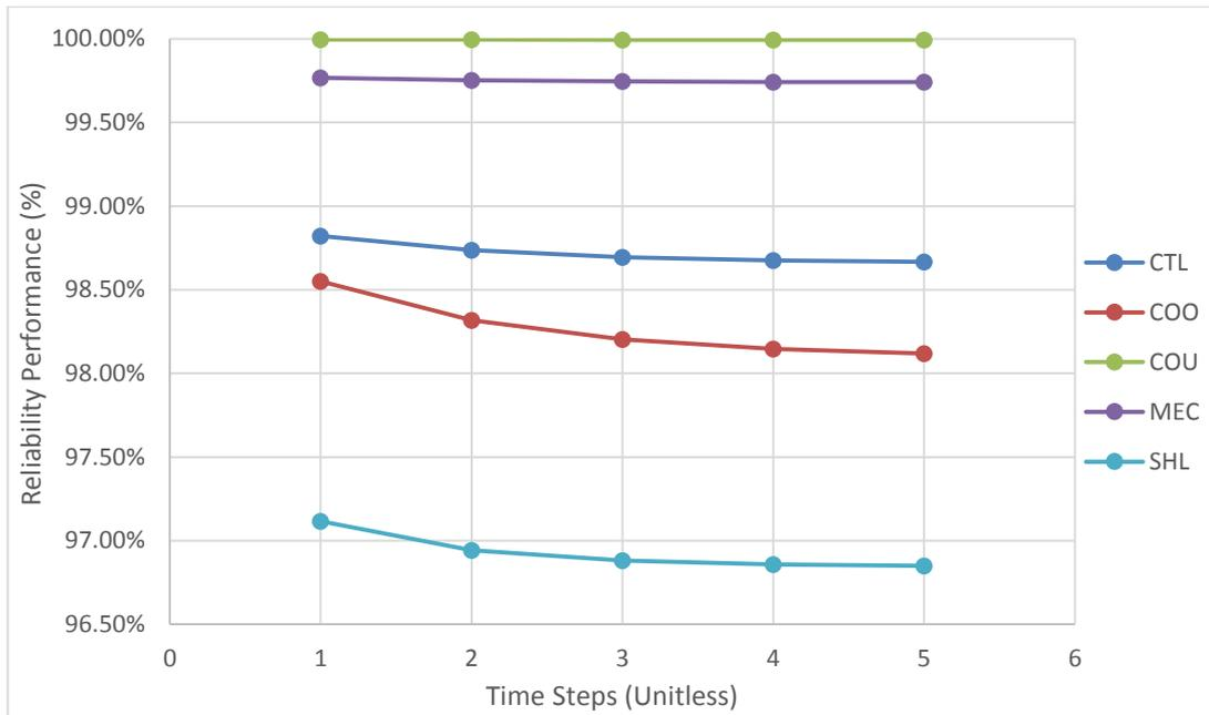
Figure 7.16 Reliability performance of oil export pump subsystem level
