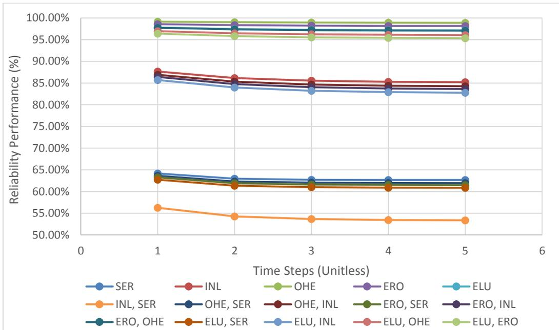
Figure G.12 Reliability performance of Diesel Generator (D/G) injections (involving one and two components)
