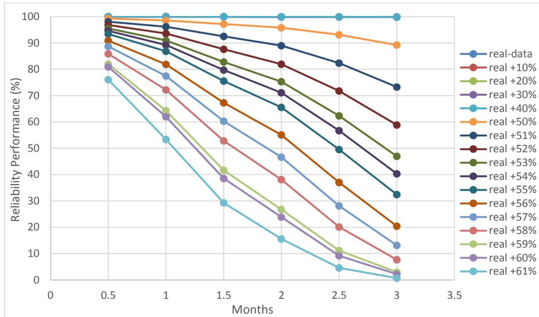
Figure 8.4 Incremental scenario analysis of thrust bearing
