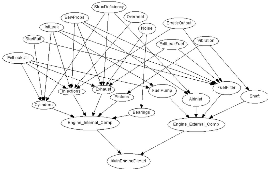
Figure 4.8 Sample of Bayesian Belief Network (BBN) structure (Dikis et al., 2014)
