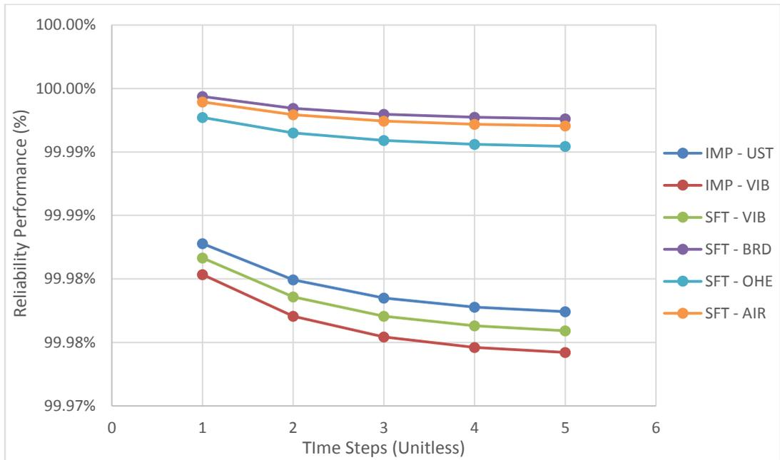
Figure G.58 Reliability performance of crude oil handling pump impeller and shaft (IMP and SFT)
