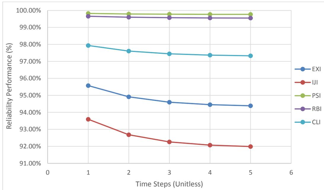
Figure G.5 Reliability performance of Diesel Generator (D/G) engine internal components subsystem (involving one component)
