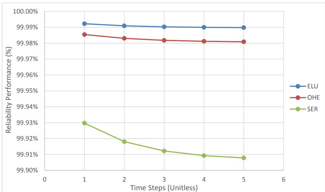
Figure G.57 Reliability performance of crude oil handling pump cooling system (failure mode level)
