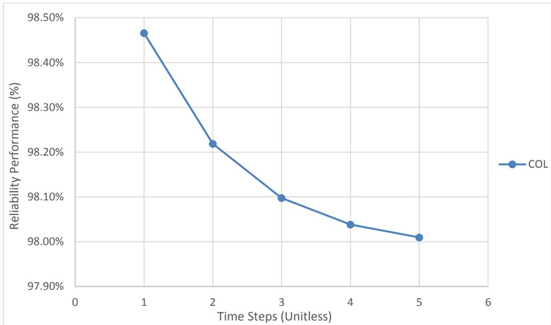
Figure G.29 Reliability performance of oil export pump cooling subsystem
