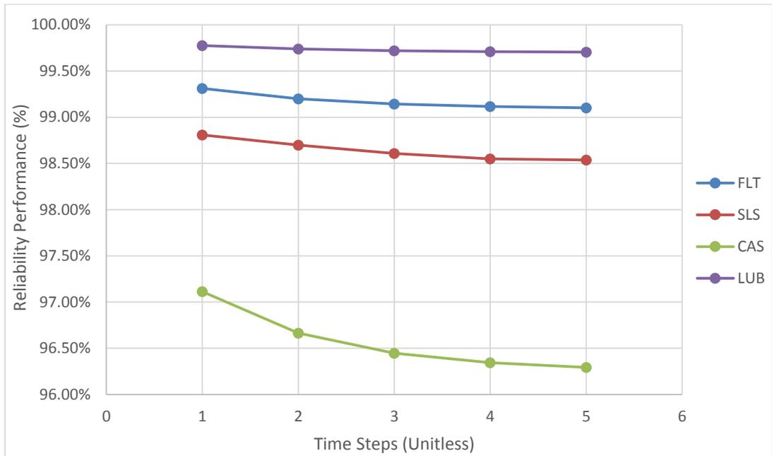
Figure G.52 Reliability performance of crude oil handling pump shell subsystem
