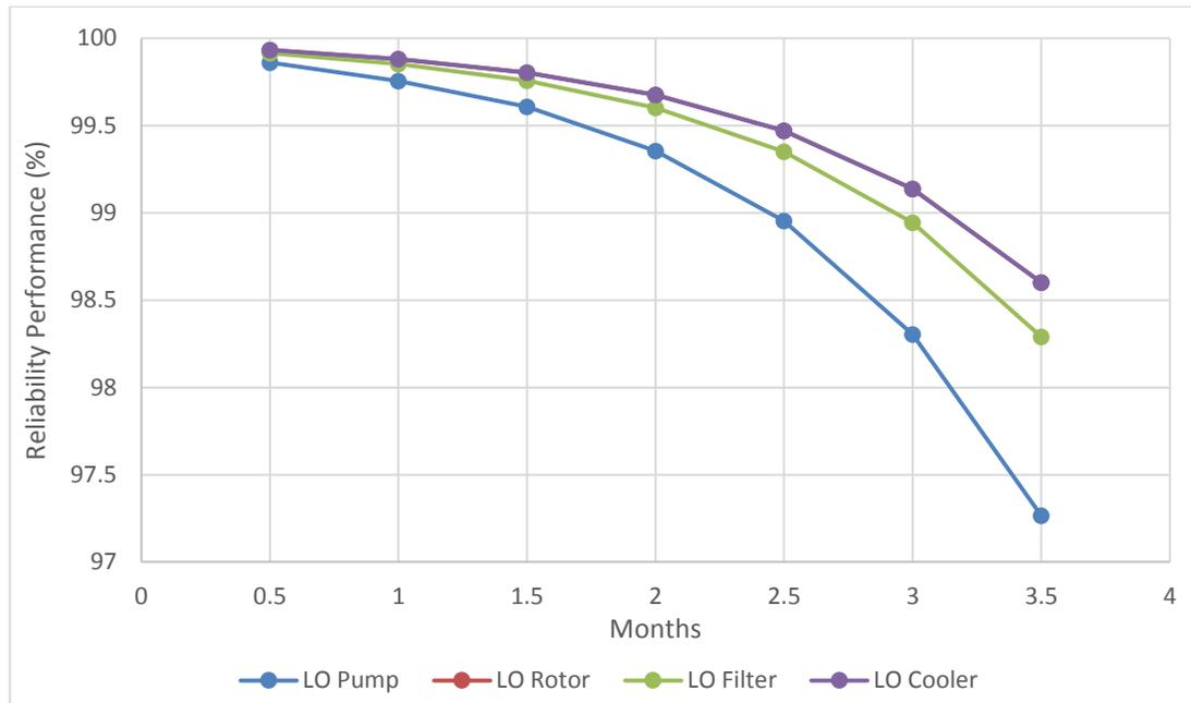
Figure 7.27 Reliability performance of lube oil system – raw data
