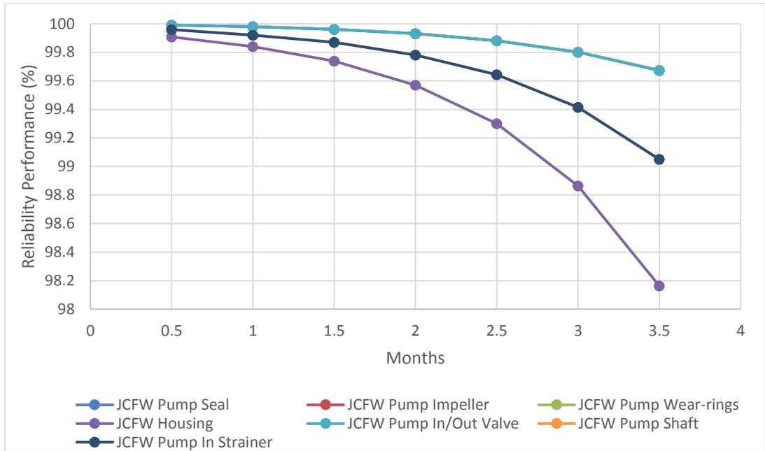
Figure G.62 Reliability performance of JCFW pump – raw data
