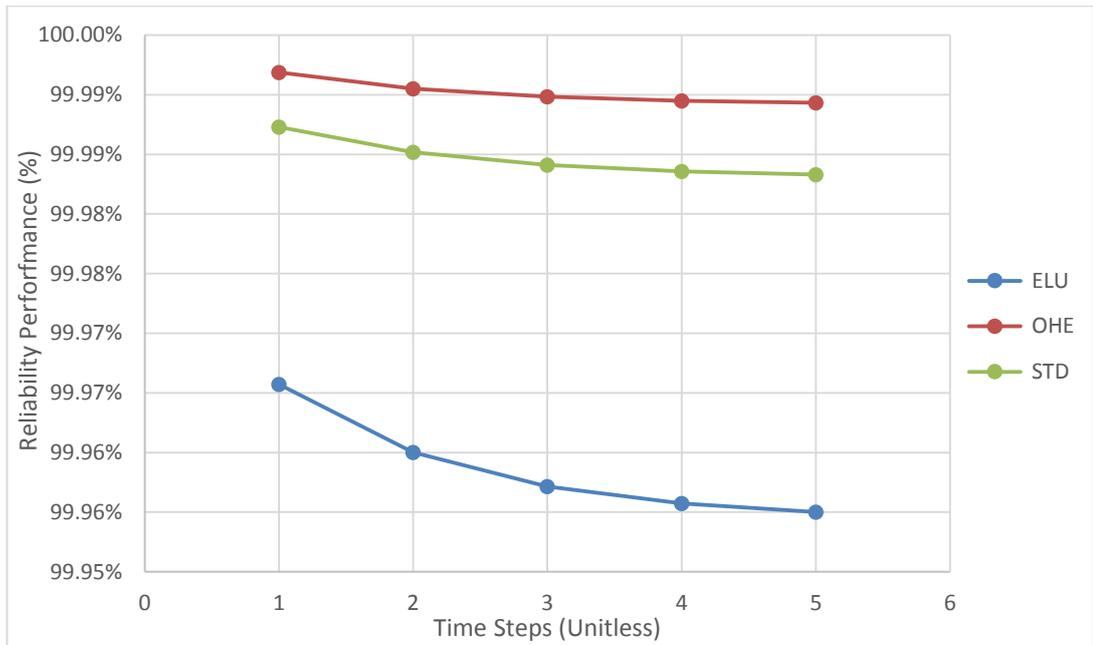
Figure G.45 Reliability performance of Firefighting Pump (FP) casing
