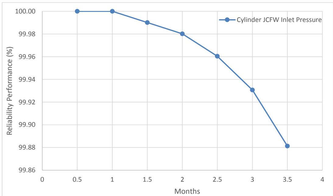
Figure G.63 Reliability performance of JCFW rotor – raw data
