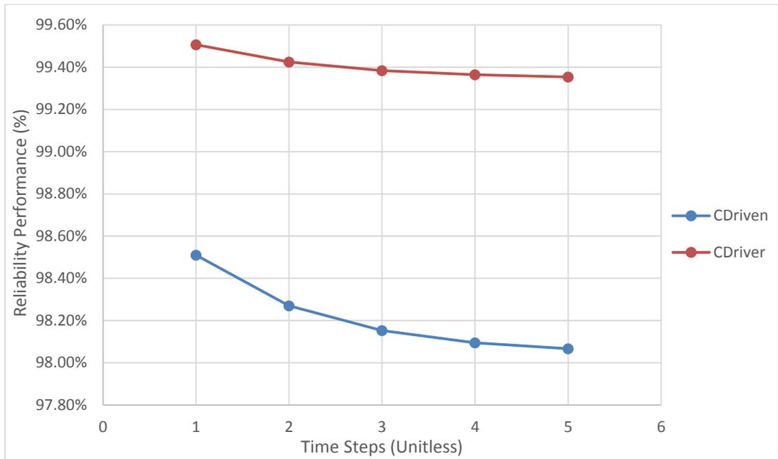
Figure G.50 Reliability performance of crude oil handling pump couplers subsystem
