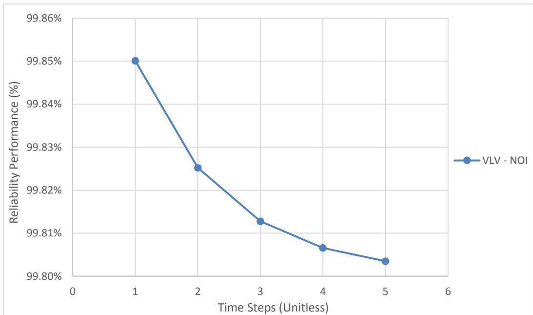
Figure G.41 Reliability performance of Cooling Water Pump (CW) valve
