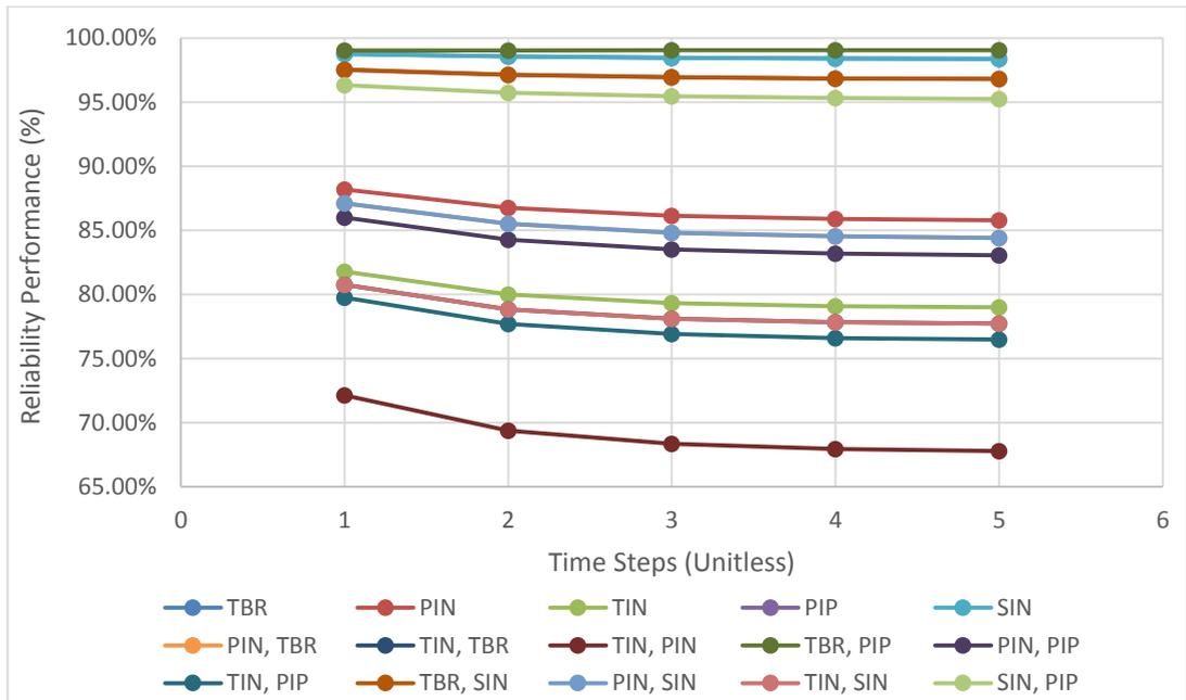
Figure G.19 Reliability performance of Turboexpander expander/recompressor turbine subsystem
