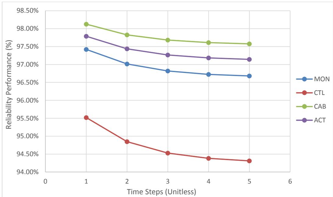
Figure G.48 Reliability performance of crude oil handling pump controller subsystem
