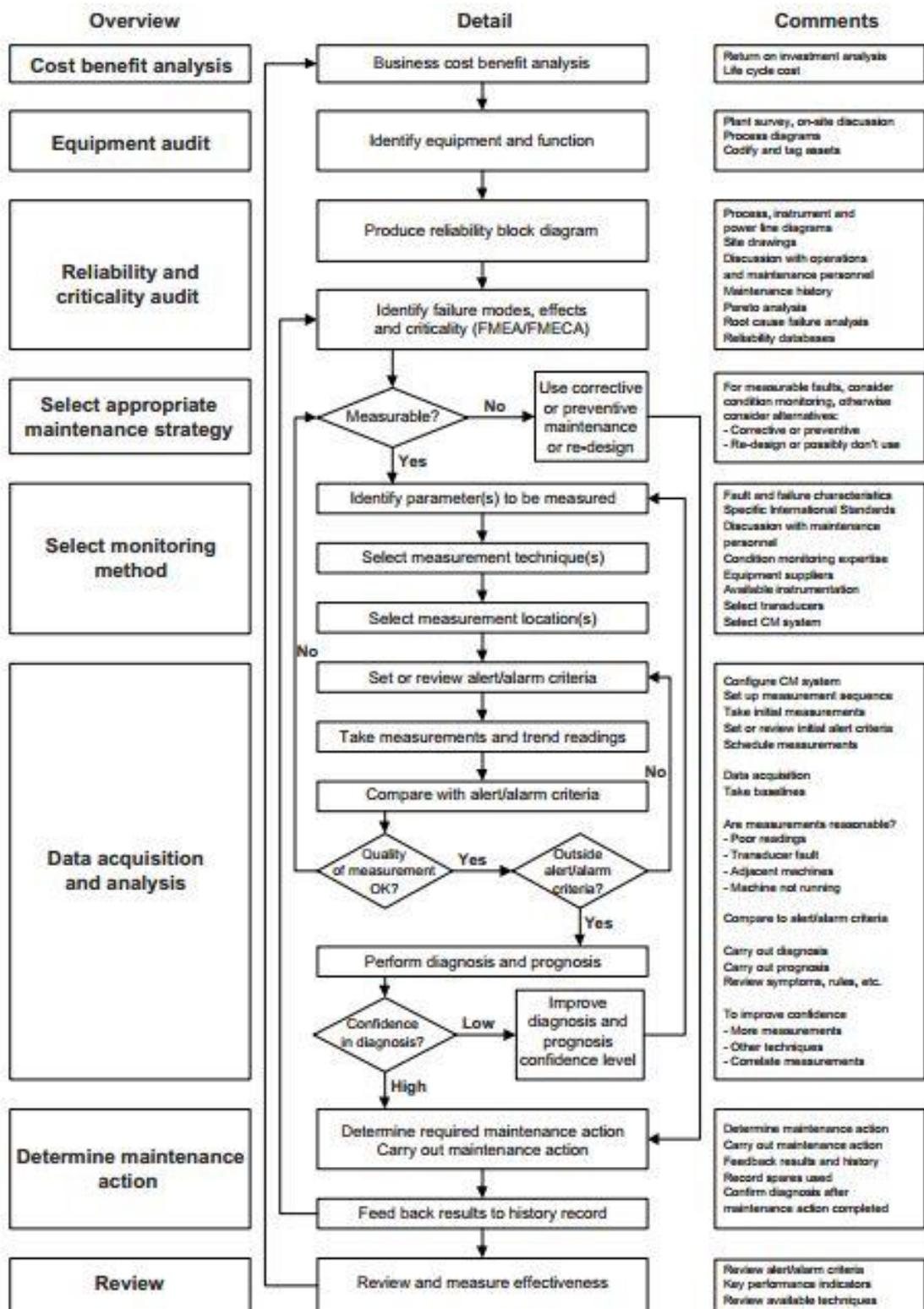
Figure B.1 BS/ISO 17359 (2011) Condition Monitoring (CM) procedure suggestion
