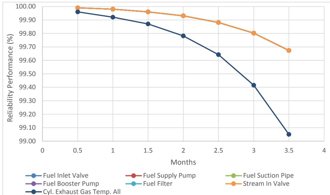
Figure G.60 Reliability performance of fuel supply – raw data
