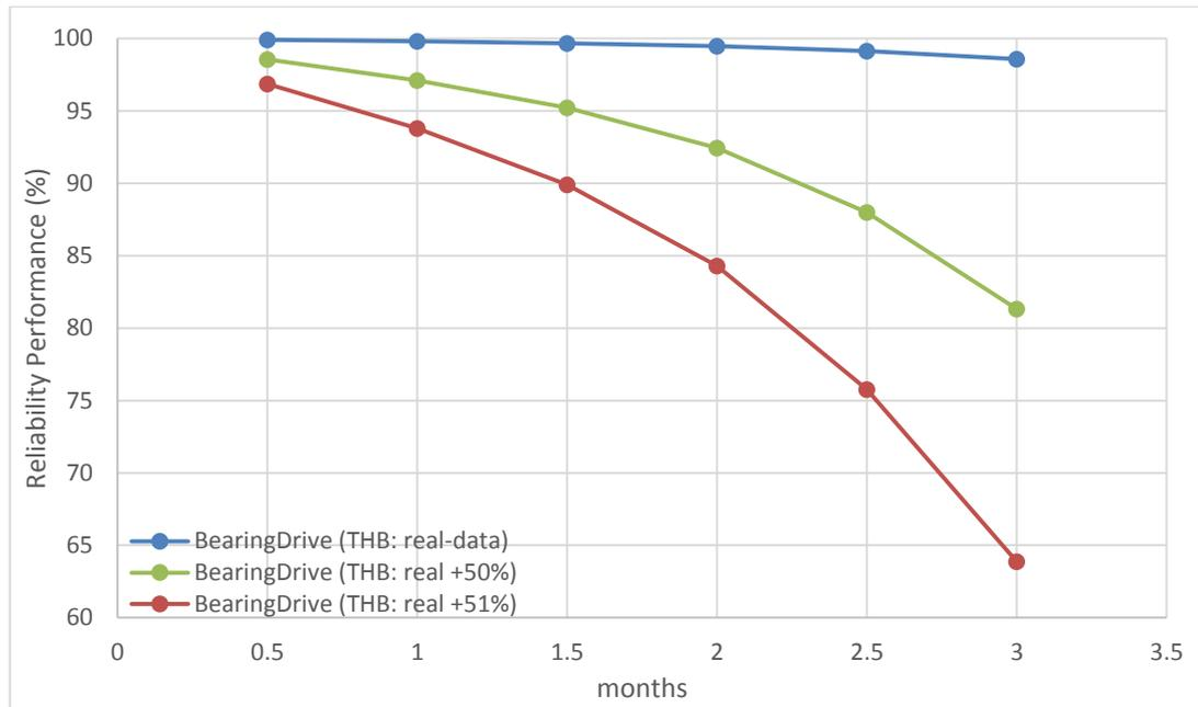
Figure 8.7 Reliability performance of bearing drive for different thrust bearing scenarios
