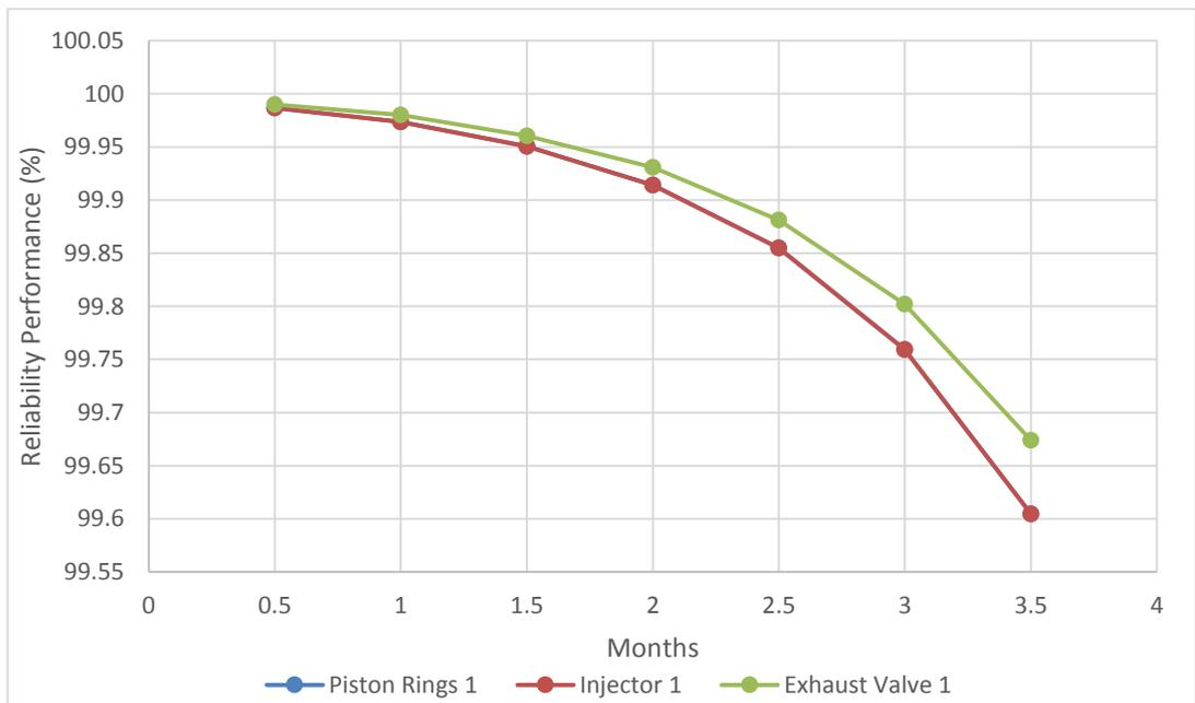
Figure G.69 Reliability performance of Cylinder 1 – raw data
