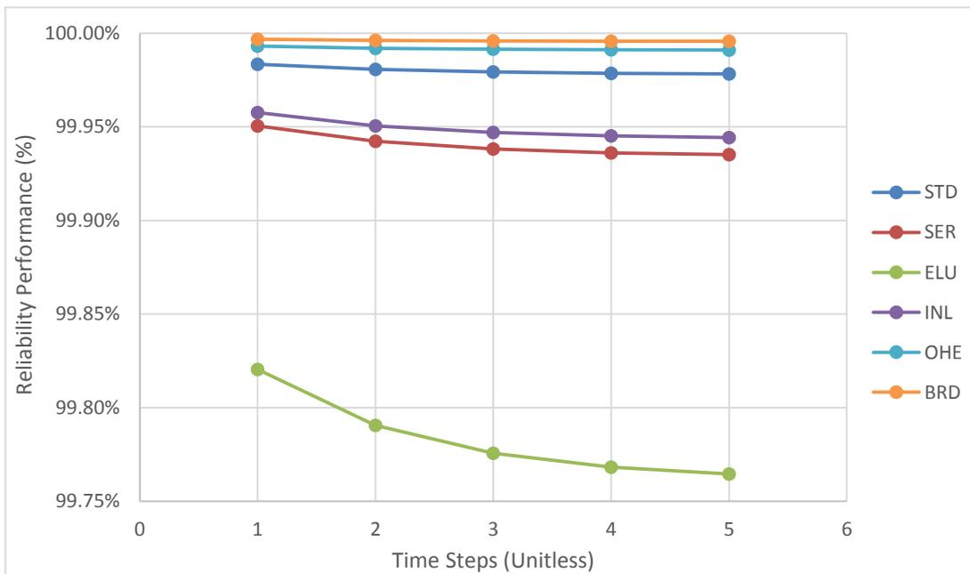
Figure G. 25 Reliability performance of seawater lift pump seals
