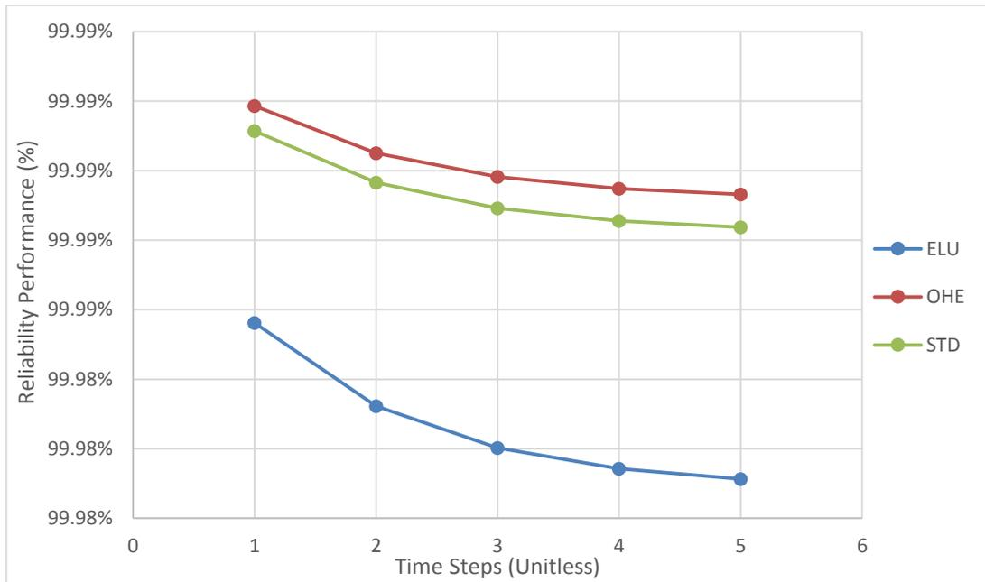
Figure G.47 Reliability performance of Firefighting Pump (FP) thrust bearing
