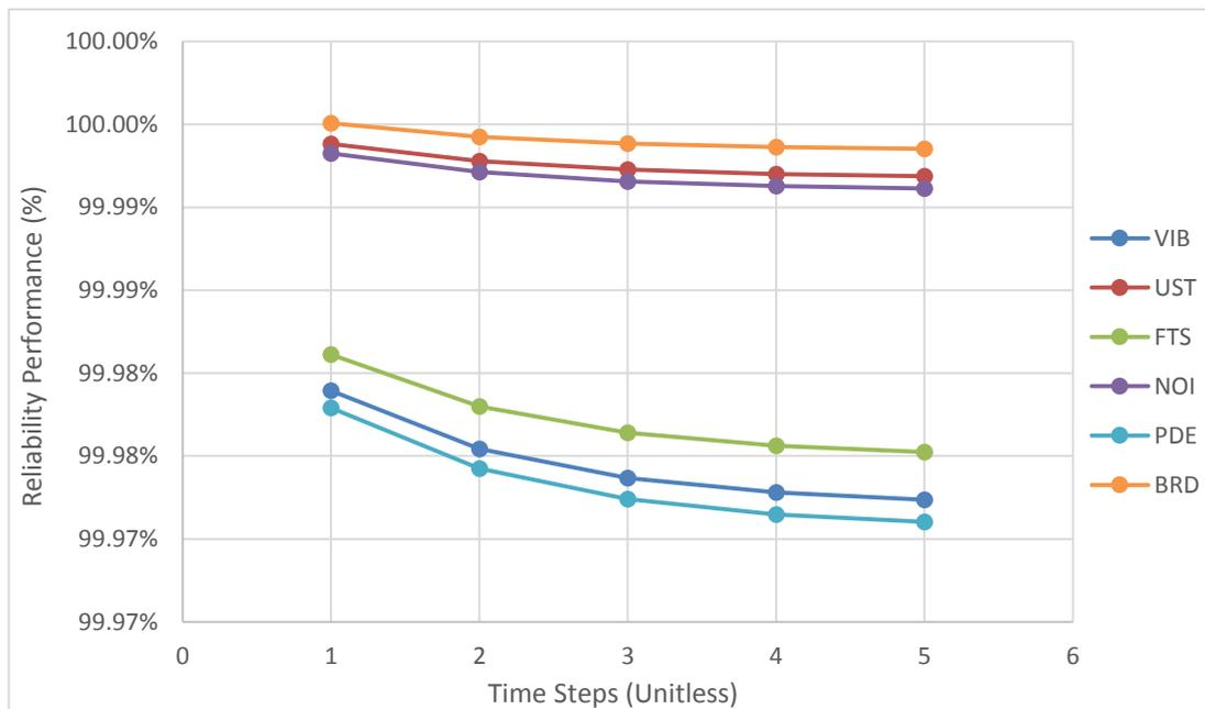
Figure G.27 Reliability performance of seawater lift pump radial bearing
