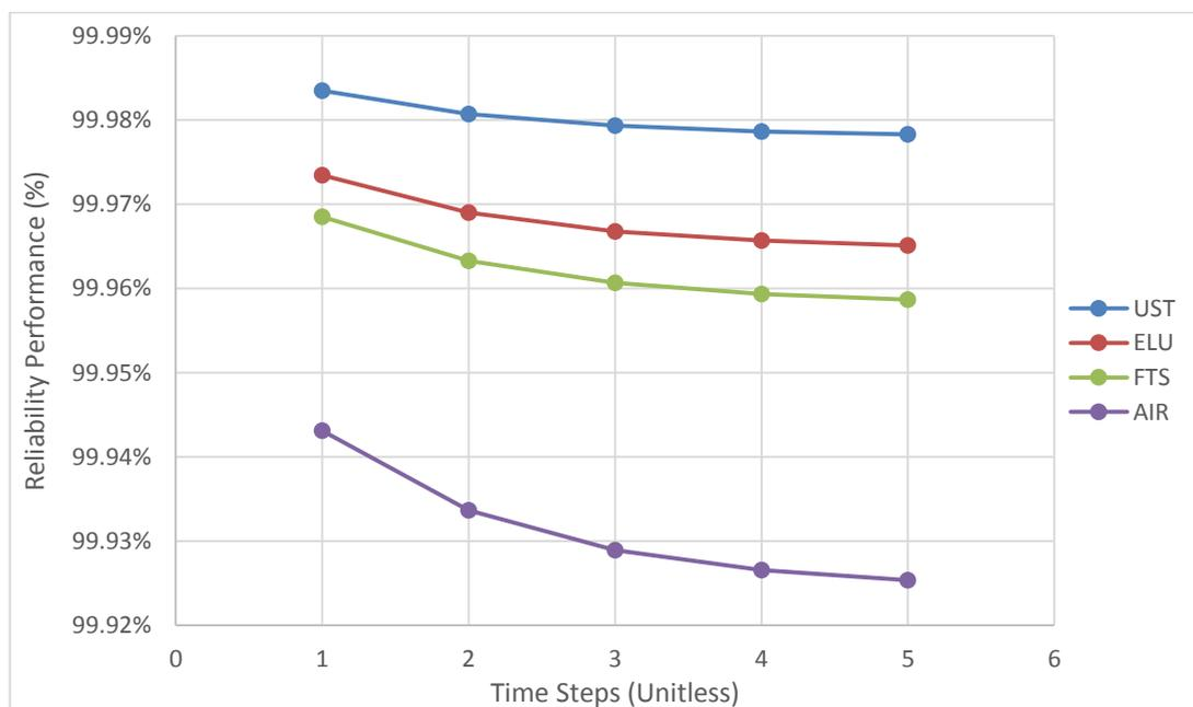
Figure 7.10 Reliability performance of Turboexpander monitoring
