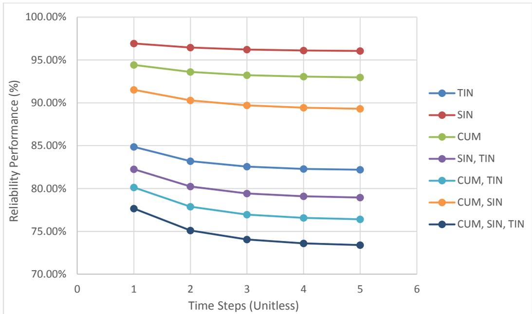
Figure G.3 Reliability performance of Diesel Generator (D/G) control monitoring subsystem
