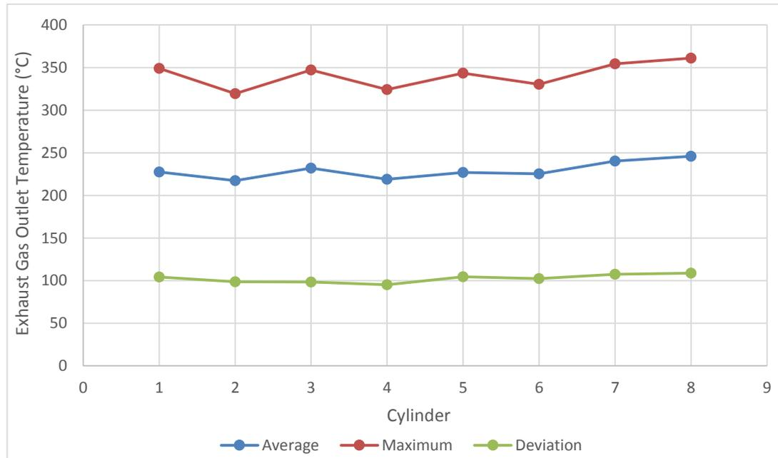
Figure 7.31 Cylinder exhaust gas outlet temperature – raw data records
