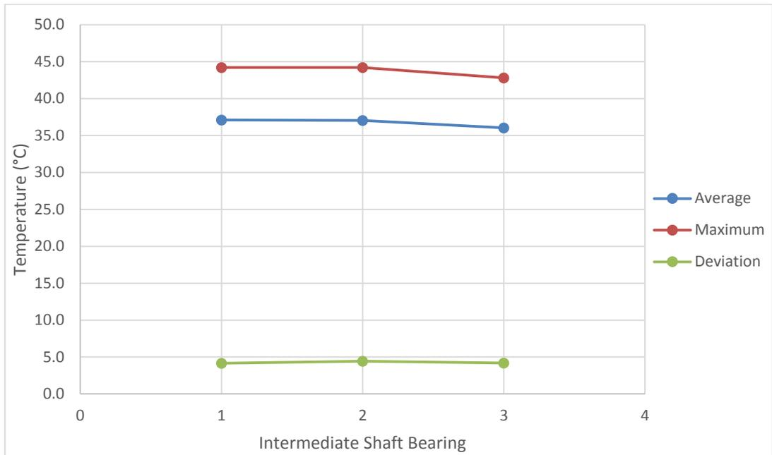
Figure G.68 Intermediate shaft bearing temperature records
