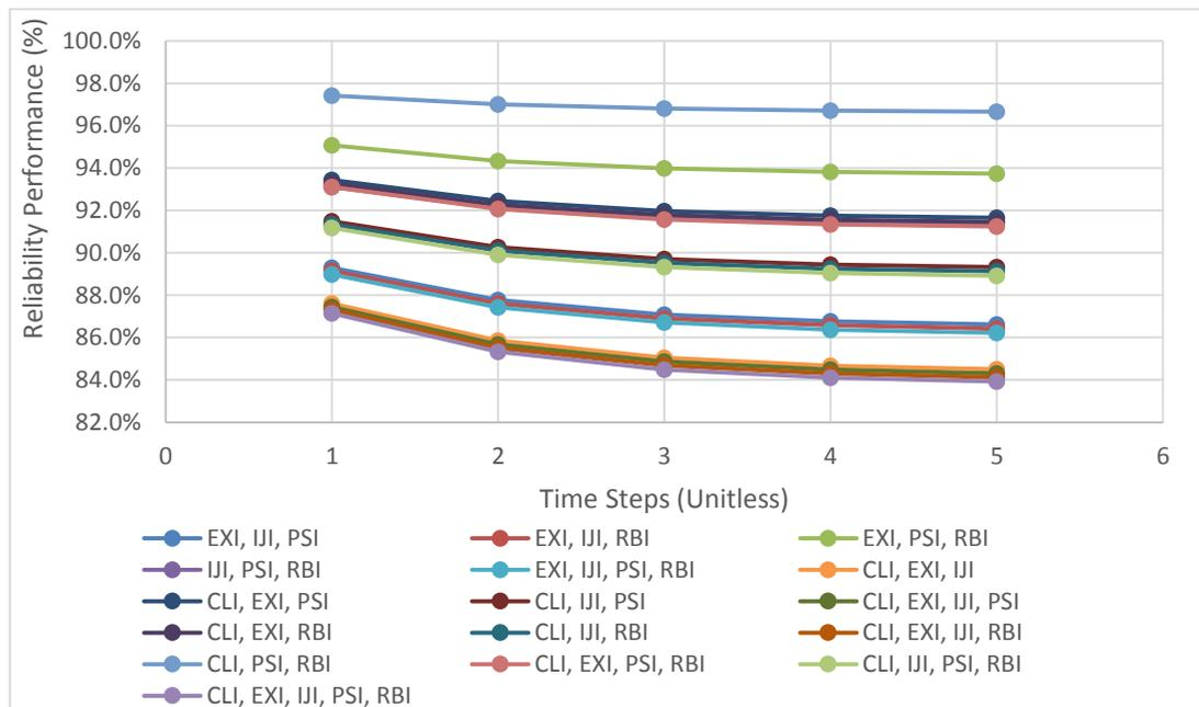
Figure G.7 Reliability performance of Diesel Generator (D/G) engine internal components subsystem (involving three, four and five components)
