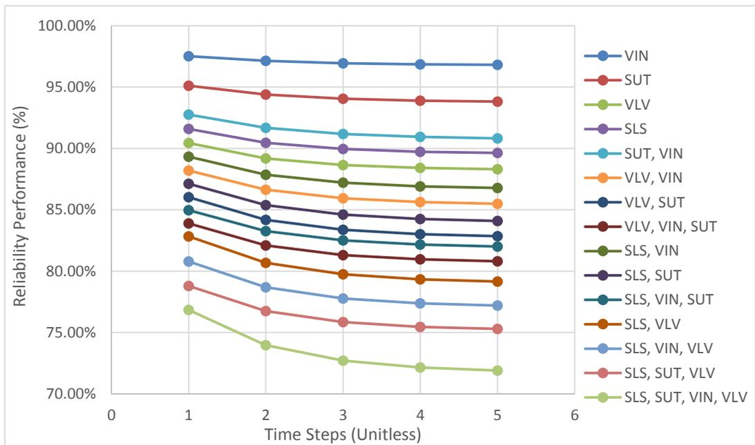
Figure G.20 Reliability performance of Turboexpander shaft and seal subsystem
