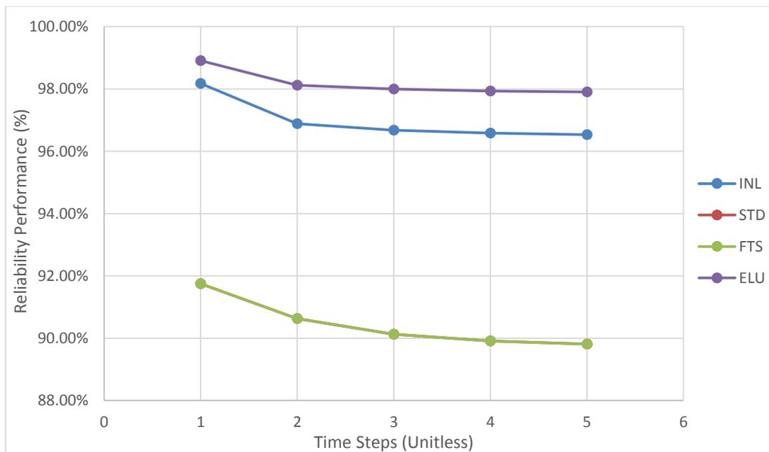
Figure 7.5 Reliability performance of Diesel Generator (D/G) cylinders
