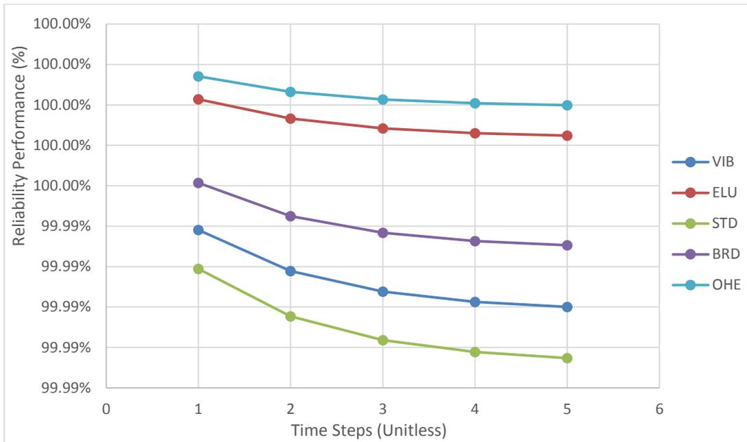
Figure G.28 Reliability performance of seawater lift pump thrust bearing
