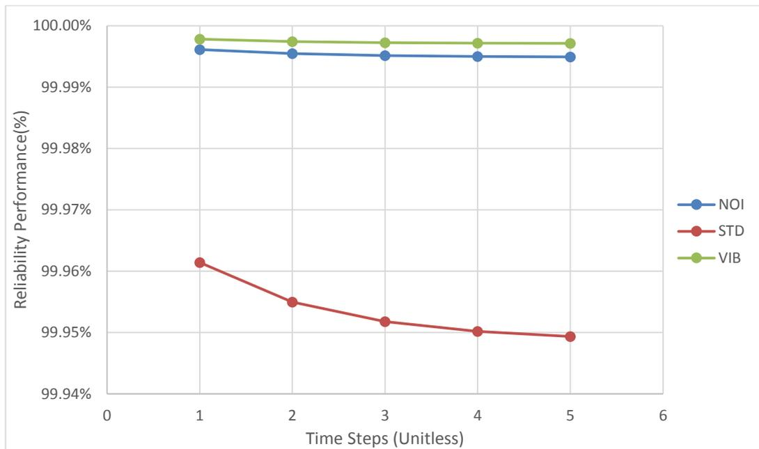
Figure 7.19 Reliability performance of oil export pump coupling driven
