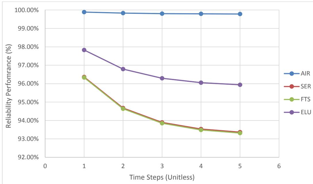
Figure 7.2 Reliability performance of diesel generator (D/G) starting unit
