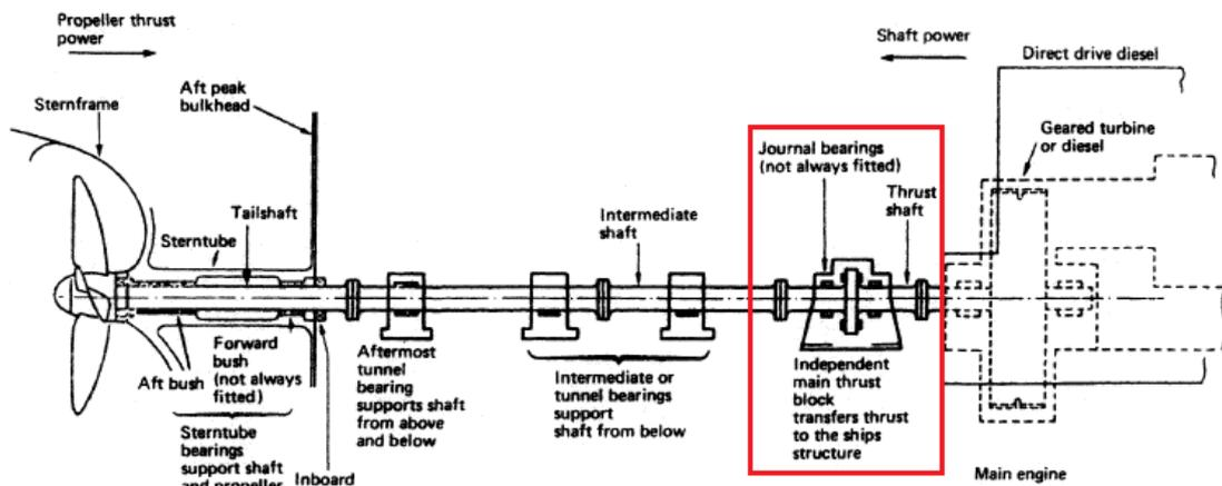
Figure 8.1 Ship shaft transmission layout engine to propeller (Taylor, 1996)
