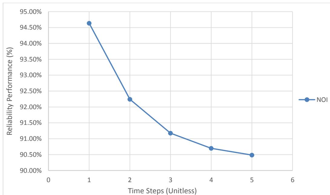
Figure 7.6 Reliability performance of Diesel Generator (D/G) radial bearings
