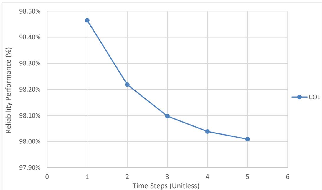
Figure G.49 Reliability performance of crude oil handling pump cooling subsystem
