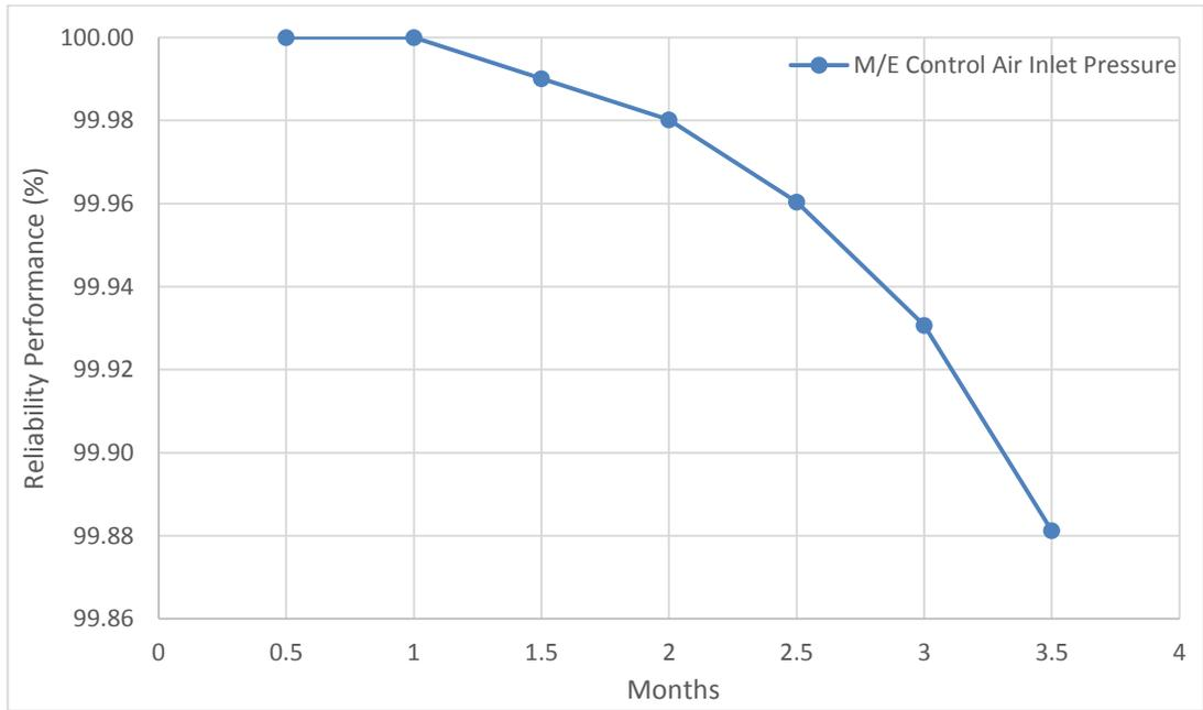
Figure G.66 Reliability performance of air piping – raw data
