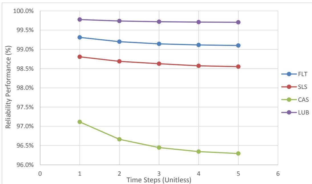
Figure G.44 Reliability performance of Firefighting Pump (FP) shell subsystem
