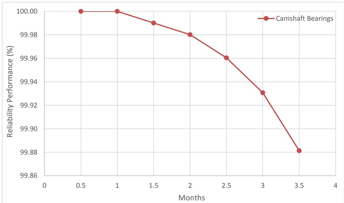
Figure G.67 Reliability performance of camshaft bearings– raw data
