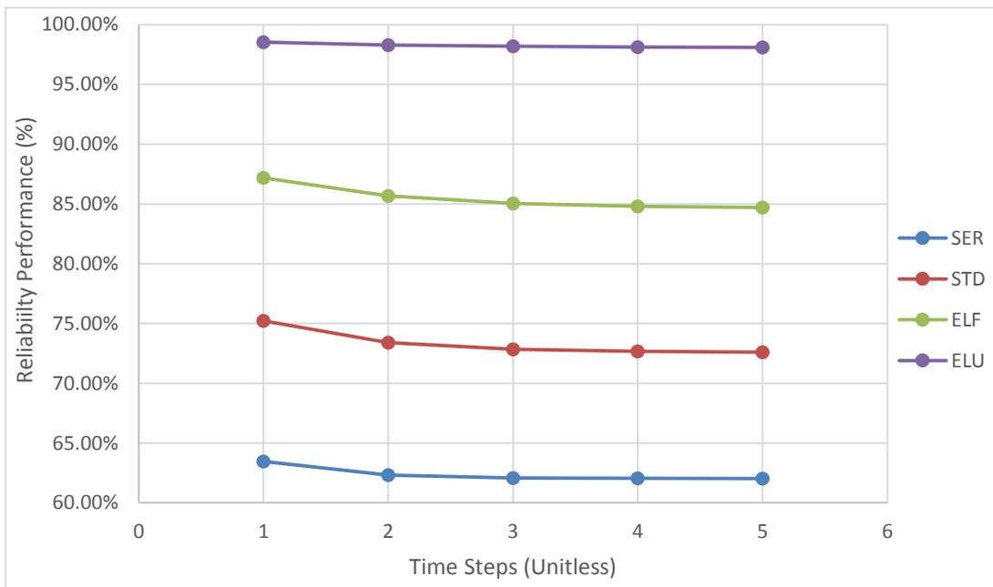
Figure G.17 Reliability performance of Diesel Generator (D/G) piping
