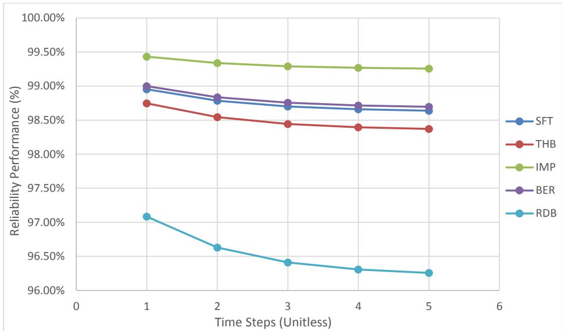
Figure G.31 Reliability performance of oil export pump mechanical power subsystem
