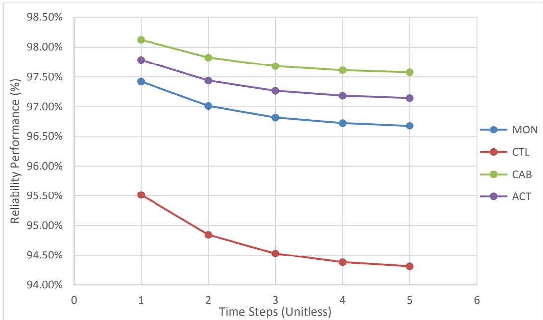
Figure G.40 Reliability performance of Cooling Water Pump (CW) controller subsystem
