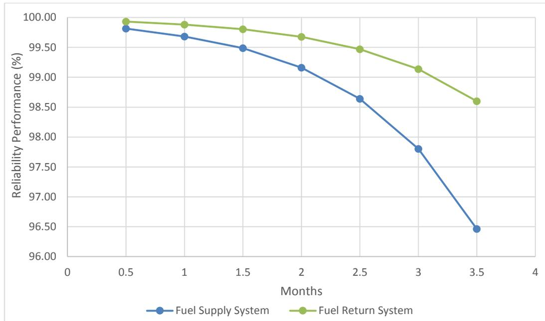
Figure 7.25 Reliability performance of fuel system – raw data
