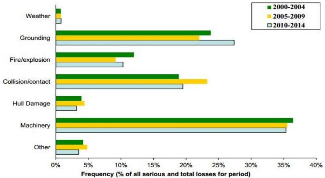
Figure 1.2 Ship serious losses by cause for all vessel types 2000-2014 vessels 500 GT and above (IUMI, 2015)
