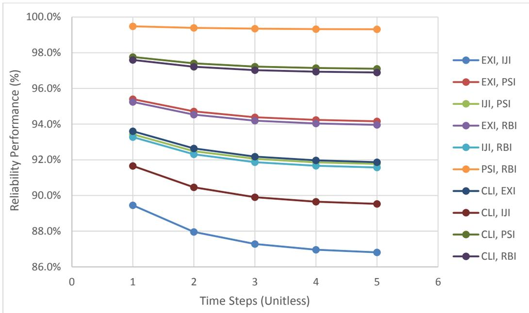
Figure G.6 Reliability performance of Diesel Generator (D/G) engine internal components subsystem (involving two components)
