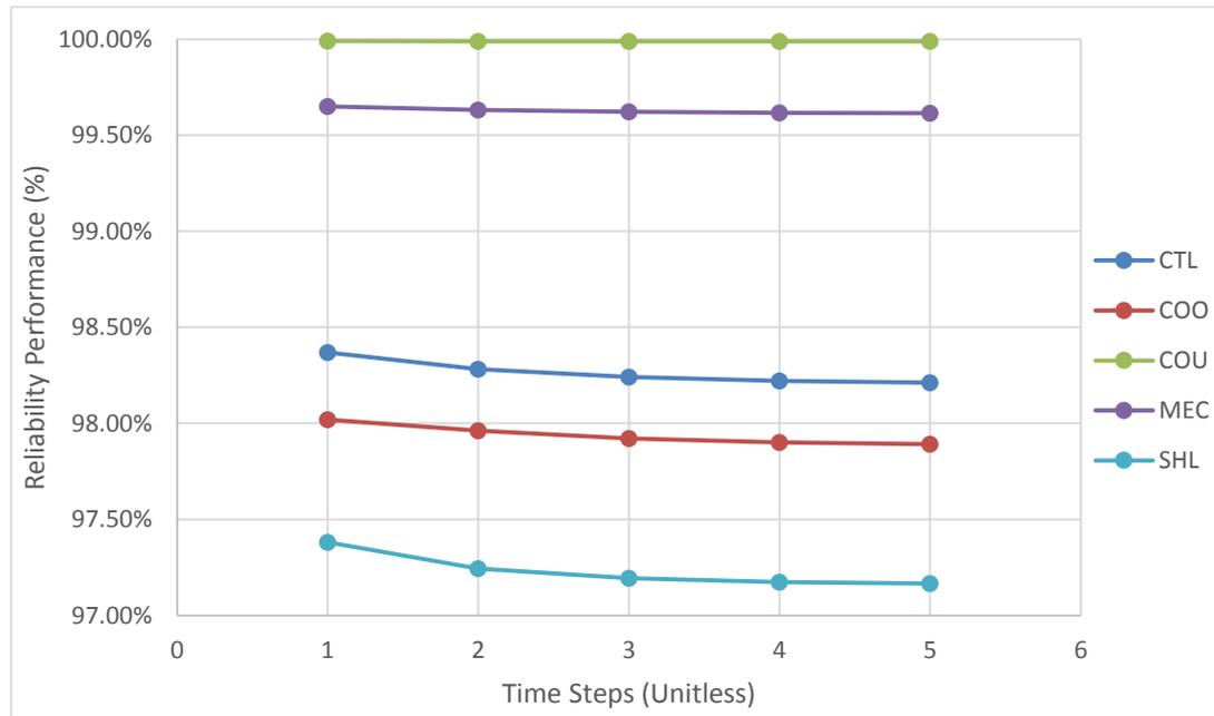
Figure 7.12 Reliability performance of seawater lift pump subsystem level
