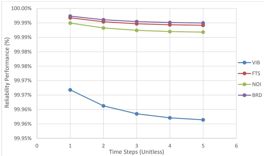
Figure G.37 Reliability performance of oil export pump radial bearing
