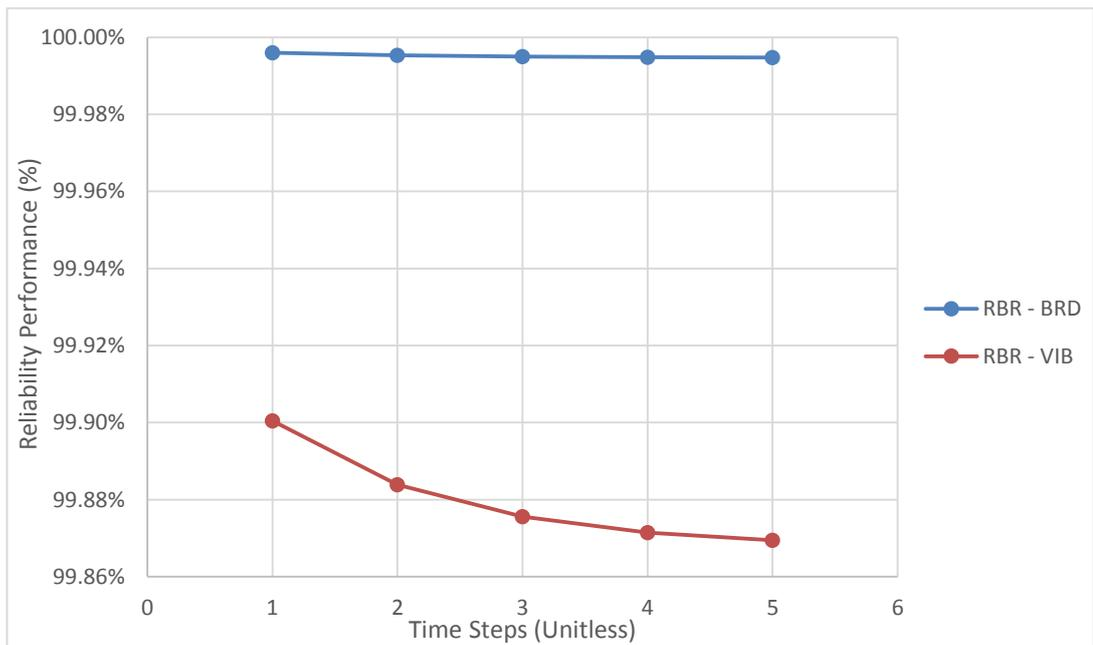
Figure G.59 Reliability performance of crude oil handling pump radial and thrust bearing (RBR and THB)
