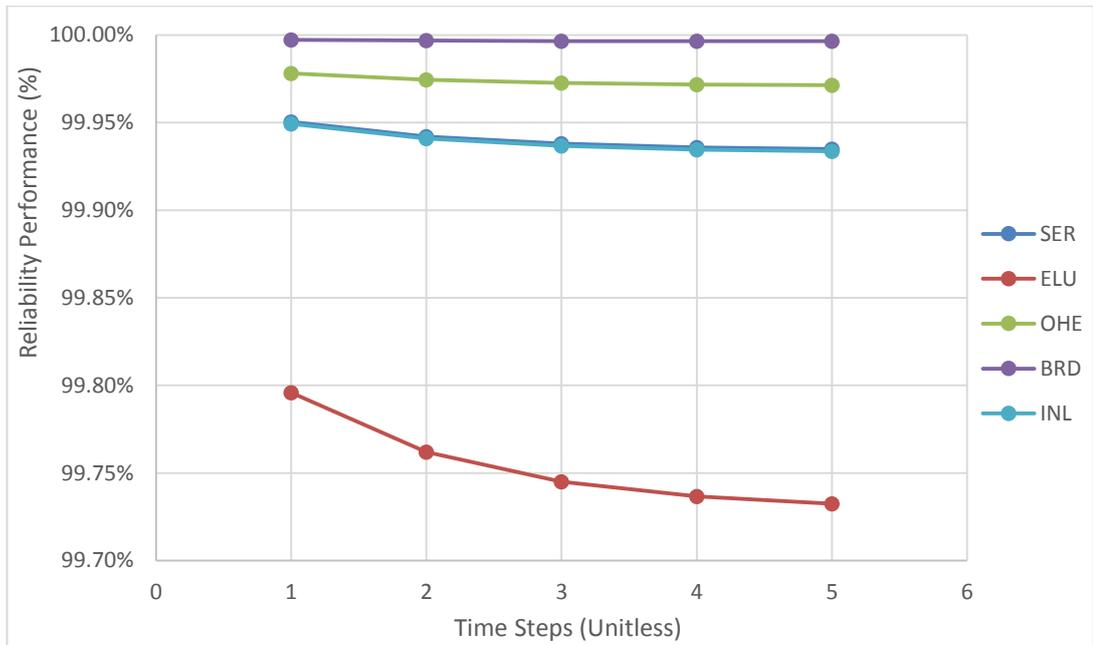
Figure G.56 Reliability performance of crude oil handling pump seals
