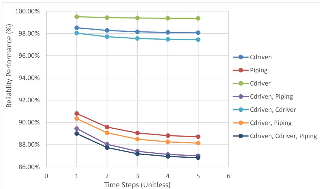
Figure G.23 Reliability performance of seawater lift pump couplers subsystem
