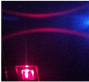
Off resonance fan-shape ASE emission from CQDs emitting at 630nm of CHDV DFB cavity.
