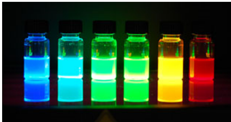
FIGURE 1.6: CQDs in solution with increasing diameter from left to right from Cytodiagnosics http://www.cytodiagnosics.com .
