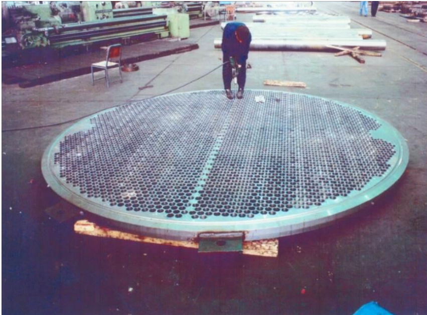
Fig (2.3): Perforated tubesheet
