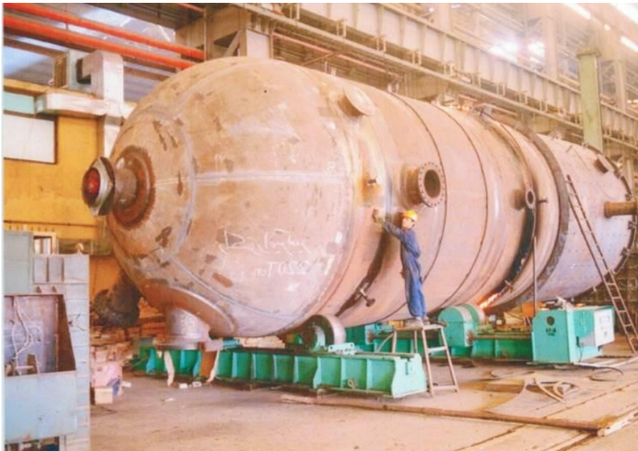
Fig ( 2.1): Reactor during assembly.
