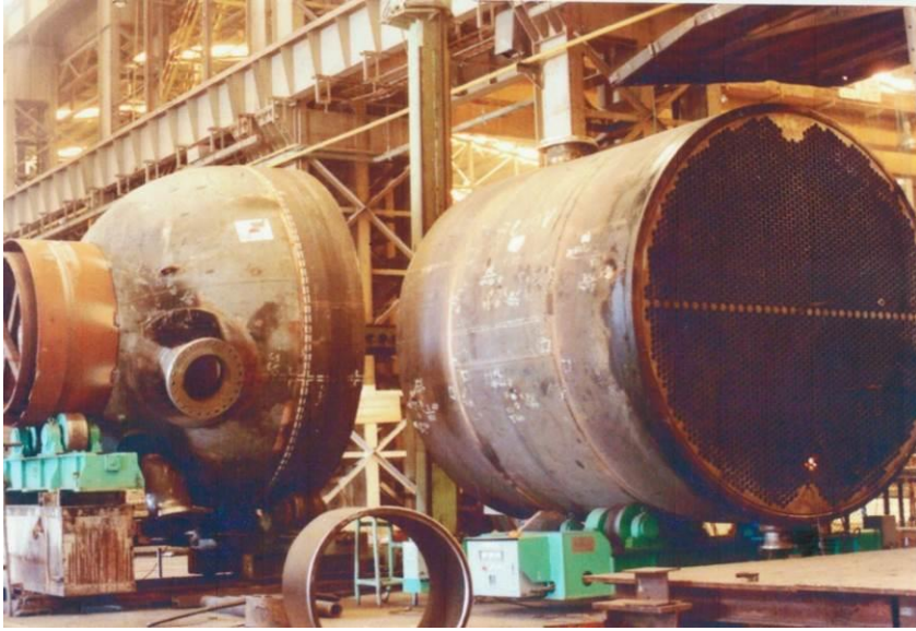
Fig (2.2): Assembled tubesheet.
